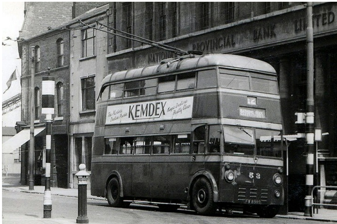
Cleethorpes No. 53 (FW8989), a 1937 AEC 661T with Park Royal 56-seat bodywork. It was withdrawn in 1951. (LTHL collection).
