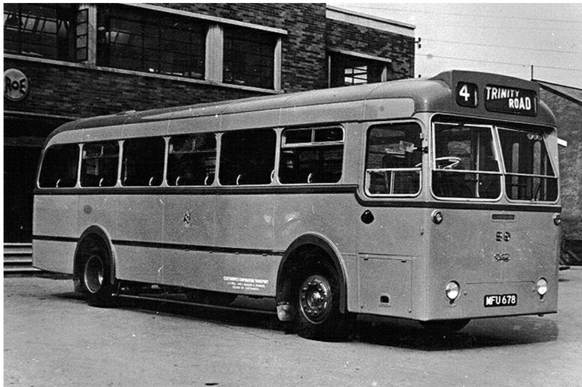
Cleethorpes' final purchase before the merger with Grimsby was No. 29 (MFU678) a Daimler D650HS with Roe 43-seat bodywork, seen here at the bodybuilders works before delivery. (LTHL collection).
