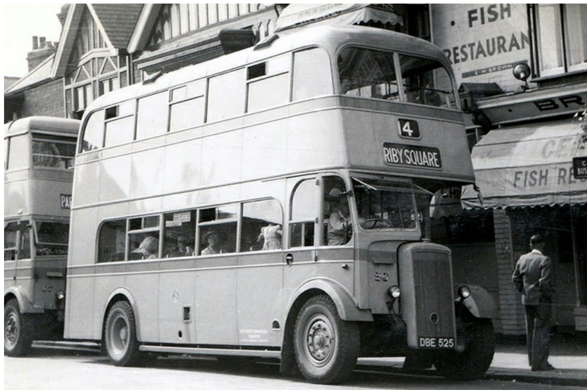
En route for Riby Square is Cleethorpes No. 20 (DBE525), a Willowbrook-bodied Daimler CWD6 dating from 1946 and sporting the later livery of grey with light blue bands and roof introduced in 1950. (LTHL collection).
