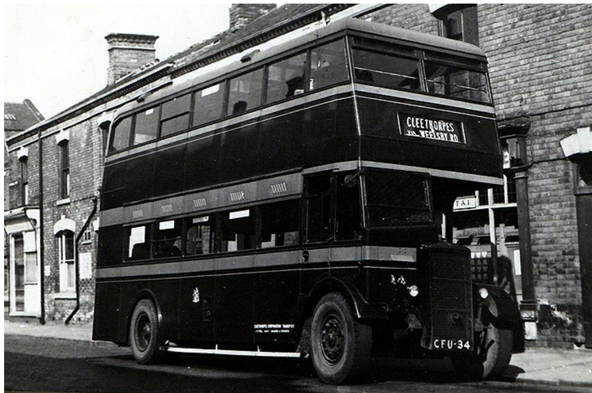
Cleethorpes No. 14 (CFU34) was a 1944 Daimler CWA6 with Brush 55-seat bodywork. Seen here in the dark blue livery with light blue bands and roof introduced in 1939/40. (LTHL collection).
