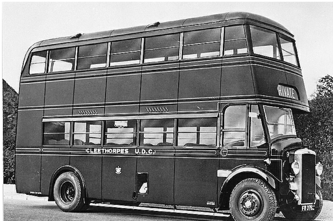
Replacing the former No. 9 in 1933 was FW3762, a Daimler CP6 with Willowbrook 52-seat bodywork. (Bus Archive).
