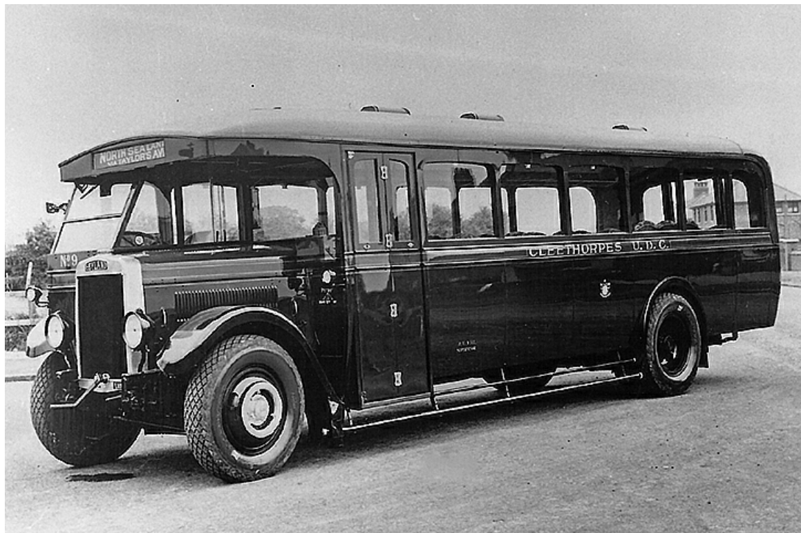
On loan from Leyland Motors during 1932-33 was No. 9 (FW3222) a Leyland LT5 with Leyland 32-seat bodywork. (Bus Archive).
