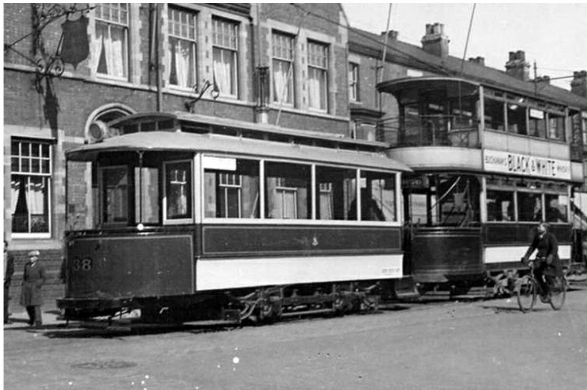
Car 38 was a 1902 ERTCW-built single-decker formerly in the Oldham Corporation fleet. It was painted dark blue and primrose, which was to be the new livery for Cleethorpes' cars but in the event it was the only one so treated. (H.B. Priestley).
