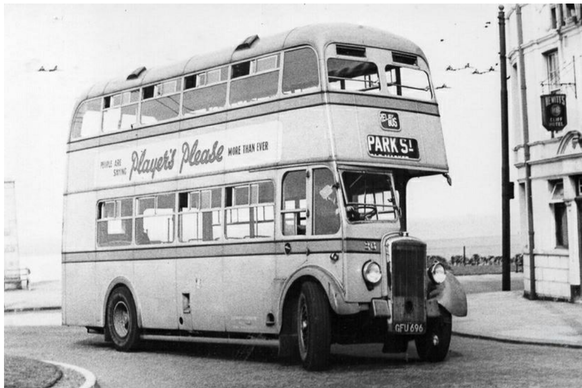
Displaying 'Relief Bus' and heading for Park Street is No. 25 (GFU696) a Daimler CVD6 with Willowbrook 54-seat bodywork dating from 1950. (LTHL collection).
