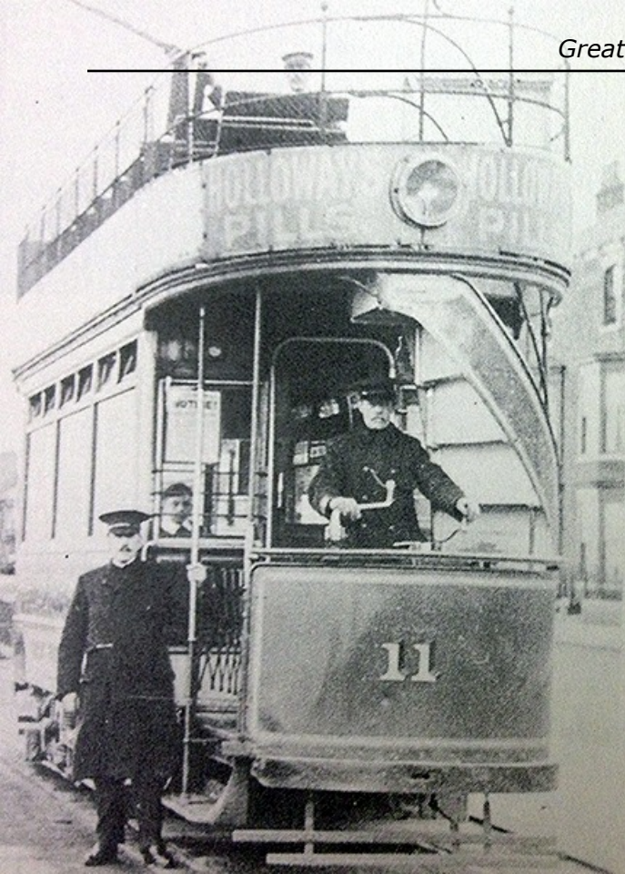
Great Grimsby car No. 11 was formerly car No. 1 built in 1901 by the Electric Railway and Tramway Carriage Works of Preston. It was re-numbered in 1929 and remained open-top throughout its working life. (LTHL collection).
