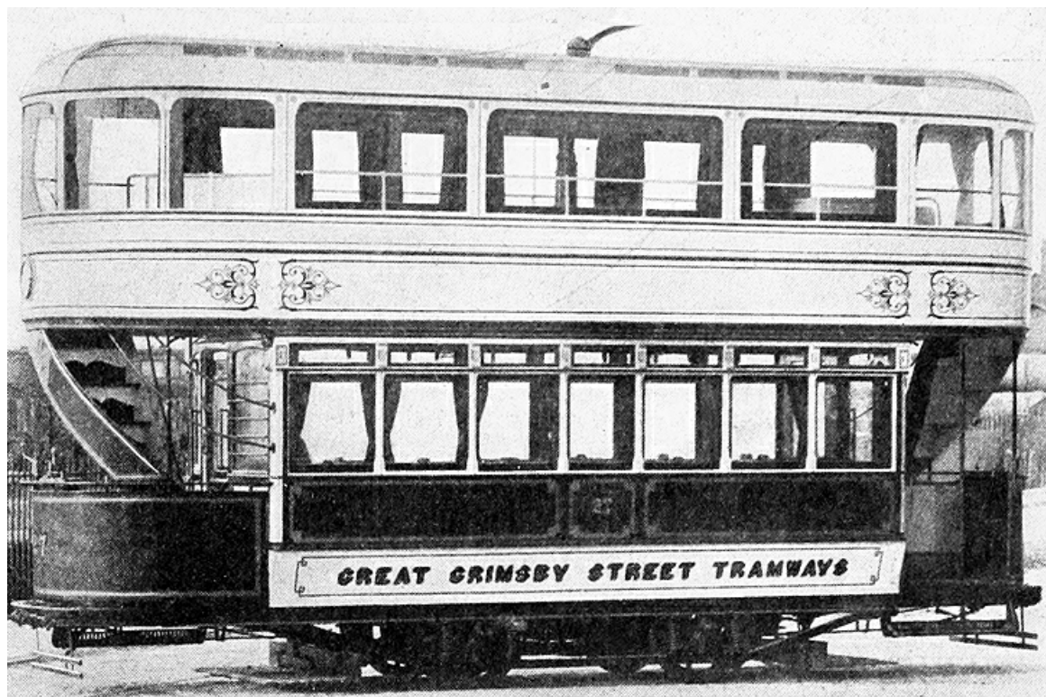
No. 27 was one of four single-deck combination cars acquired from the Alexandra Park Electric Railway and rebuilt by the Company in double-deck form. No. 27 was the only car to be fully-enclosed but was rebuilt with a balcony top cover c. 1910. (LTHL collection).
