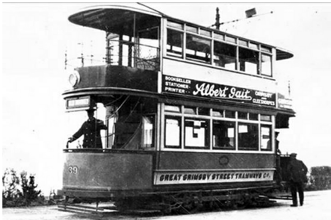
No. 39 was a Company-built car dating from 1925, originally open-top but top-covered in 1926. It passed to Cleethorpes UDC in 1936. (LTHL collection).
