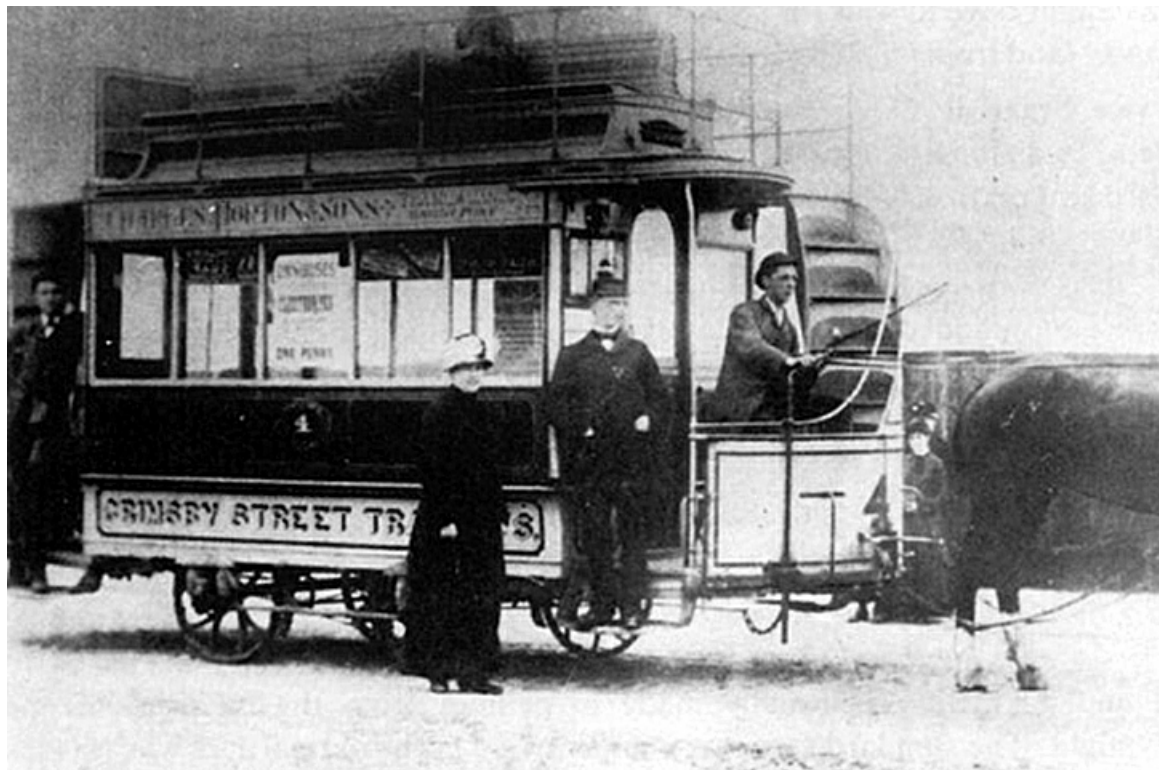
Car No. 4 was one of the original one horse cars built in 1881 for the opening of the system. They were only small vehicles and it was not possible to have the whole company name on the panels, hence the shortened version. (Tramways & Light Railway Society).
