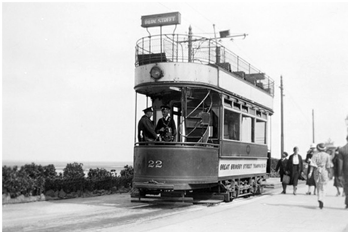
No. 22 was one of a number of trams drafted in from Provincial's Gosport & Fareham fleet in 1929. It was a 1906 Brush-built open-topper seating 55. (M J O'Connor/National Tramway Museum).
