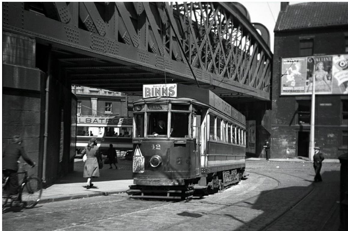
No. 12 was a 1901 single-deck combination bogie car built by the Electric Tramway and Railway Carriage Works of Preston and seating 42. (G. S. Hearse).
