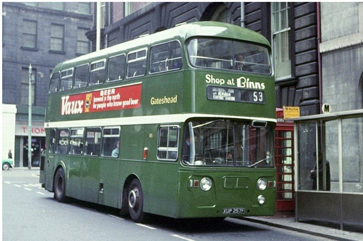
No. 145 (XUP257F) was a 1968 Alexander-bodied Leyland PDR1/1 that was transferred from Northern General in 1970. It was thought that the dual-door bodywork might help speed up loading on the high capacity Gateshead services. (David Taylor).
