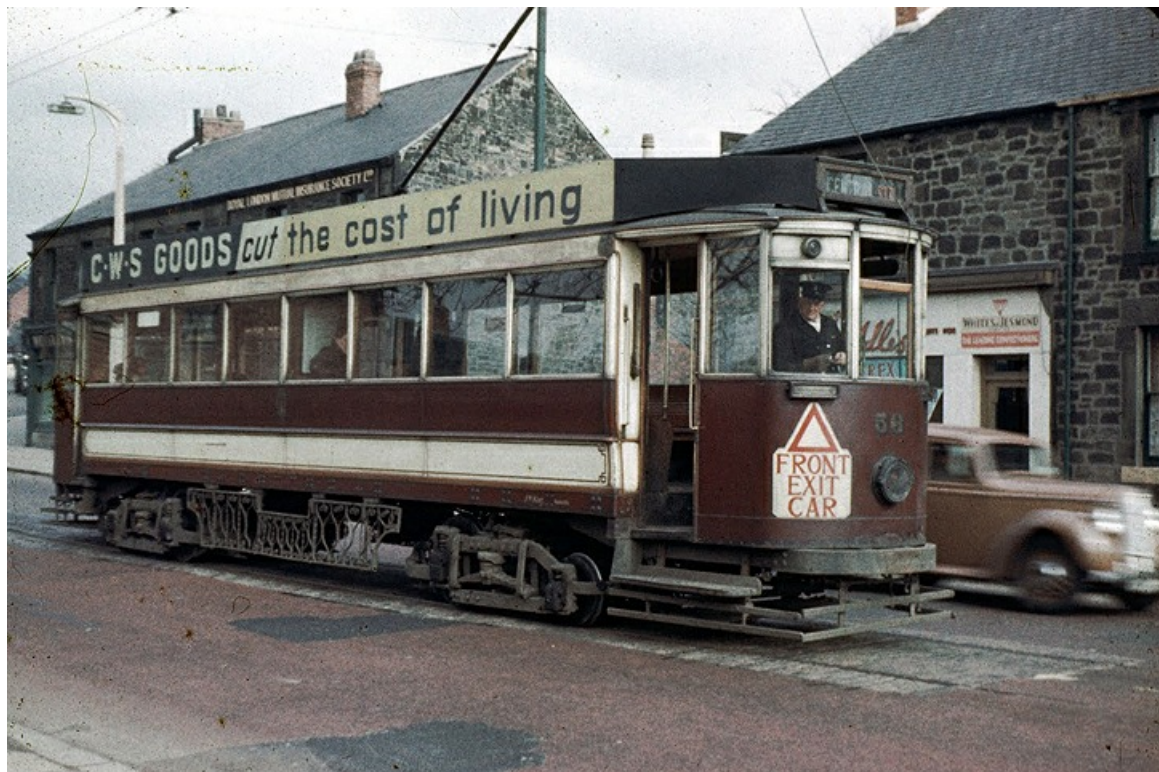
No. 56 was one of five Brush-built single-deck bogie cars built in 1921 and seated 48. (LTHL collection).
