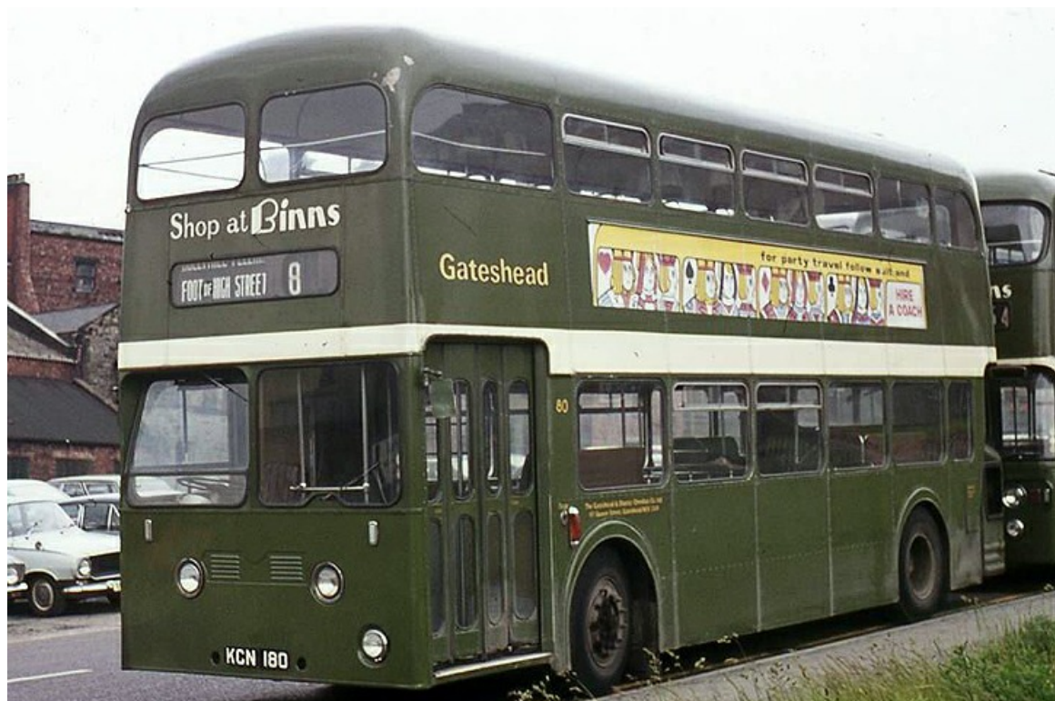
No. 80 (KCN180) was numerically the first Leyland PDR1/1 'Atlantean' in the Gateshead fleet. It carried Alexander 78-seat bodywork and is seen here in Gateshead in June 1972. (Donald Hudson).
