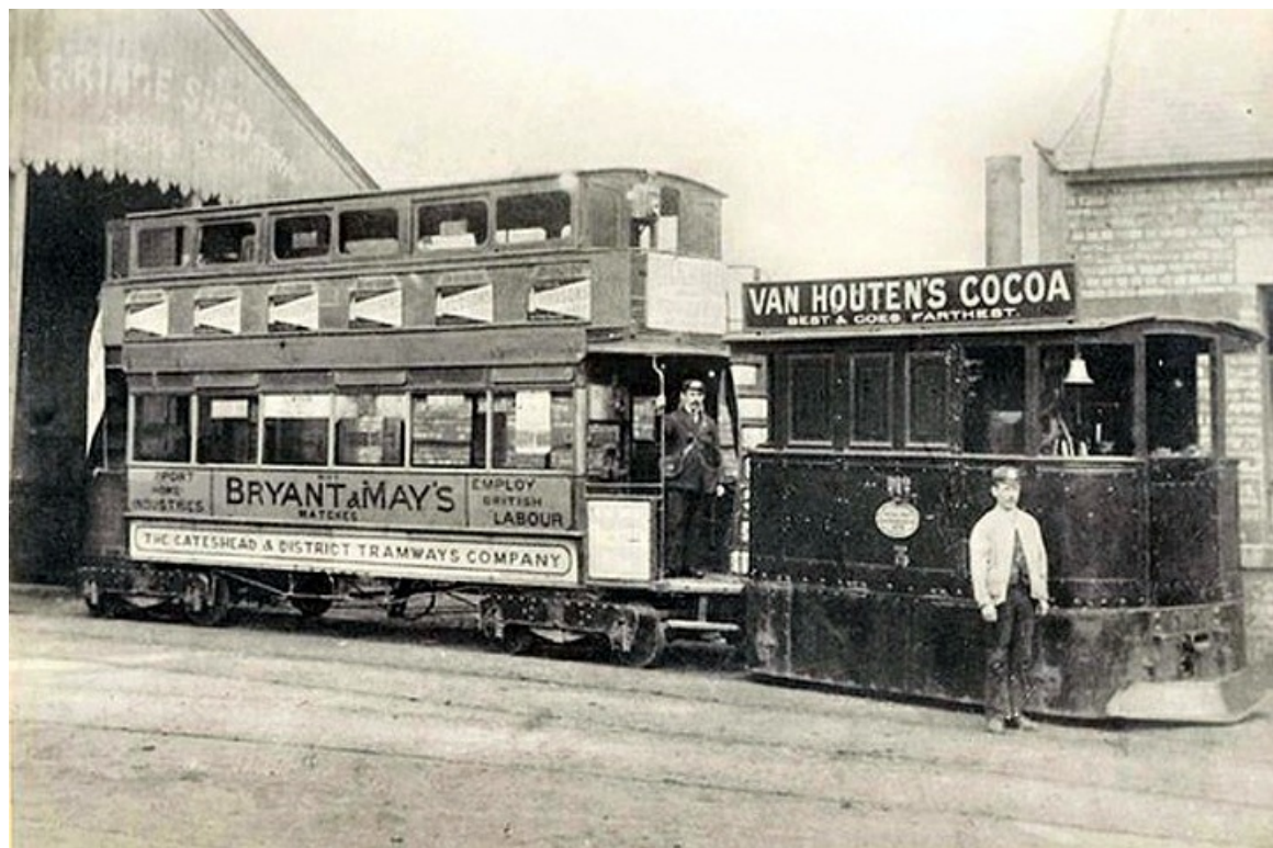
Loco No. 3, built in 1883 by local builders Black, Hawthorn and an unidentified trailer car (possibly one of the two (15-16) built by the Lancaster Carriage & Wagon Company?) c. 1895 outside the depot in Sunderland Road. (LTHL collection).
