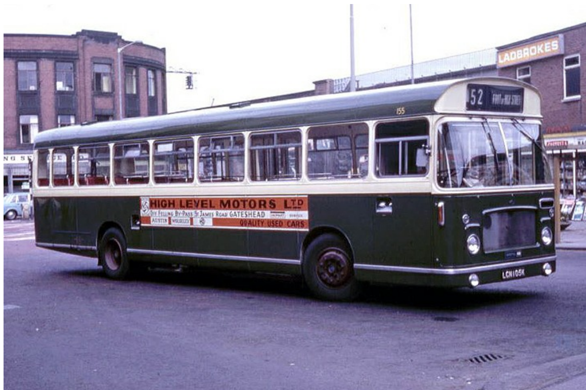
No. 155 (LCN105K) was a 1971 Bristol RELL6G with ECW 44-seat dual entrance bodywork. It did not remain at Gateshead long, being transferred to Northern General in 1972. (George Cropper courtesy Donald Hudson).
