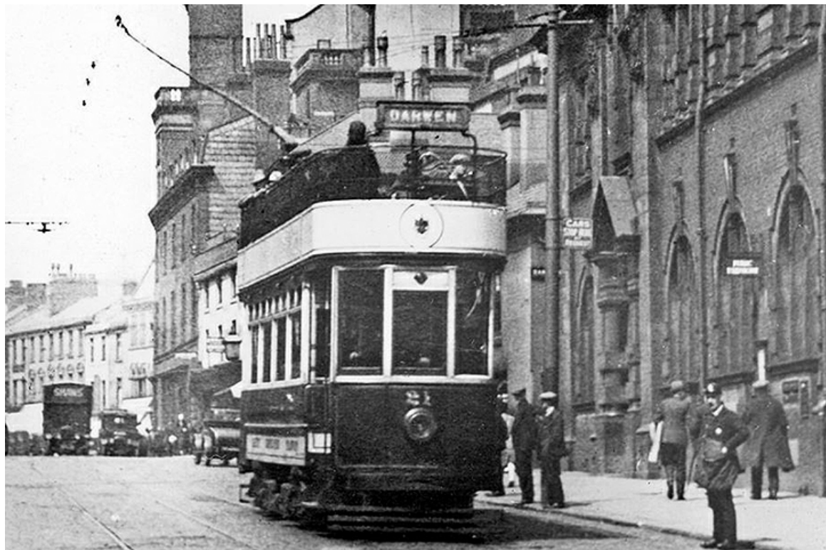
No. 21 was a 1921 English Electric-built double-deck car on English Electric Burnley bogies seating 66. (LTHL collection).
