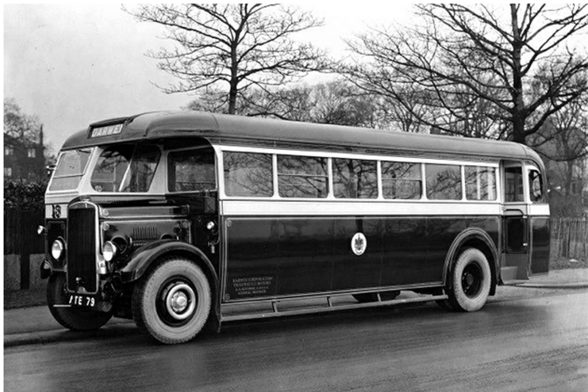
1936 Leyland LT7 No. 13 (ATE79) with English Electric 32-seat bodywork. (GEC collection courtesy David Beilby).
