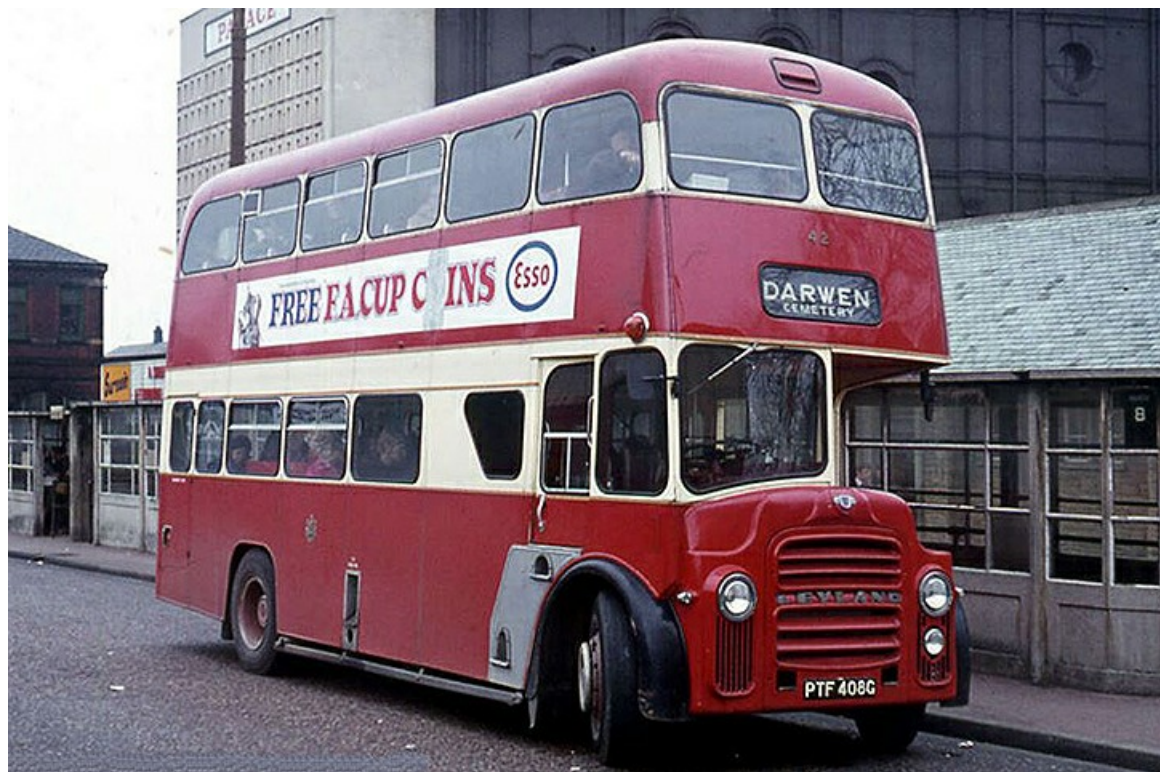
Standing in Blackburn Bus Station in April 1972 is No. 42 (PTF408G), a 1969 Leyland PD2/47 with East Lincs 65-seat bodywork. (John Kaye).
