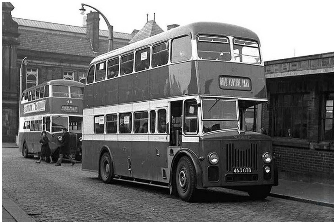
No. 26 (463GTD) was a 1958 East Lancs-bodied Leyland PD2/10 at Darwen Circus in March 1960. (John Kaye).
