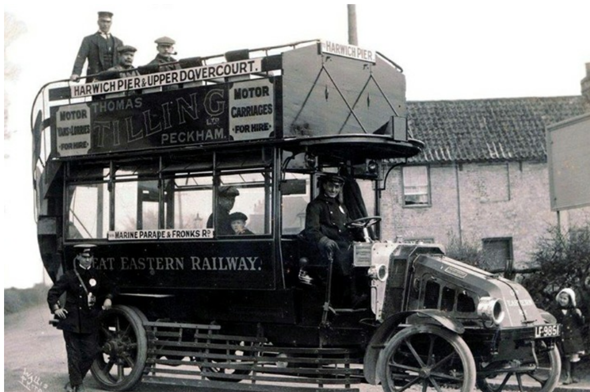
A Tilling Stevens TTA1 petrol-electric bus first introduced on 11th June 1911 and became the standard bus used by Tilling in London and other provincial areas. This is LF9851 on contract to the Great Eastern Railway during 1914. (LTHL collection).
