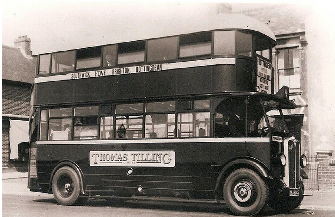
No. 6005 (GJ2005), a Tilling AEC Regent with Tilling open-staircase bodywork operating in Brighton in the early 1930's. It passed to the Brighton, Hove & District company when it was formed in 1935 and later converted to open top. (LTHL collection).
