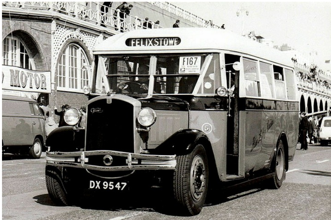
In 1930 Gilford introduced the AS6 with a seating capacity of around 20. This is a preserved AS6 of Blue Safety Coaches with Eaton 20-seat bodywork. (LTHL collection).
