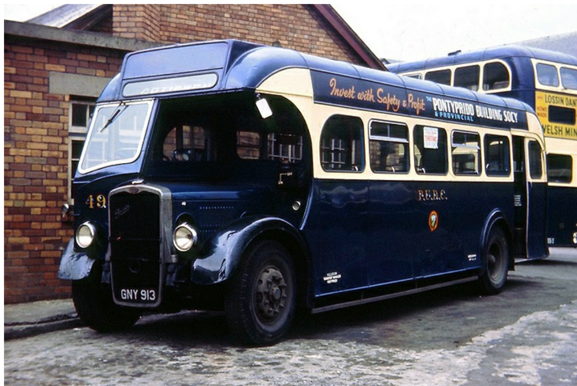
No. 49 (GNV213) was one of four Bristol L5G's with Beadle B32R bodywork purchased in 1947. (John Huddleston).
