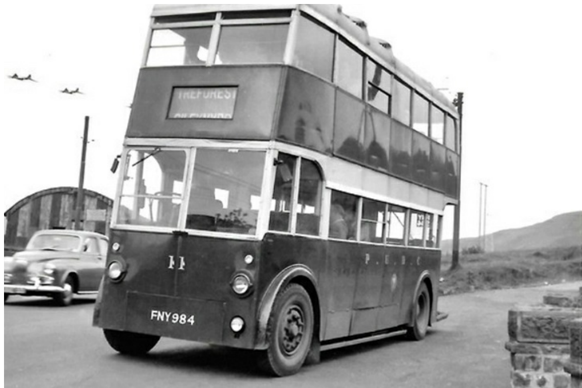
No. 11 (FNY984) was a 1945 Karrier W with Weymann 56-seat bodywork. It remained in service until the end of the system in 1957. (LTHL collection).
