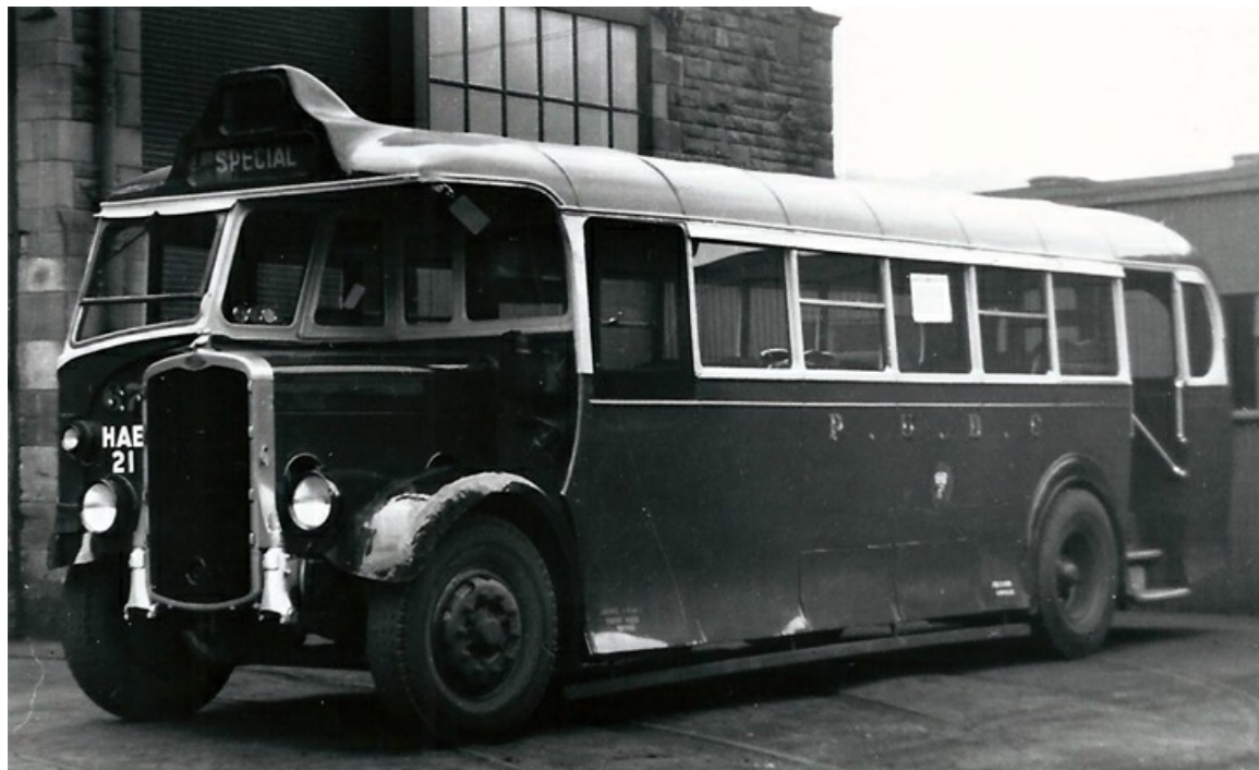
In 1952 Pontypridd acquired three 1941 Bristol L5G's with Bristol B32D bodywork from the Bristol Tramways & Carriage Company. This is No. 67 (HAE21). The forward entrance was not used in service and this particular vehicle had the entrance panelled over whilst the other two had their entrance doors locked. (LTHL collection).
