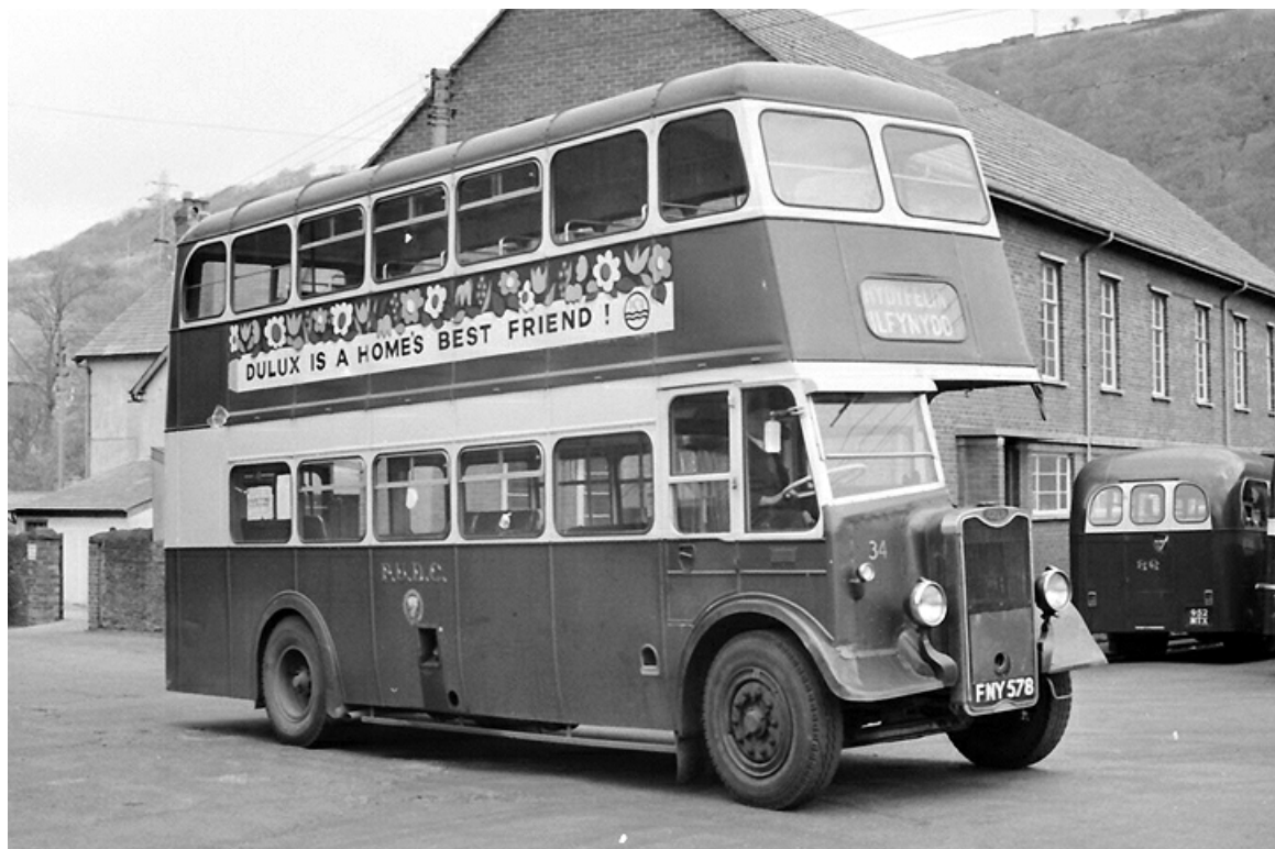
No. 34 (FNY578) was a Guy Arab II with Park Royal H30/26R bodywork dating from 1944. (Stuart Johnson).
