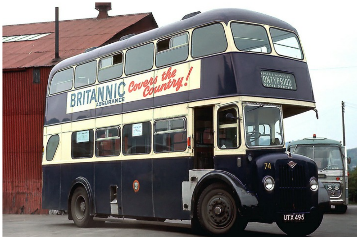
Seen at Glyntaff garage and sporting a plain fleet number is 1957 Guy Arab IV No. 74 (UTX495) with Roe H33/25R bodywork. It was withdrawn in July 1973. (Alan Snatt).
