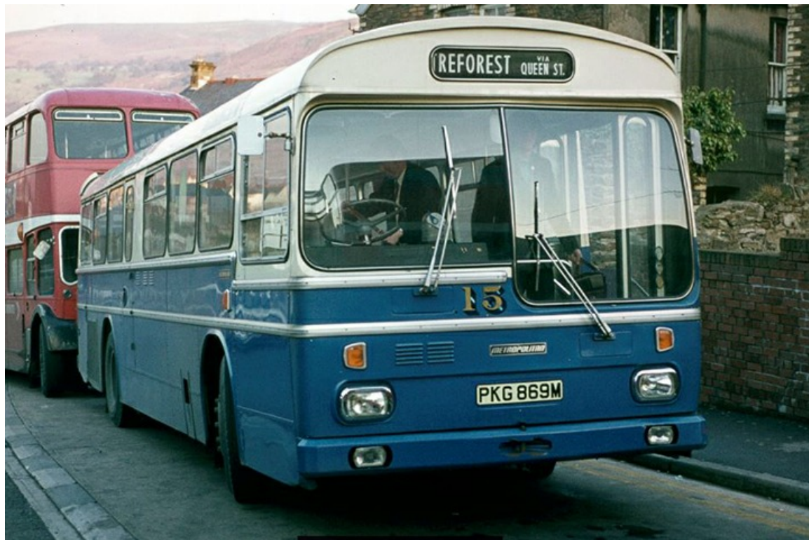
No. 15 (PKG869M), a 1974 Metro-Scania BR11MH with Metro-Cammel 44-seat bodywork. It passed to Taff-Ely Borough Council later that year. (Richard Simons).
