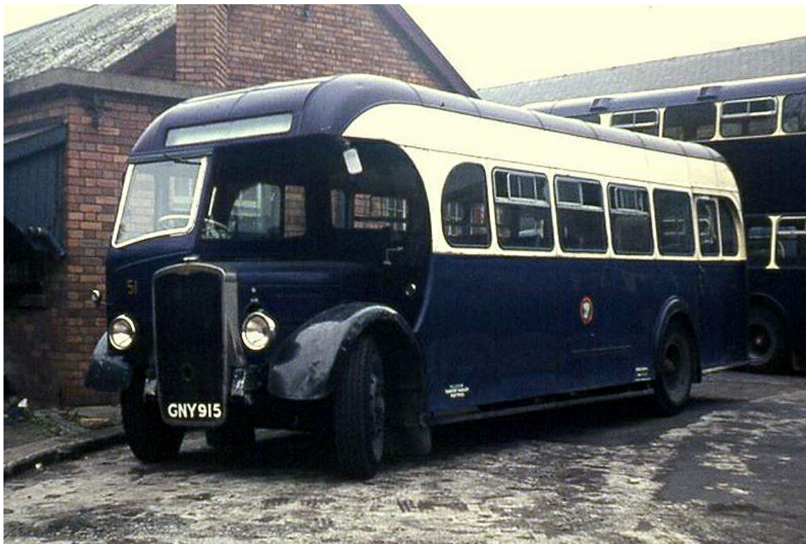
No. 51 (GNY915), a 1947 Bristol L6G with Beadle 32-seat bodywork. It was used as the towing vehicle from 1967 and put back in service for a short while in 1972 before finally being withdrawn in 1973. (John Kaye).
