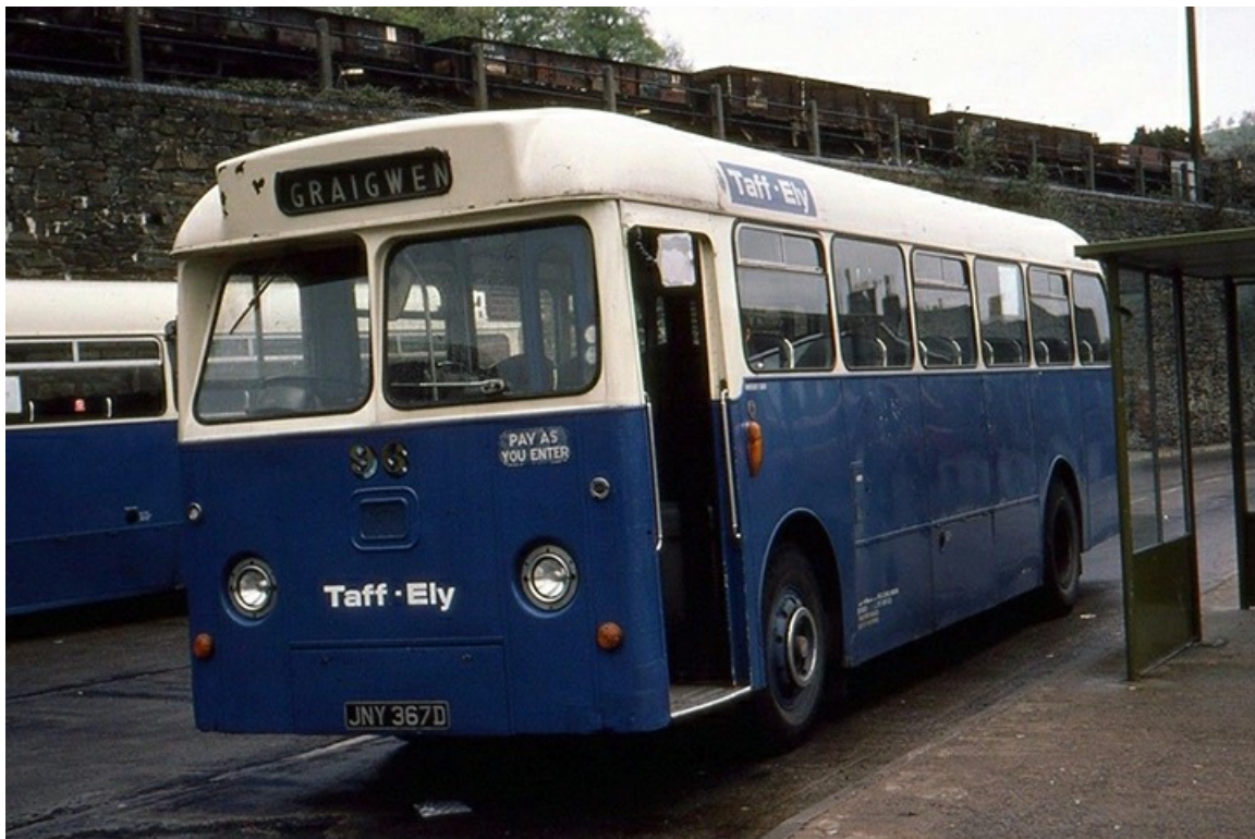
No. 96 (JNY367D), dating from 1966 was an AEC Reliance with Willowbrook 45-seat bodywork, seen here after Pontypridd became Taff-Ely District Council in 1974. (LTHL collection).
