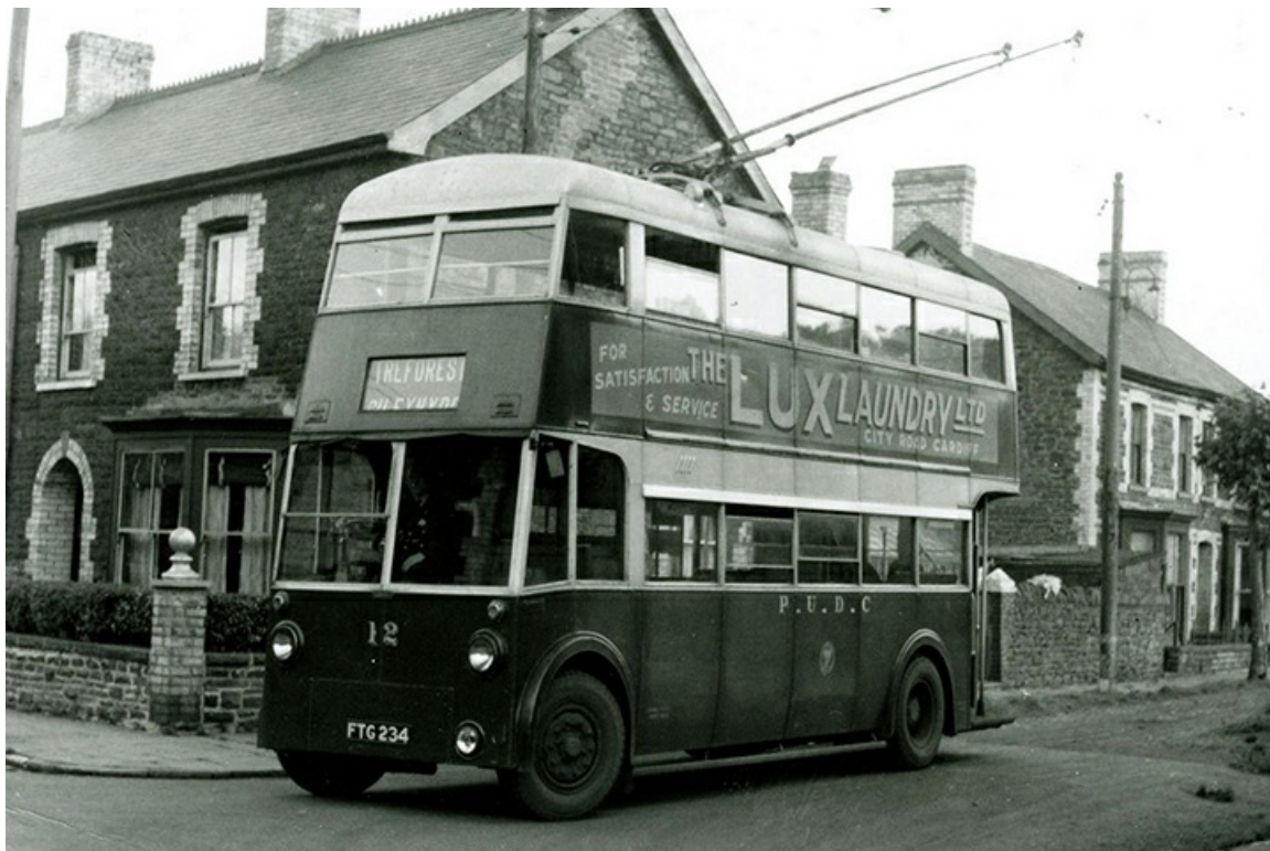
No. 12 (FTG234), dating from 1945, was also a Karrier W but with Park Royal 56-seat bodywork that also survived until the end of the system in 1957. (LTHL collection).
