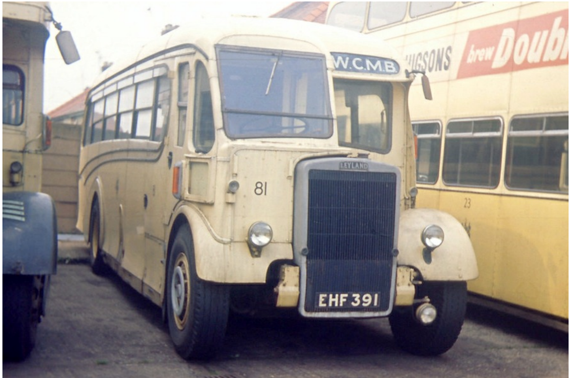
No. 81 (EHF391), originally No. 7, was a 1957 Leyland PD2/10 was fitted with the 1947 Burlingham body from No. 24 (also originally No. 7) of 1936. It was withdrawn in 1966. (John Huddlestone).
