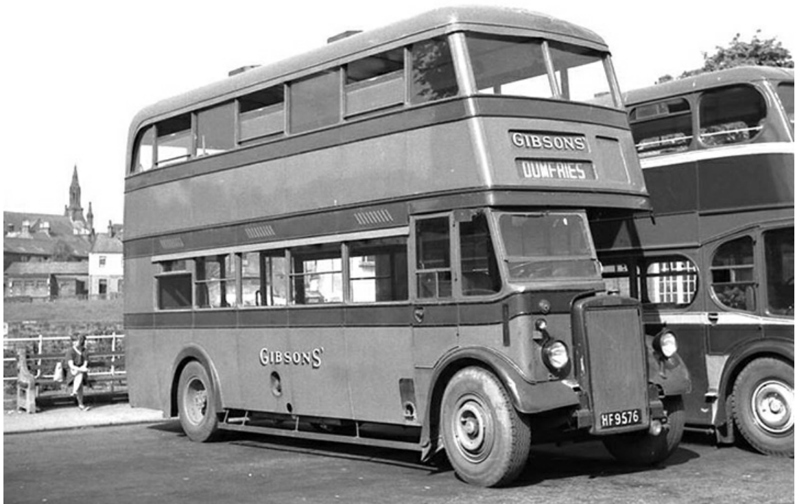
HF9576, a 1946 Leyland PD1 with MCCW 56-seat bodywork seen here in service in Dumfries with Gibsons, was formerly Wallasey Corporation No. 79 that had been withdrawn in 1958. (John Boylett courtesy John Kaye).
