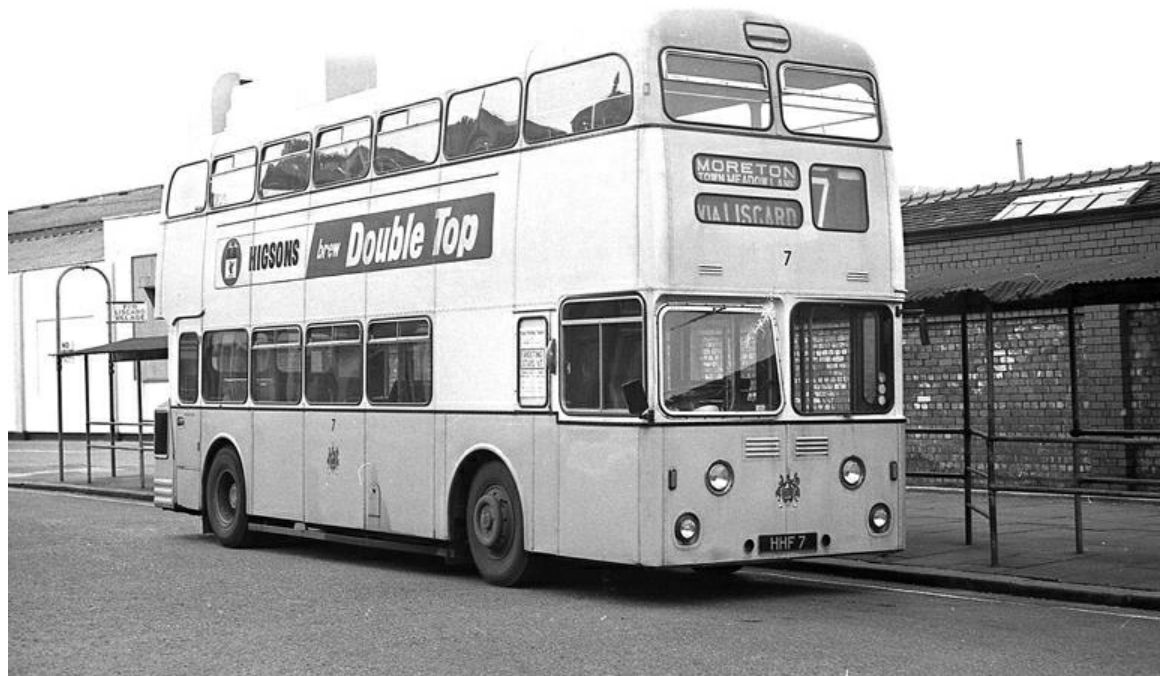
No. 7 (HHF7), was a 1960 Leyland PDR1/1 'Atlantean' with MCCW 77-seat bodywork. It passed to Merseyside PTE in 1969. (Mike Beamish).
