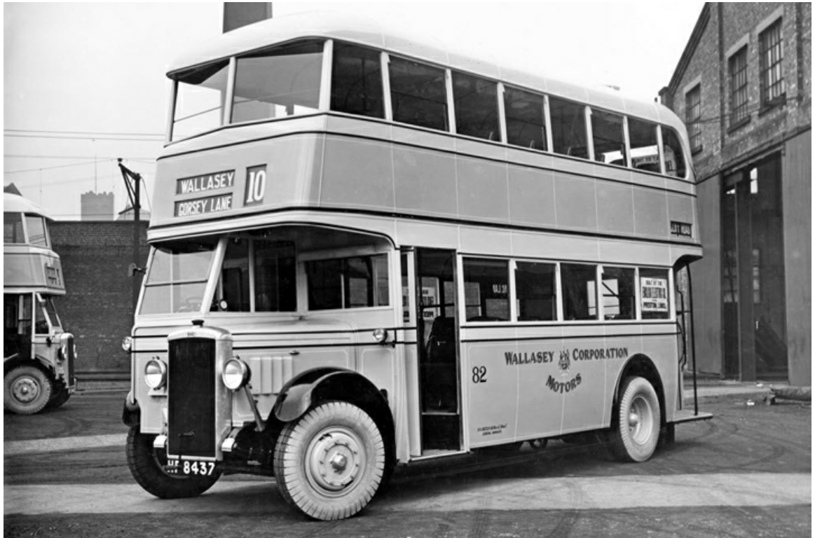
HF8437 was a 1933 Daimler CP6 with English Electric dual entrance 48-seat bodywork. Numbered 82, it was withdrawn in 1941. (GEC collection courtesy David Beilby).
