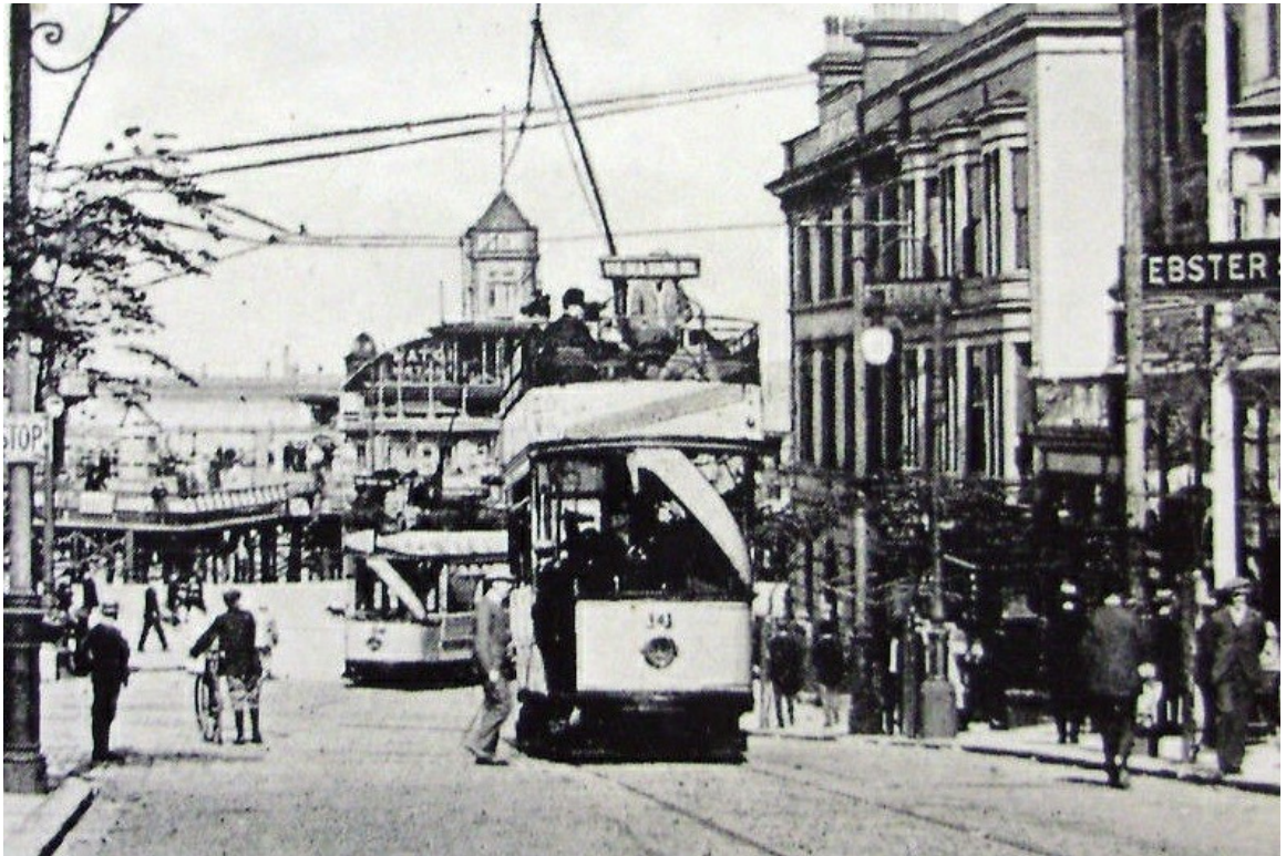
Wallasey No. 14 was a 1902 Electric Railway & Tramway Carriage Works built 4-wheel double-deck car. It is seen here in New Brighton in original form c. 1903 and was top-covered by 1905. (LTHL collection).
