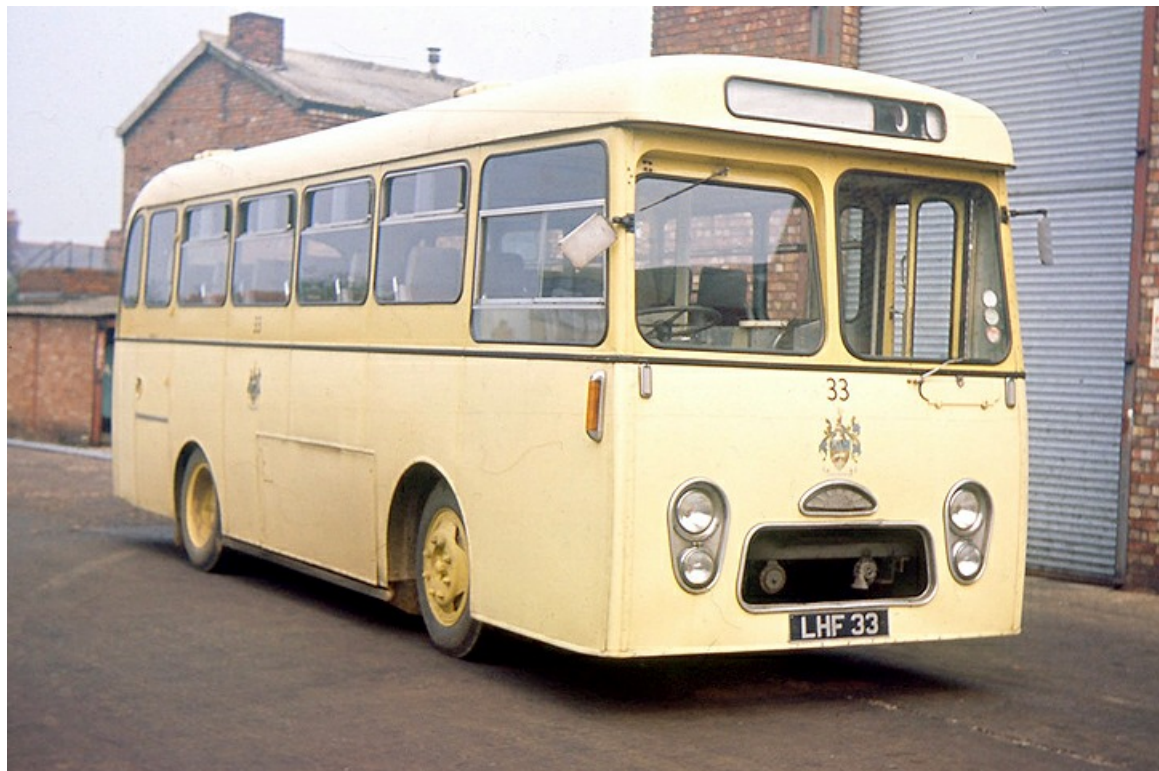
No. 33 (LHF33) was one of 4 of Albion Nimbus chassis with Strachan dual-purpose 31-seat bodywork purchased in 1962. (John Huddleston).
