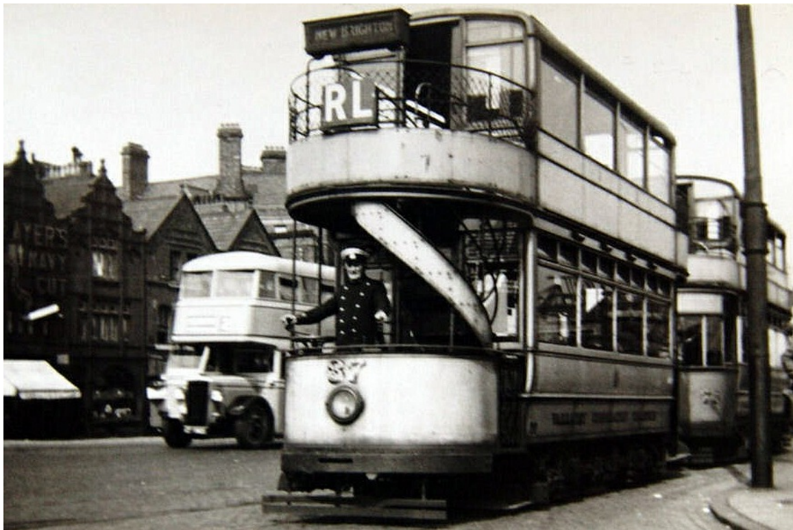
Wallasey car No. 37 was a 1908 United Electric Car-built top-covered double-decker on Mountain & Gibson trucks, seating 62. (LTHL collection).
