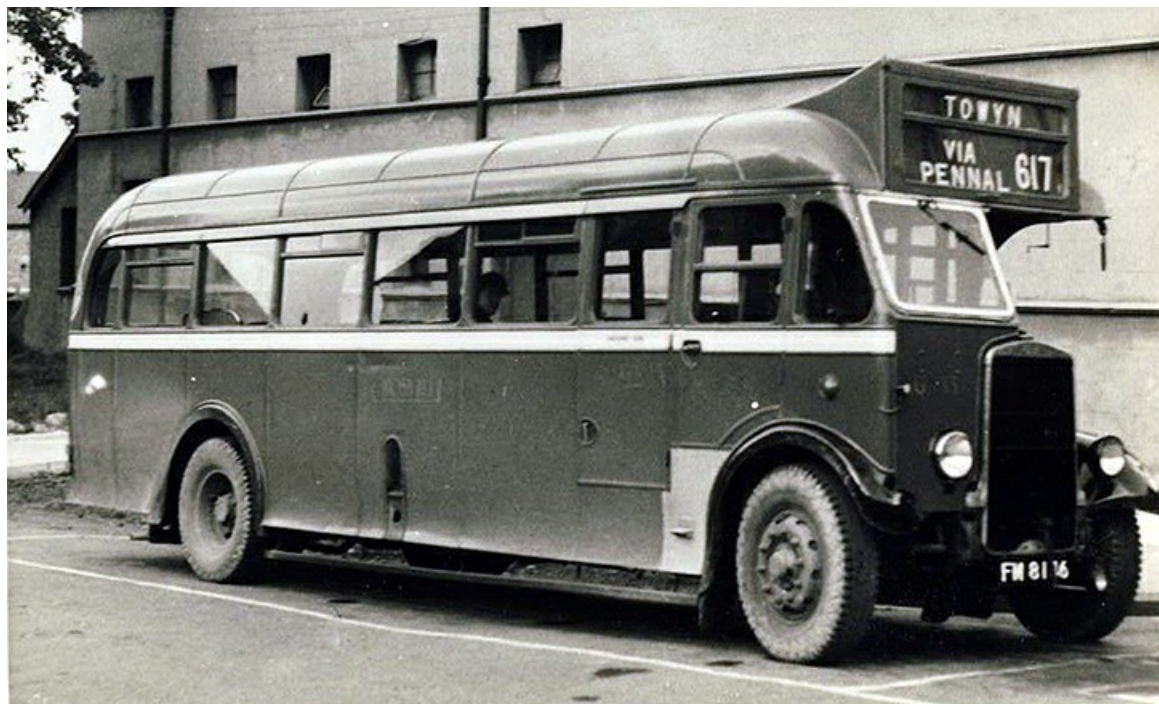
No. 903 (FM8136) was a 1934 Leyland LT5A originally with Eastern Counties B32F bodywork. It was re-numbered G5 in 1935 then fitted with an oil engine in 1949, re-bodied by Burlingham to B35F and re-numbered GA5 as seen here. (LTHL collection).
