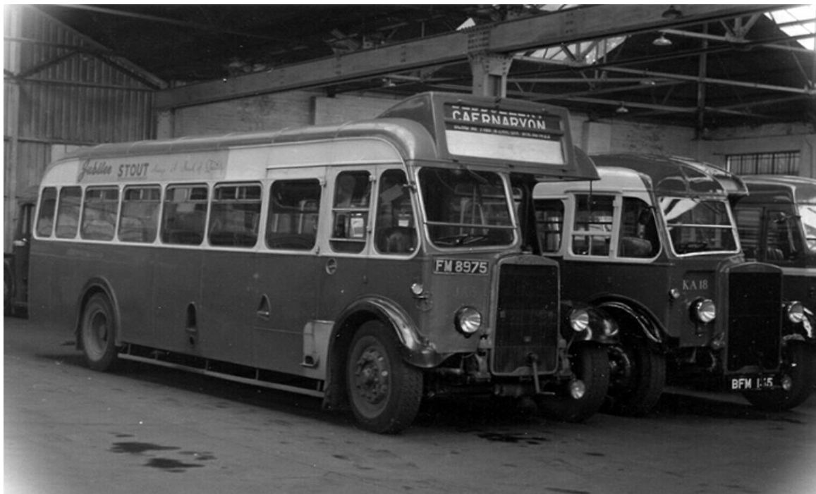
Crosville JA5 (FM8975) was originally J5 but was re-bodied by ECW, fitted with an oil engine and re-classified JA in 1949. It was a 1935 Leyland LT7 and survived until 1960 in this form. (Dennis Kerrison via Ron Hughes).
