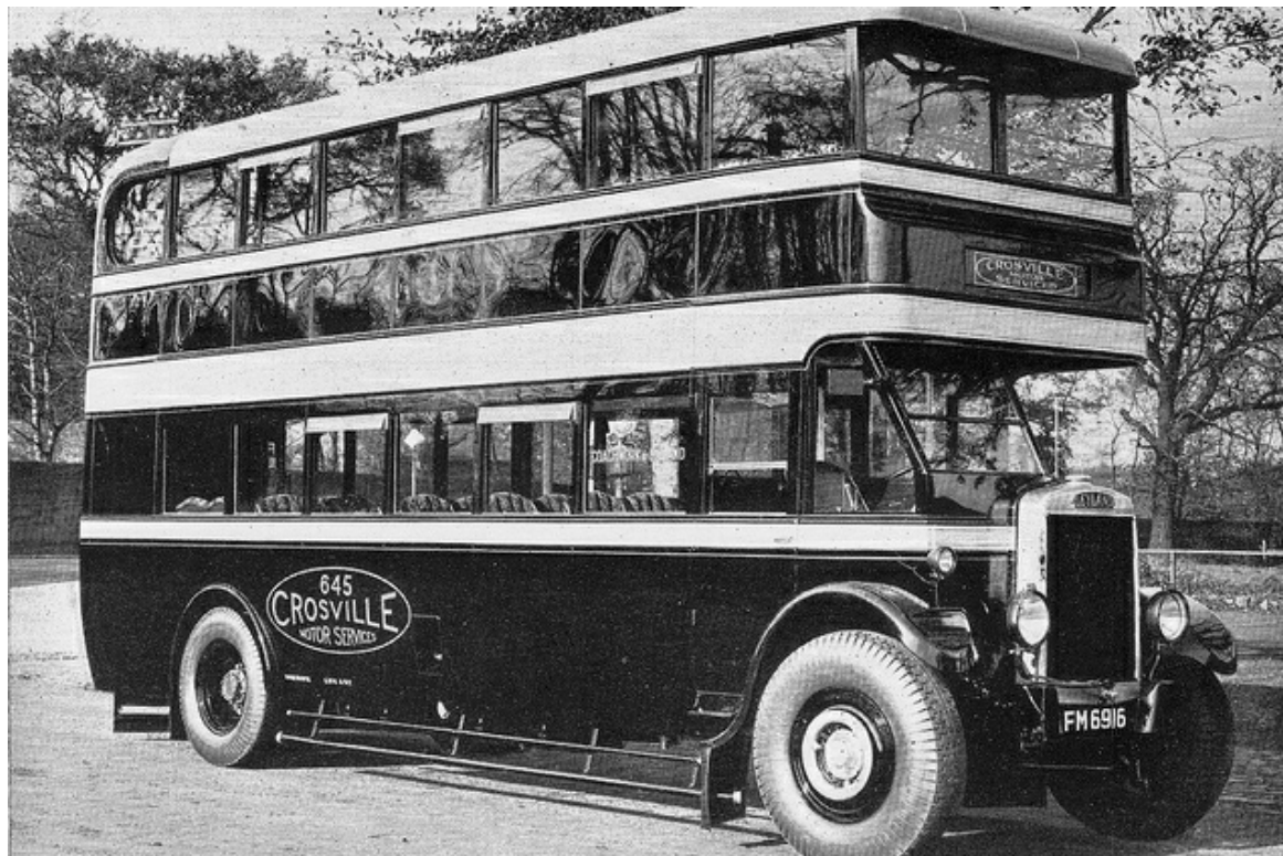
No. 645 (FM6916) was a 1931 Leyland TD2 with Leyland 51-seat body. It was fitted with an oil engine and re-numbered M22 postwar and withdrawn in 1954. (LTHL collection).
