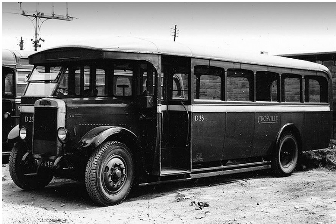
D25 (FM6419) was originally No. 440 a 1931 Leyland LT2 with Leyland B35F body. It had been withdrawn by 1952. (Dennis Kerrison via Ron Hughes).
