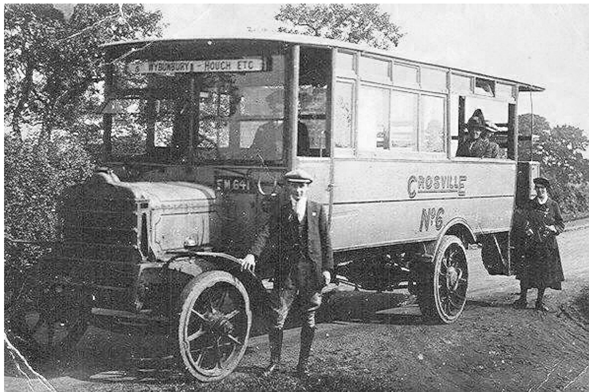
Crosville No. 6 (FM641) was a 1913 Daimler CD with Henry Eaton B32R bodywork. The lady conductress dates this photo to World War I. (LTHL collection).
