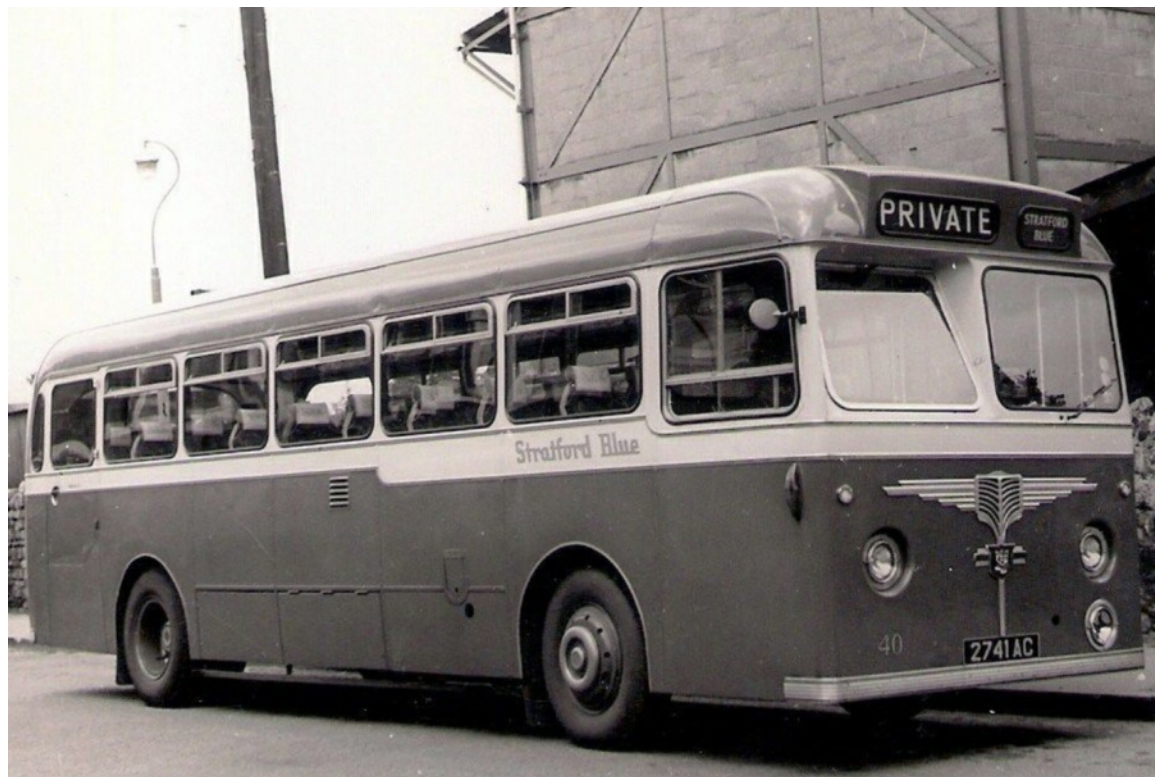
No. 40 (2741AC) was a 1959 Leyland Tiger Cub with Willowbrook 45-seat dual purpose bodywork. (LTHL collection).
