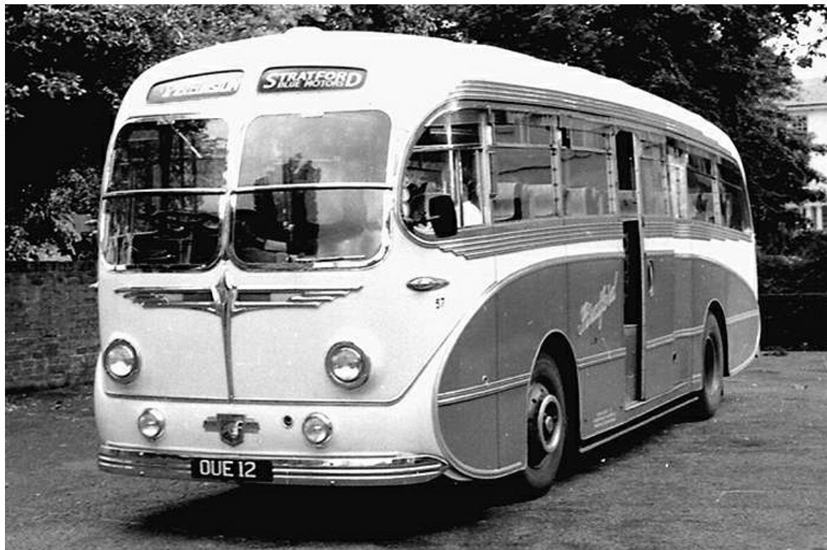
Leyland Tiger No. 57 (OUE12) dated from 1954 and carries a Burlingham 'Seagull' 37-seat body. (LTHL collection).
