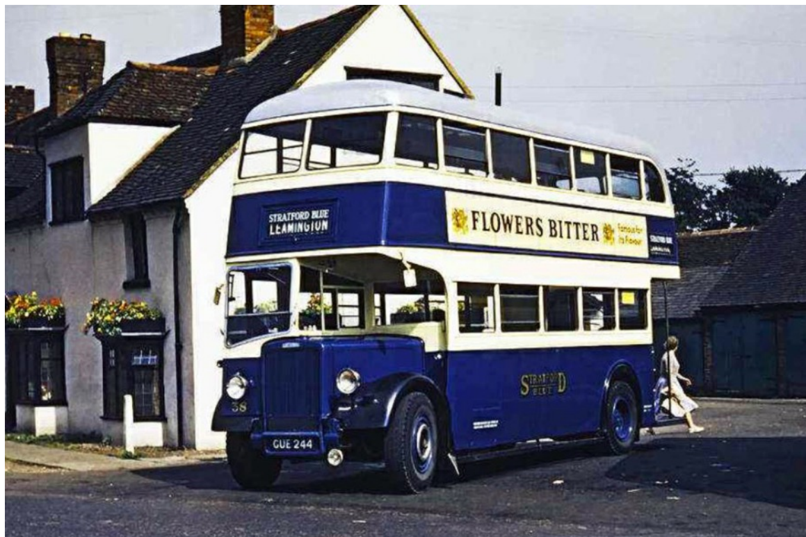
No. 38 (GUE244) was a Leyland PD2/1 with Leyland 56-seat bodywork, one of eight similar vehicles purchased in 1948. (LTHL collection).
