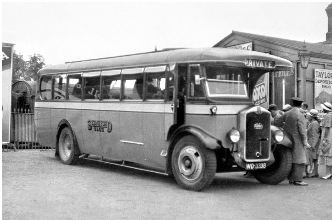
WD3338 was a 1932 Albion PV70 demonstrator with Cowieson 32-seat bodywork, which was on loan for 6 months during 1932 and numbered 23 during its stay. (Bus Archive).
