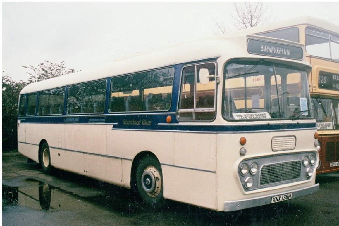
No. 36 (XNX136H) was the last vehicle to be delivered before Stratford Blue were absorbed by Midland Red. It was a Leyland PSU3A/4R 'Leopard' with Alexander 49-seat dual purpose bodywork. (LTHL collection).
