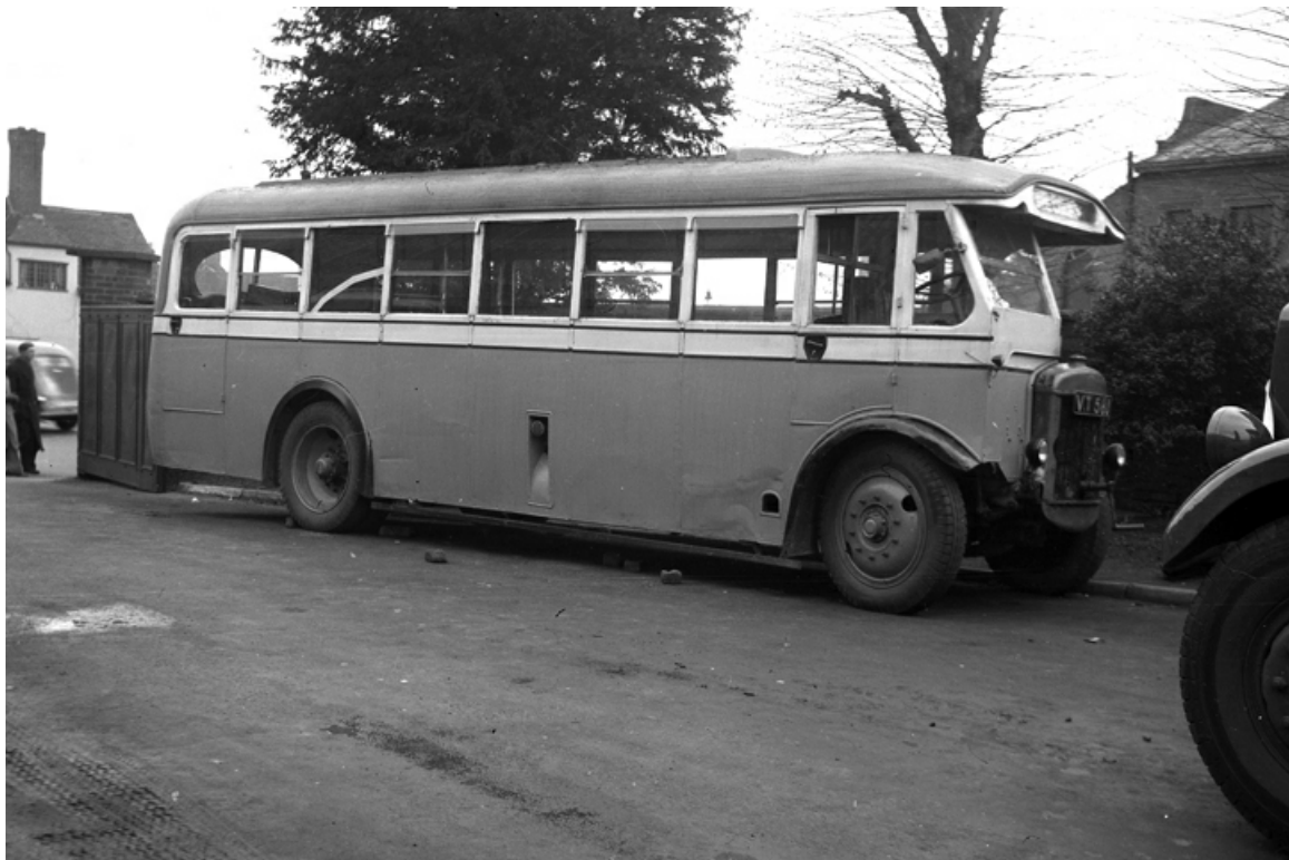
No. 12 (VT580) was acquired from Trent Motor Traction in 1936 and was new in 1927. It was a Tilling-Stevens B10A2 with Willowbrook B32F bodywork. (Bus Archive).
