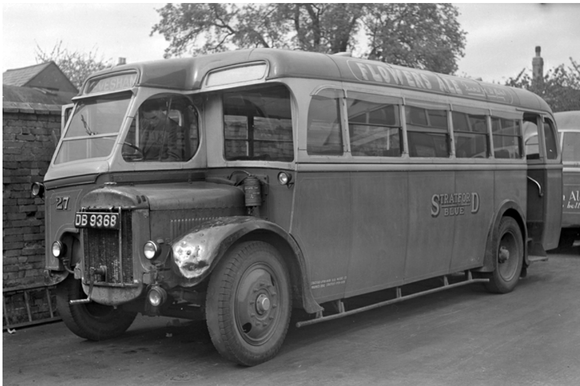
No. 27 (DB9368) was yet another 1930 Tilling-Stevens B10A2 from North Western Road Car this time with an Eastern Counties B31R body. (Bus Archive).
