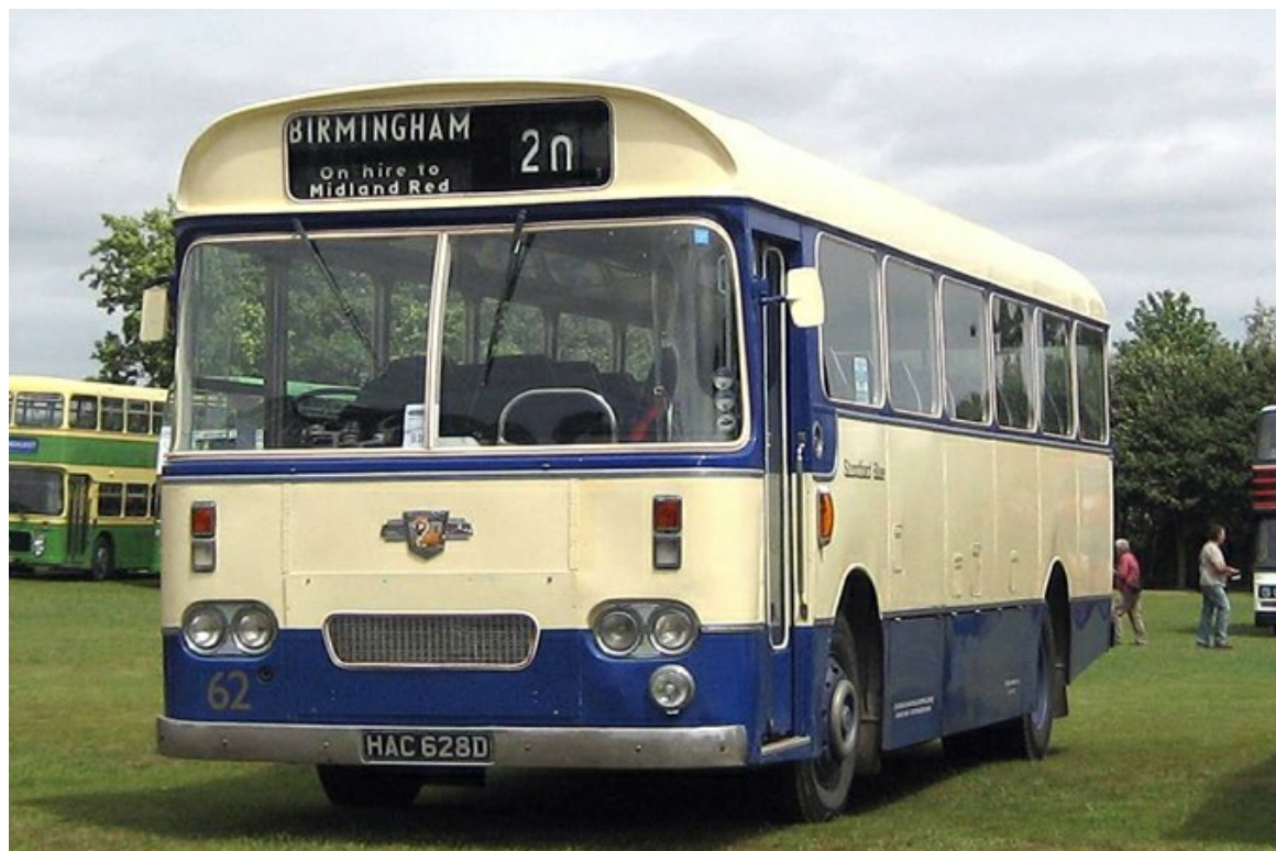
Preserved Stratford Blue No. 62 (HAC628D), a 1966 Leyland Leopard with Marshall dual-purpose 41-seat bodywork. (David Lang).
