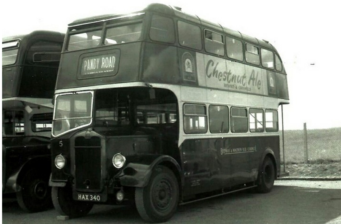
Bedwas & Machen No. 5 (HAX340) was a 1948 Albion CX1 with Welsh Metal Industries 57-seat lowbridge bodywork. It was withdrawn in 1961. (LTHL collection).
