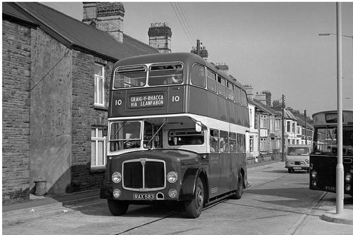
No. 10 (RAX583) was another AEC Regent V with Massey 57-seat bodywork built in 1957, it was withdrawn in 1973. (Dick Dapr ).
