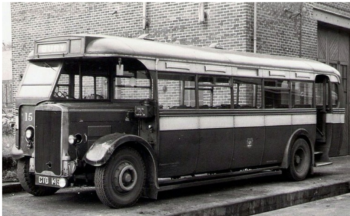
No. 15 (CTD149) was a 1937 Leyland Tiger TS8 with Roe 36-seat bodywork. It spent 21 years in the fleet before being withdrawn in 1958. (LTHL collection).
