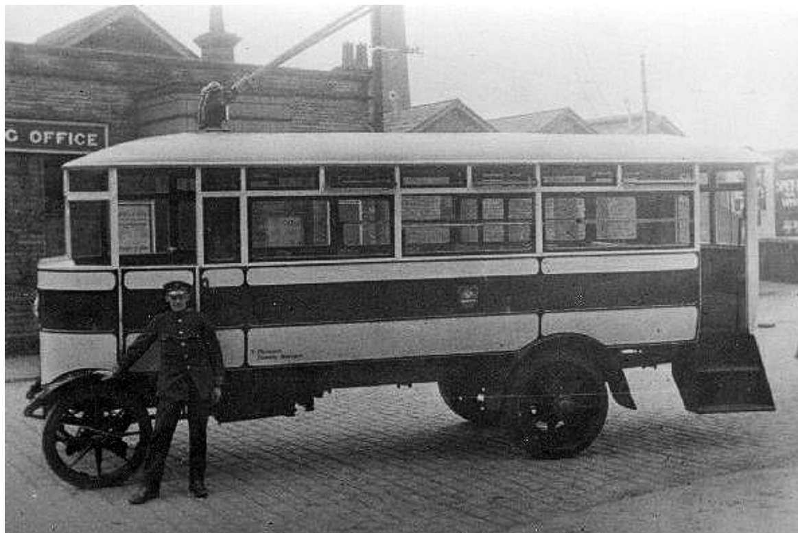
No. 7 was a 1922 Railless M-type built by Thornycroft with Short Bros B26R bodywork. (LTHL collection).
