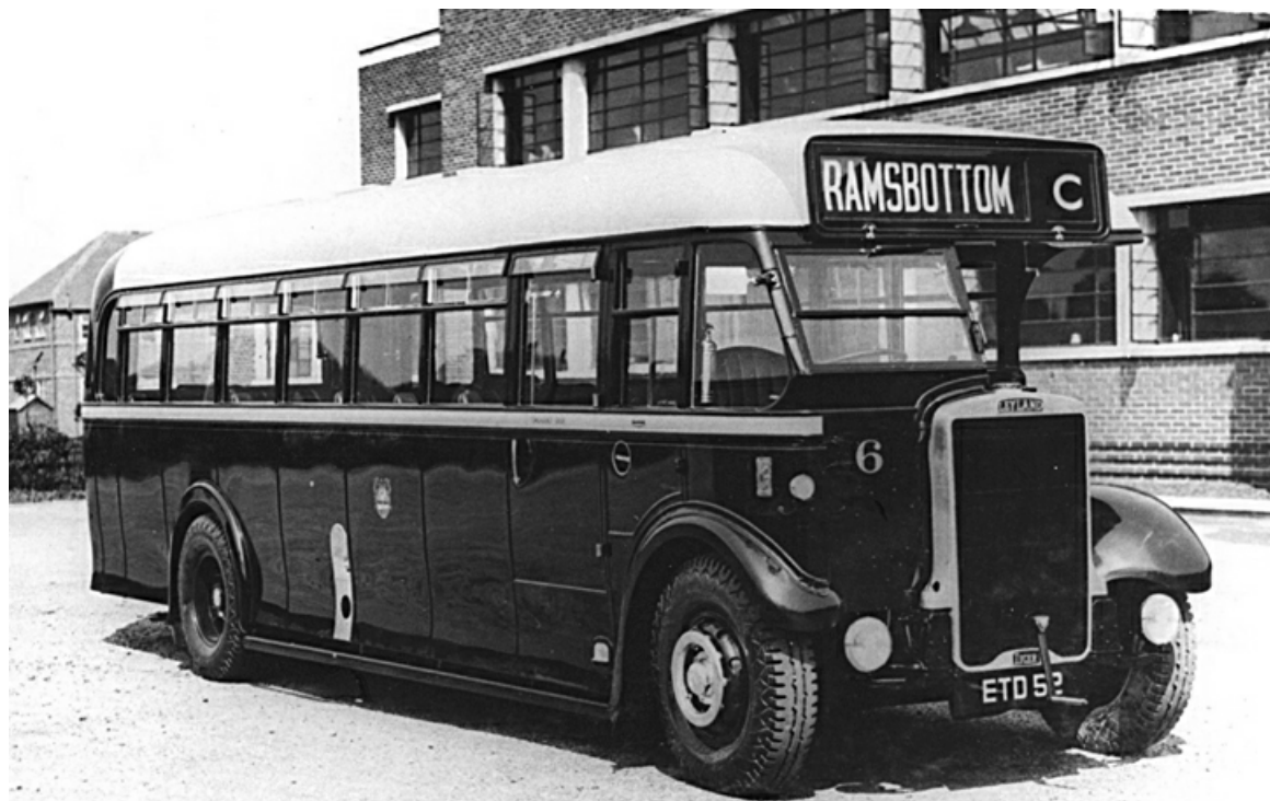
No. 6 (ETD52) was one of two Leyland TS8 'Tigers' with Roe B36R bodywork purchased in 1939. (LTHL collection).
