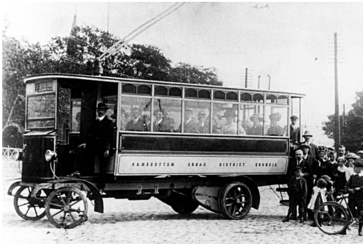
Ramsbottom No. 2 at Edenfield terminus. It was a 1913 Railless trolleybus with Milnes Voss 28-seat bodywork. (LTHL collection).
