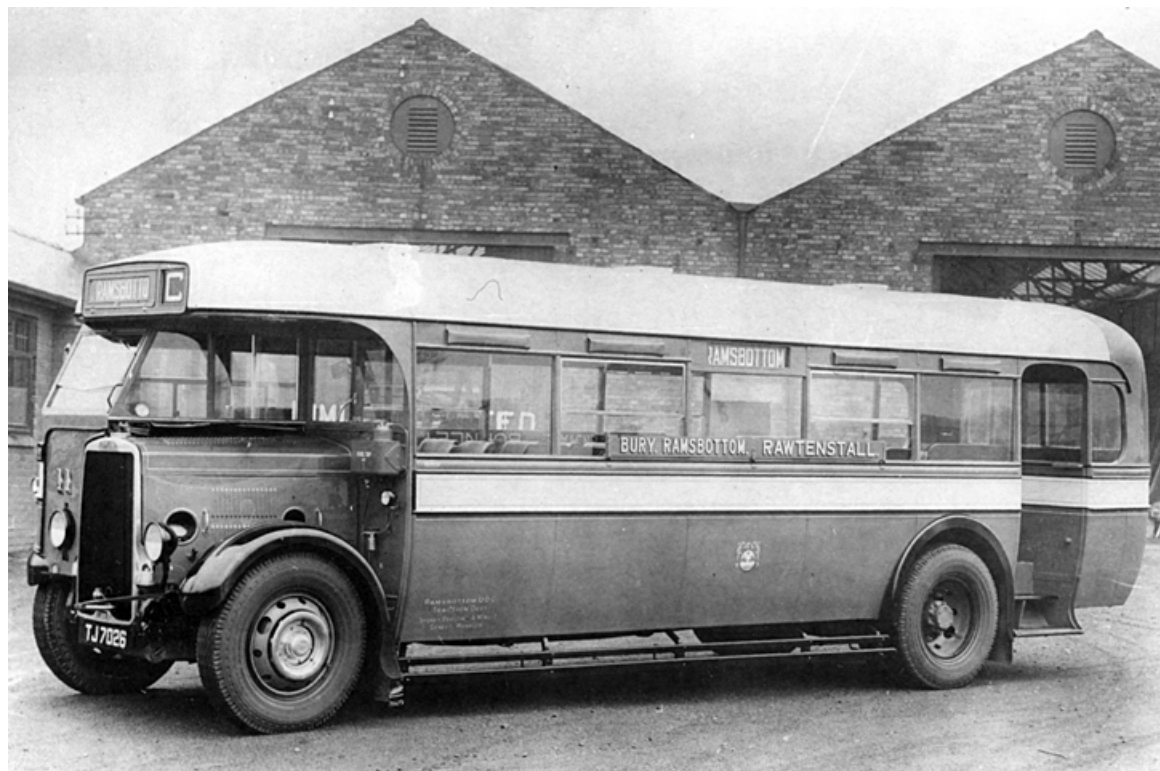
Seen outside the depot is No. 11 (TJ7026) a 1934 Leyland LT5A with Roe B36R bodywork. (LTHL collection).
