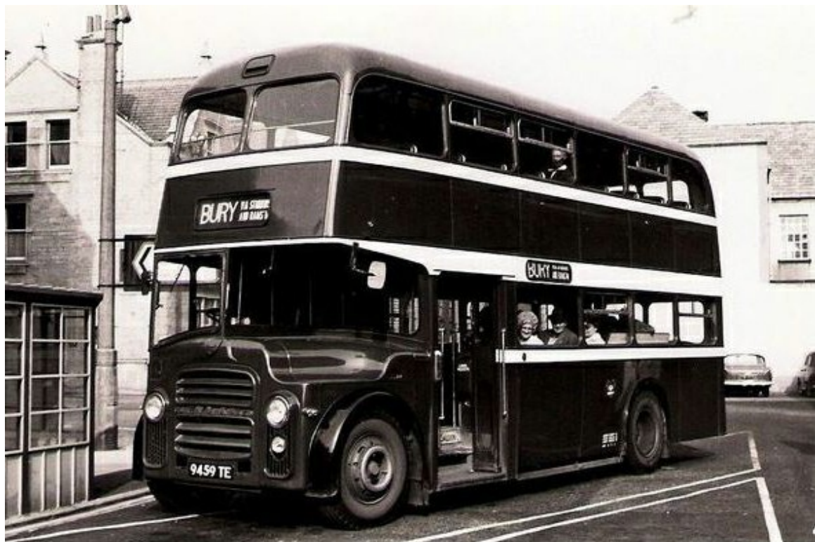
1963 Leyland PD2A/3 No. 3 (9459TE) with East Lancs 63-seat bodywork. This bus passed to SELNEC in 1969 where it became No. 6403. (LTHL collection).
