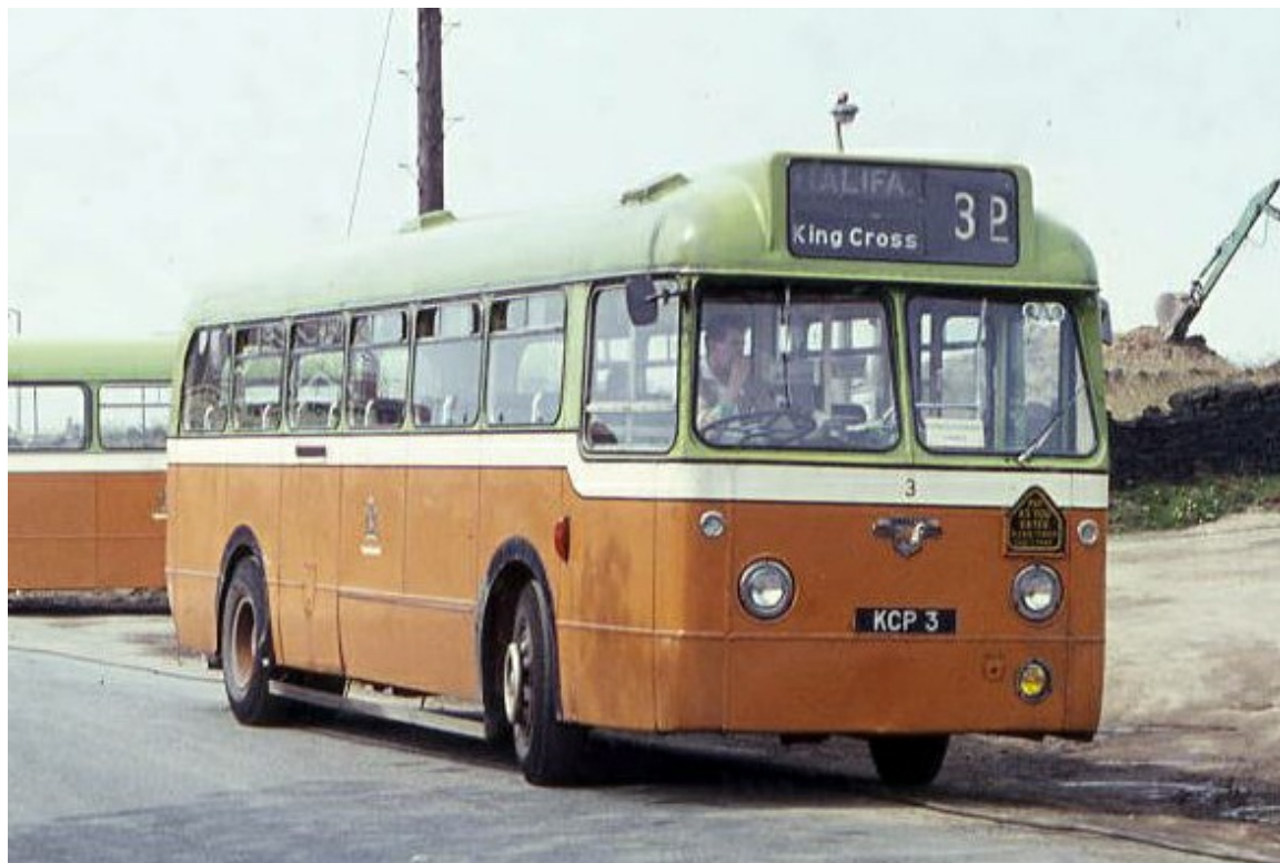
No. 3 (KCP3) was one of nine Leyland Royal Tiger Worldmasters purchased in 1958. All had Weymann 42-seat bodies. (David Mitchell).
