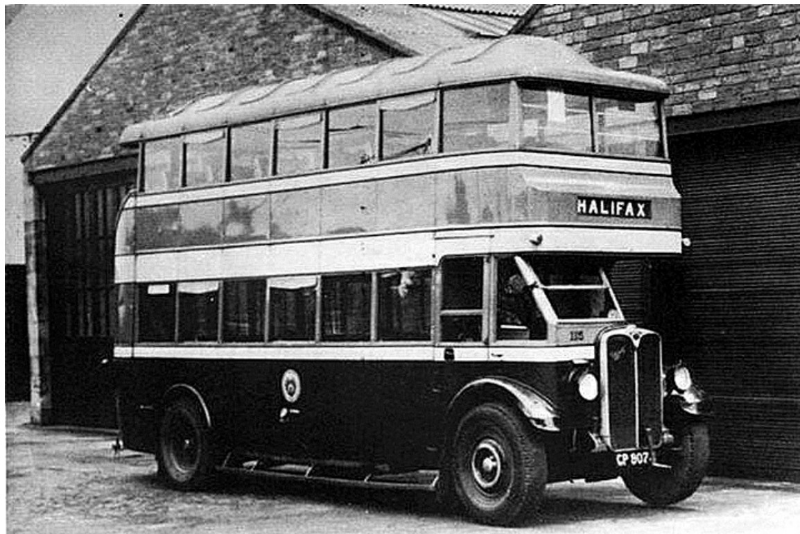
Halifax No. 115 (CP9078) was a 1931 AEC Regent with Hoyal 50-seat open staircase bodywork. (LTHL collection).
