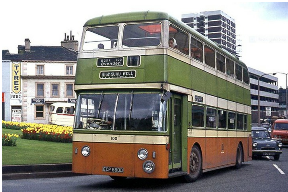
No. 100 (ECP680D) at the Cow Green/Bull Green roundabout in April 1972. It was a 1966 Daimler CRG6LX with Northern Counties 75-seat bodywork. (John Kaye).
