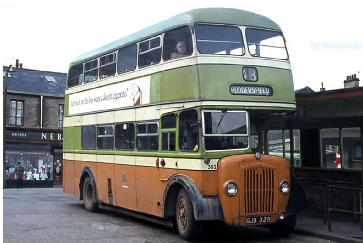
Seen here in Crossfields Bus Station is No. 302 (GJX329), a 1956 Daimler CVG6 with Roe 65-seat bodywork. Originally Halifax Corporation No. 17, it was transferred to the Joint Omnibus Committee fleet in 1971 as their No. 302 and passed to Calderdale JOC later that year. (John Kaye).
