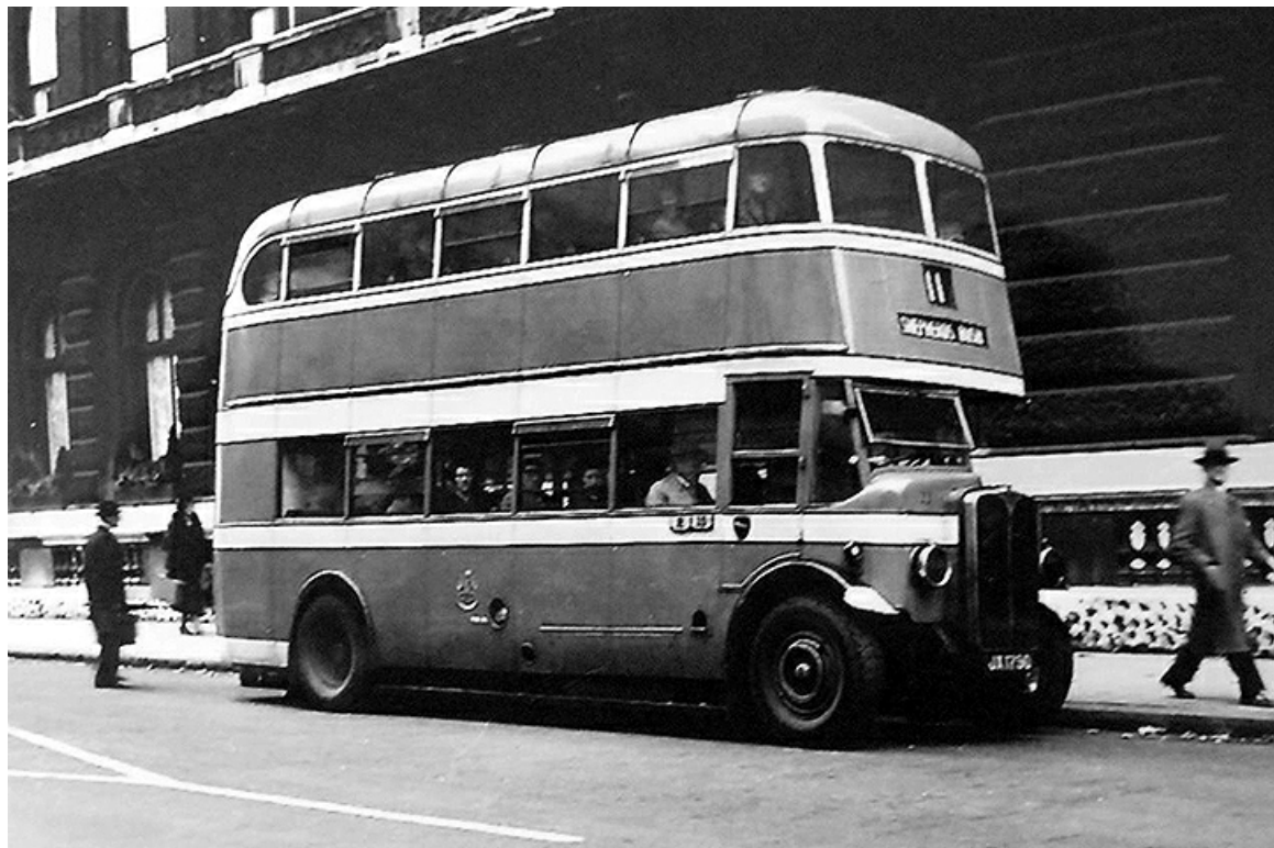
No. 11 (JX1790), a 1934 AEC Regent with Park Royal 54-seat bodywork, seen here whilst on loan to London Transport. (LTHL collection).
