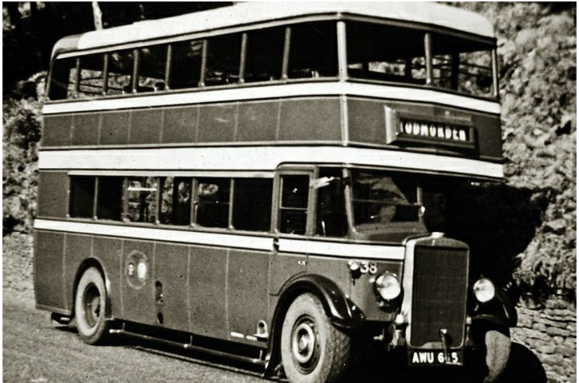
No. 38 (AWU665) was a 1935 Leyland TD4 with Leyland 52-seat lowbridge bodywork, owned by the London, Midland & Scottish Railway, following the formation of the JOC in 1931. (courtesy Pennine Heritage/Todmorden Antiquarian Society).
