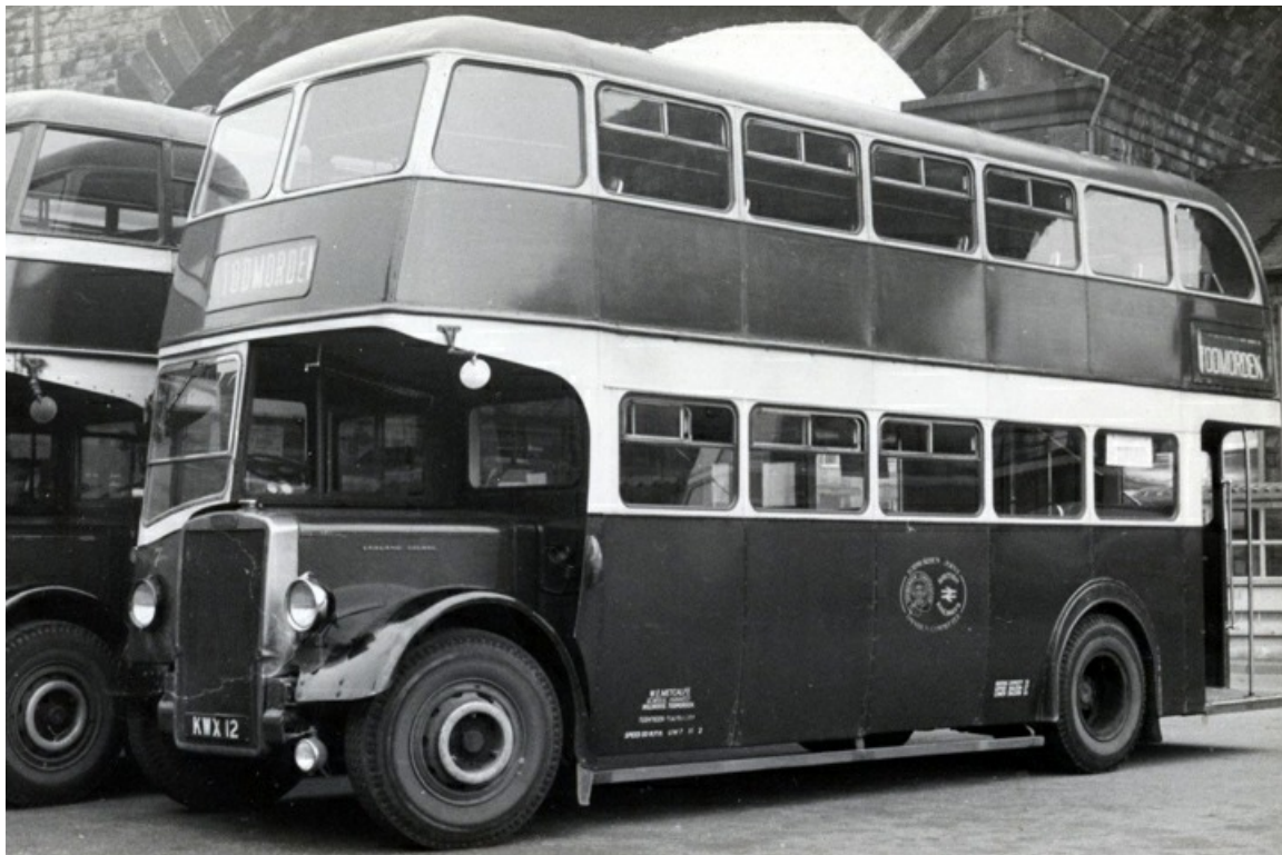
No. 7 (KWX12) was a 1951 Leyland PD2/12 with Leyland 53-seat bodywork owned by the Corporation. It passed to the Calderdale JOC in 1971 as their No. 353. (LTHL collection).
