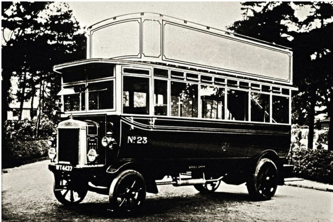
No. 23 (WT4437) was a 1924 Leyland SG2 with Leyland 51-seat bodywork. (courtesy Pennine Heritage/Todmorden Antiquarian Society).
