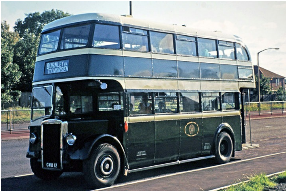
No. 2 (GWU12), a 1948 Leyland PD2/1 with Leyland 53-seat bodywork. This bus now survives in preservation. (courtesy Pennine Heritage/Todmorden Antiquarian Society).
