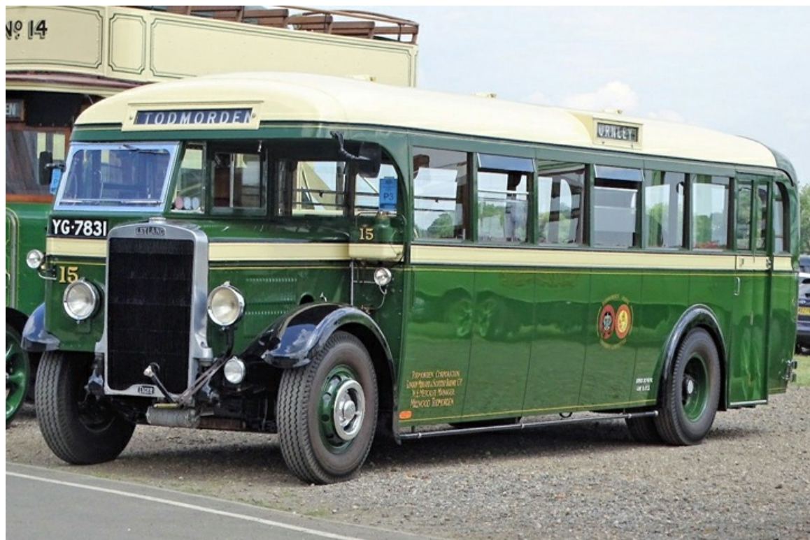
No. 15 (YG7831) in the Todmorden JOC fleet was this beautifully preserved 1934 Leyland TS6 with Northern Counties 36-seat bodywork. (LTHL collection).
