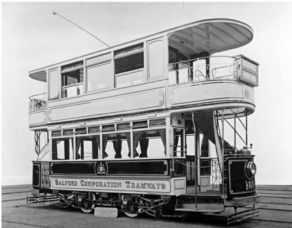
No. 185 was a 1913 top-covered car built by the United Electric Car Co of Preston, seen here when new with open ended top cover. (LTHL collection).
