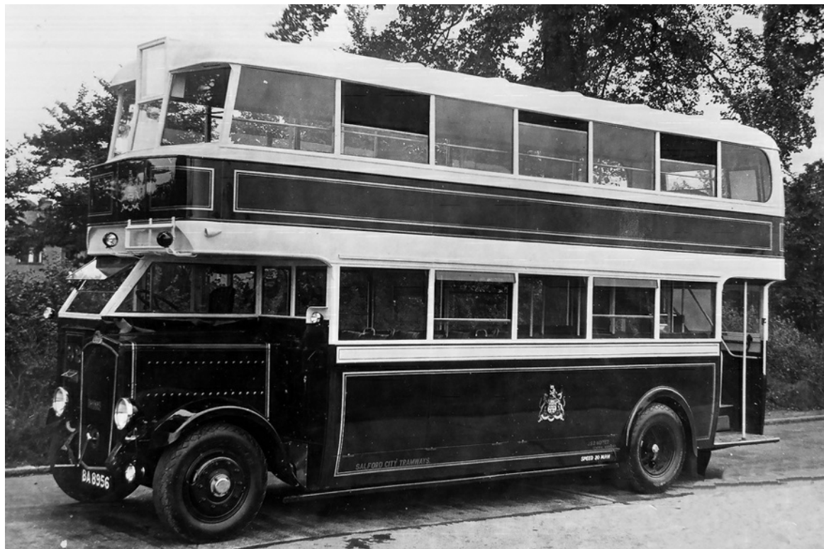
No. 92 (BA8956) was a 1930 Dennis Lance I with Park Royal (the successor to Hall Lewis) 50-seat lowbridge bodywork. (Bus Archive).
