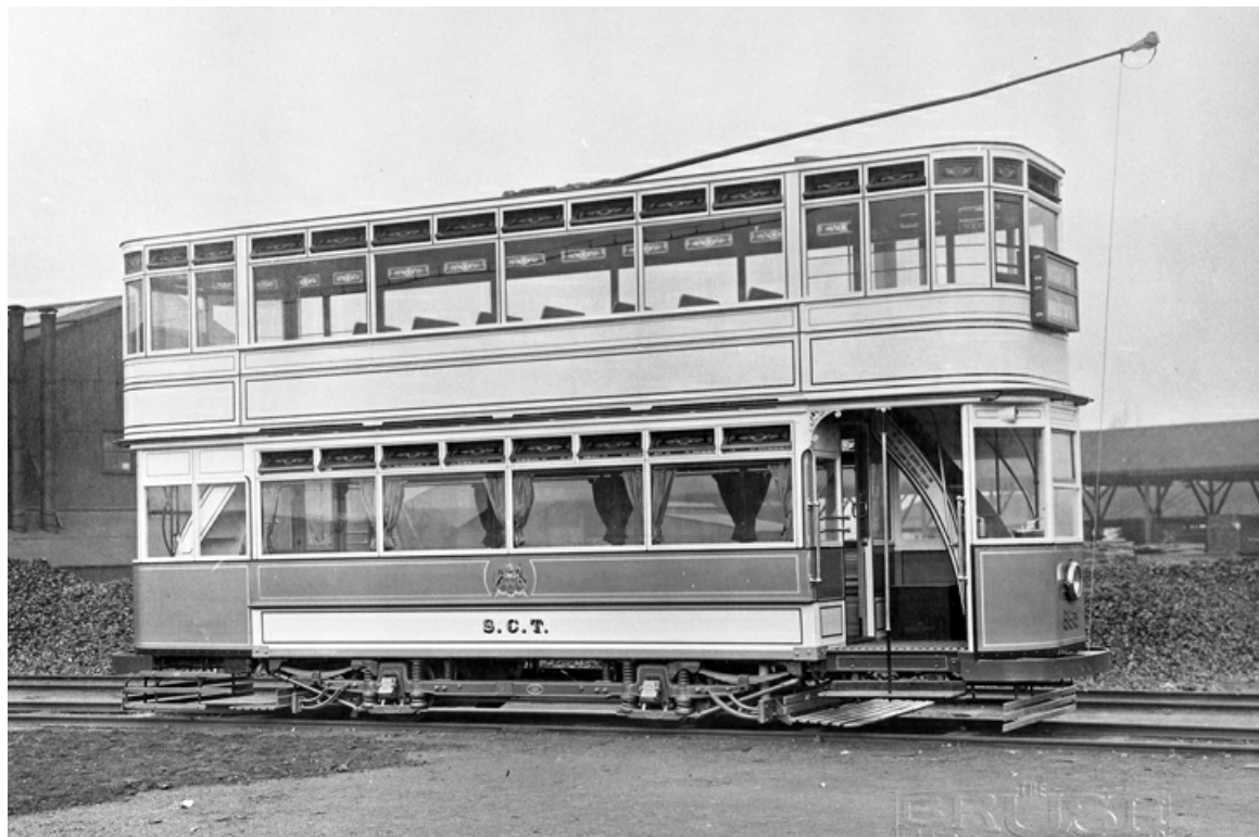
No. 225 was one of six special low-built all-enclosed cars that enabled them to pass under the Great Ducie Street bridge connecting Manchester Exchange and Victoria Stations. (LTHL collection).
