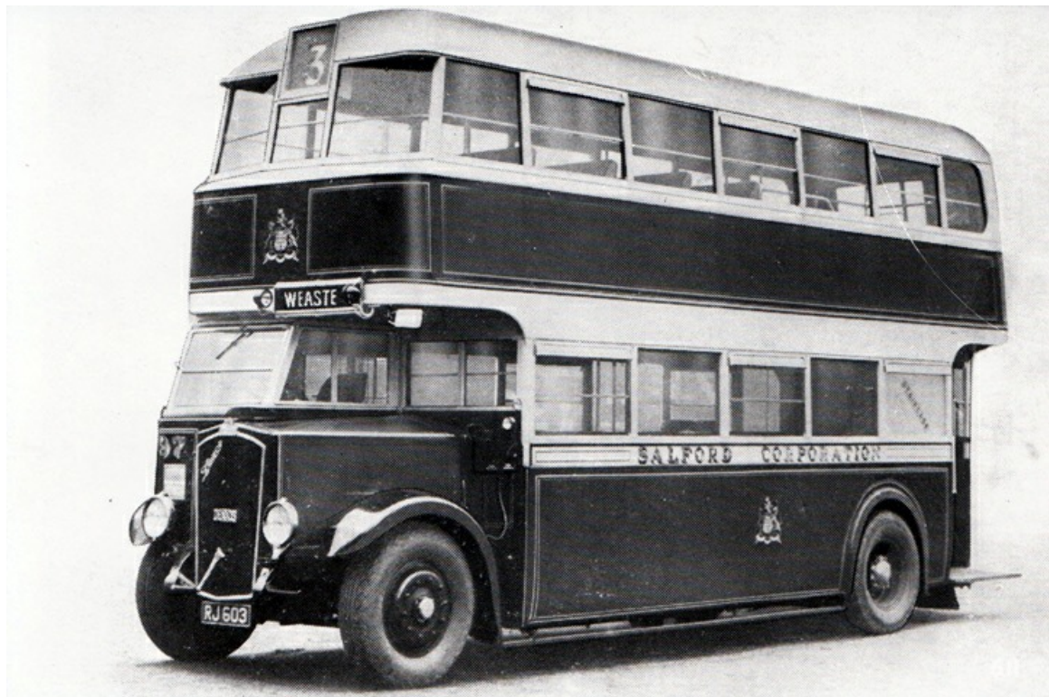
Salford No. 97 (RJ603), was this 1932 Dennis Lance II with Strachans 53-seat bodywork. (Bus Archive).
