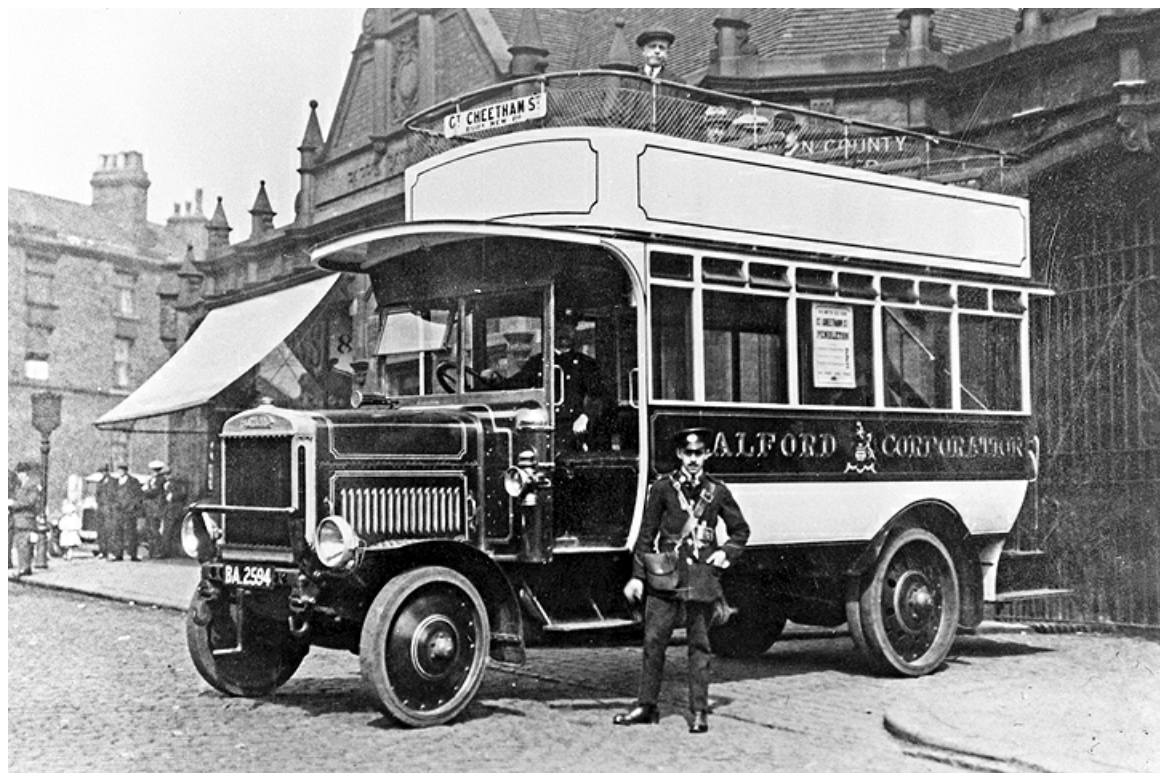
Salford's first bus was No. 1 (BA2594) a Leyland 31M of 1920 with 45-seat double-deck bodywork. (Bus Archive).
