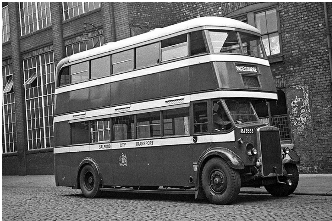
Salford's practice of gap-filling meant batches of similar vehicles were not always consecutively numbered. This is No. 29 (RJ3533) of 1934, a Leyland TD4 with MCCW H26/22R bodywork. (LTHL collection).
