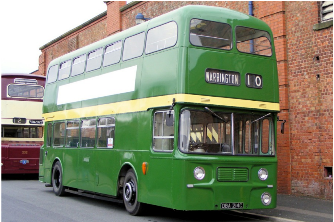
Preserved Salford Leyland PDR1/1 with MCCW bodywork No. 214 (DBA214C), dating from 1965, seen here outside the Museum of Transport, Manchester. (LTHL collection).
