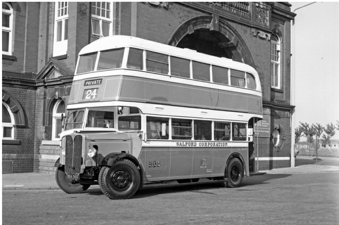
No. 235 (BBA560), a 1940 AEC Regent with Park Royal bodywork became a driver training bus after withdrawal in 1948 which enabled it to survive into preservation and it is seen here after restoration into original red and cream livery. (LTHL collection).
