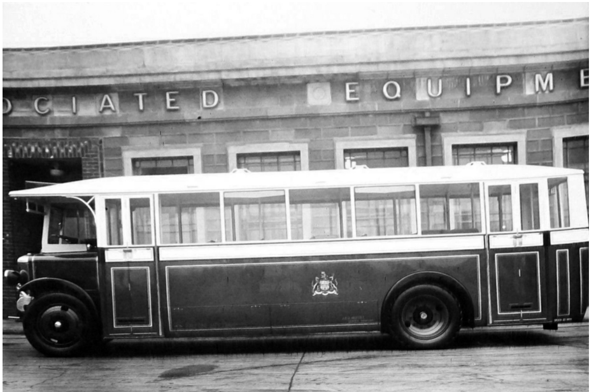
In 1929 Salford took delivery of a number of AEC 426 chassis with Hall Lewis 32-seat dual entrance bodywork. This is one of those vehicles, although its exact identity is uncertain - it is pictured here at the AEC works before delivery. (LTHL collection).
