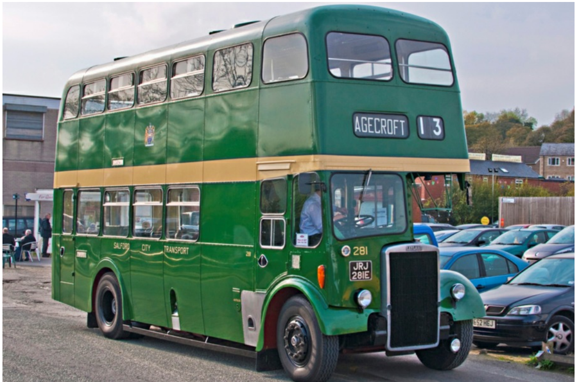
After a brief flirtation with rear-engined vehicles Salford returned to the front-engined Leyland PD2/40 for their 1966 and 1967 purchases. This is No. 281 (JRJ281E) dating from 1967 with MCCW 64-seat bodywork. (LTHL collection).
