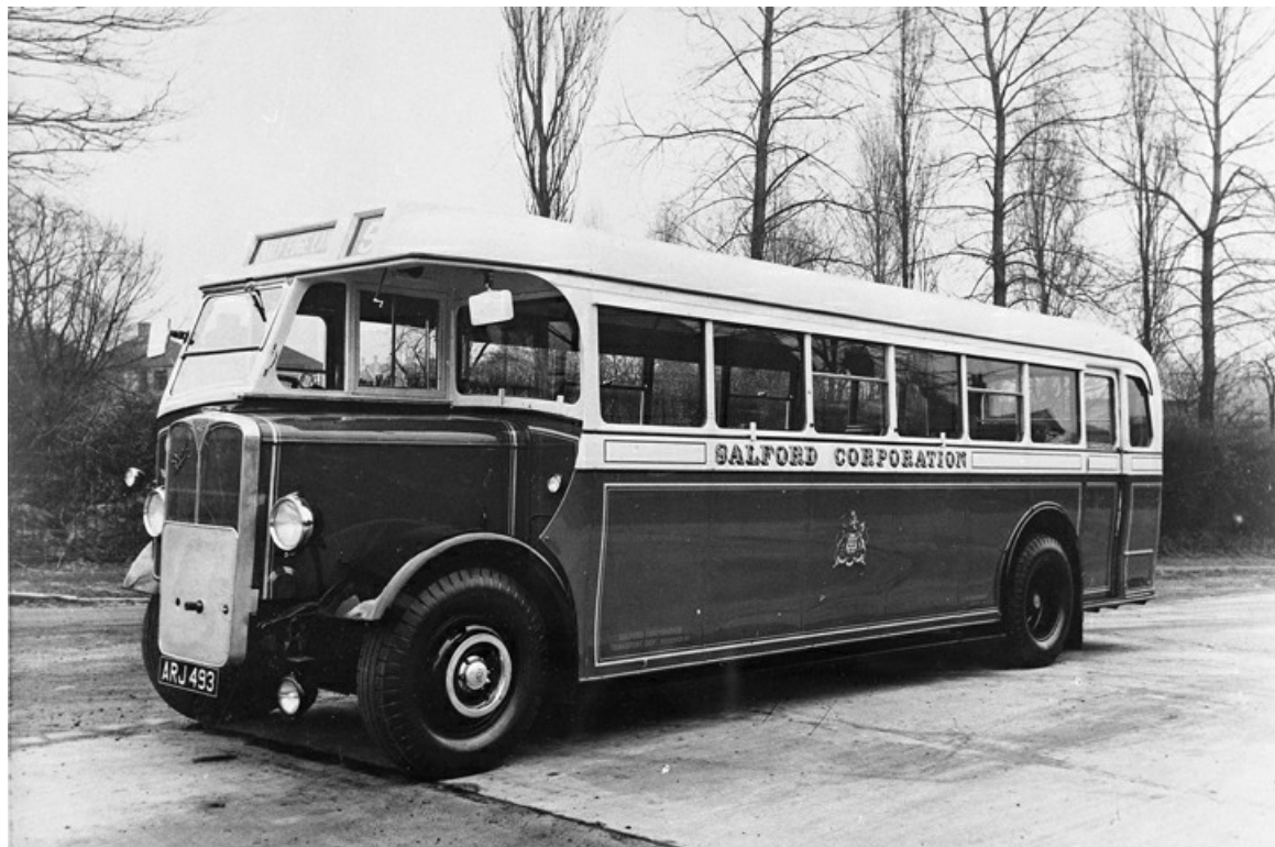
Salford's choice for single-deck chassis was the AEC Regal. This is No. 66 (AERJ493) dating from 1939 and carrying English Electric B30R bodywork. (Bus Archive).
