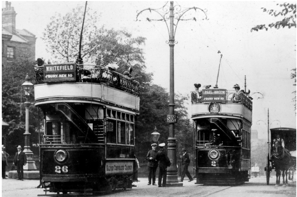
Salford Corporation trams No. 2 and No. 26 at Kersal. Both are 1901 Milnes-built 55-seat open top 4-wheel cars on Brill 21E trucks and in original form; later top-covered, fitted with vestibules and new staircases by Massey Brothers between 1926 and 1928. (LTHL collection).
