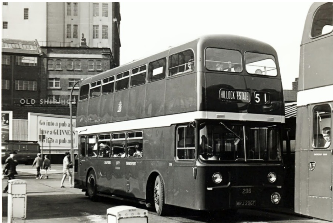
No. 296 (MRJ296F) was a 1968 Leyland PDR1/1 Atlantean with MCCW bodywork. (Christopher Leach).
