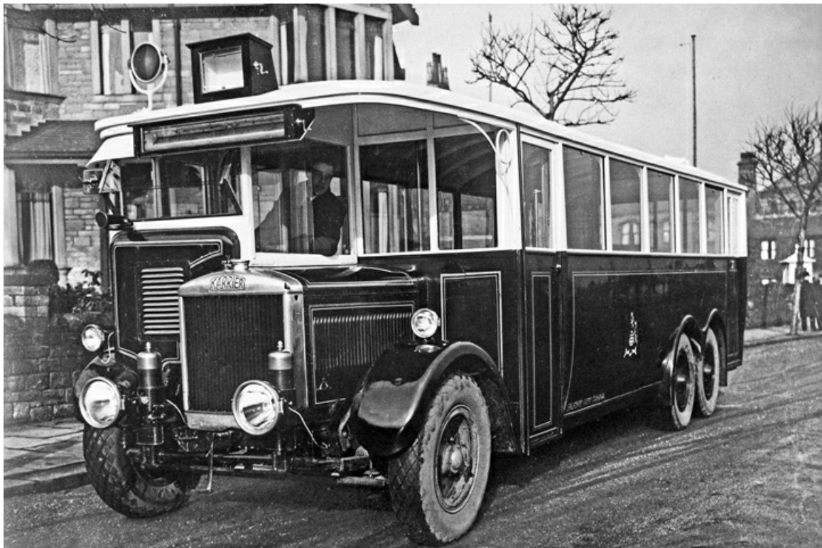
No. 22 (BA6261) was a 1927 six-wheeled Karrier WL6/1 with Massey B32D bodywork. (Bus Archive).
