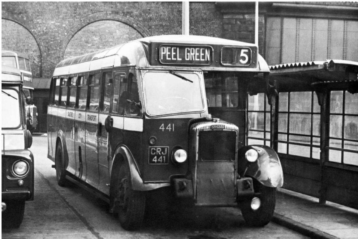
1950 Daimler CVG6 No. 441 (CRJ441) with Burlingham 33-seat rear entrance bodywork, seen here in Victoria Bus Station awaiting departure to Peel Green. It was withdrawn in 1962. (LTHL collection).
