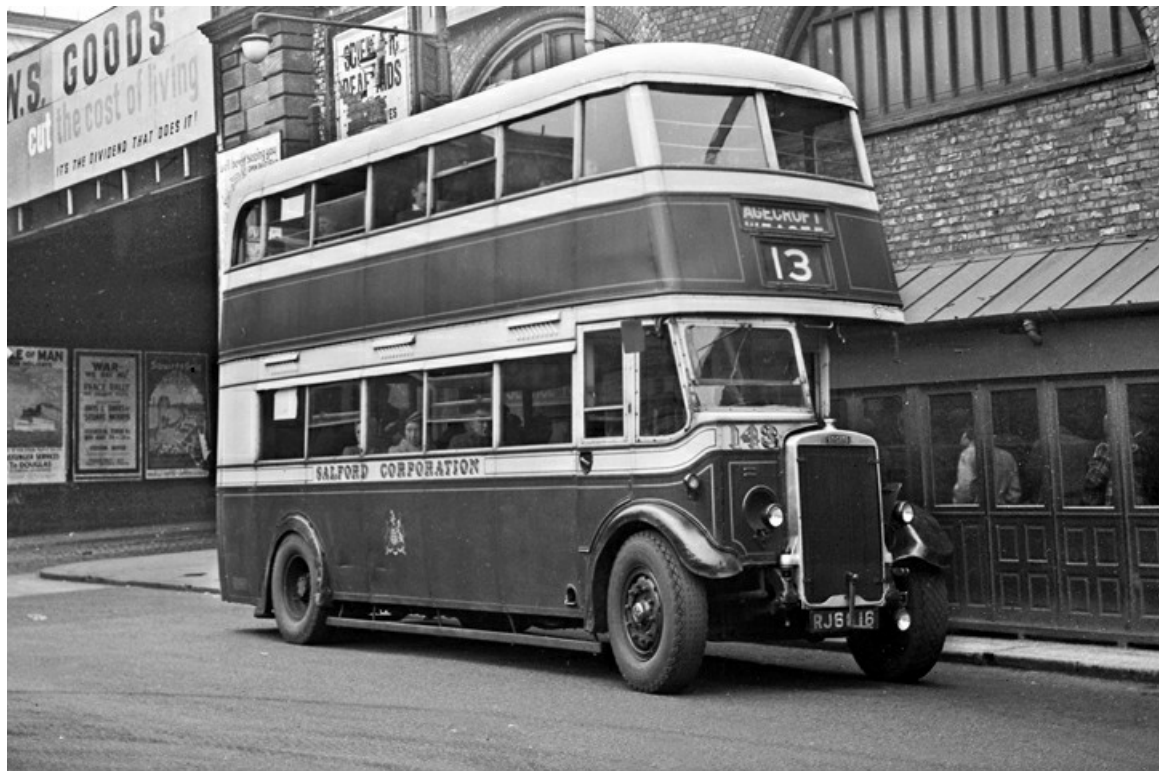
No. 143 (RJ6616), seen here in Victoria Bus Station awaiting departure to Agecroft still sporting the red and cream livery, was a 1936 Leyland TD4 with MCCW H26/22R bodywork. (LTHL collection).
