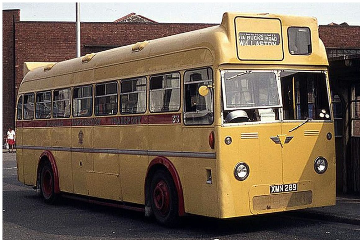
Douglas Corporation No. 33 (XMN289) a 1958 AEC Reliance with unusual Mulliner 42-seat bodywork. (Donald Hudson).
