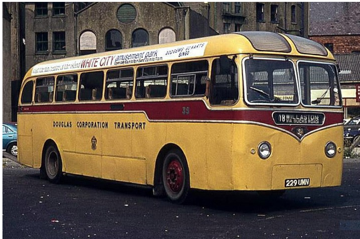
Douglas Corporation No 35 (229UMN) a 1957 Leyland Tiger Cub PSUC1/2 with Duple Midland bodywork, one of 8 vehicles acquired from Lancashire United in 1970. (Donald Hudson).
