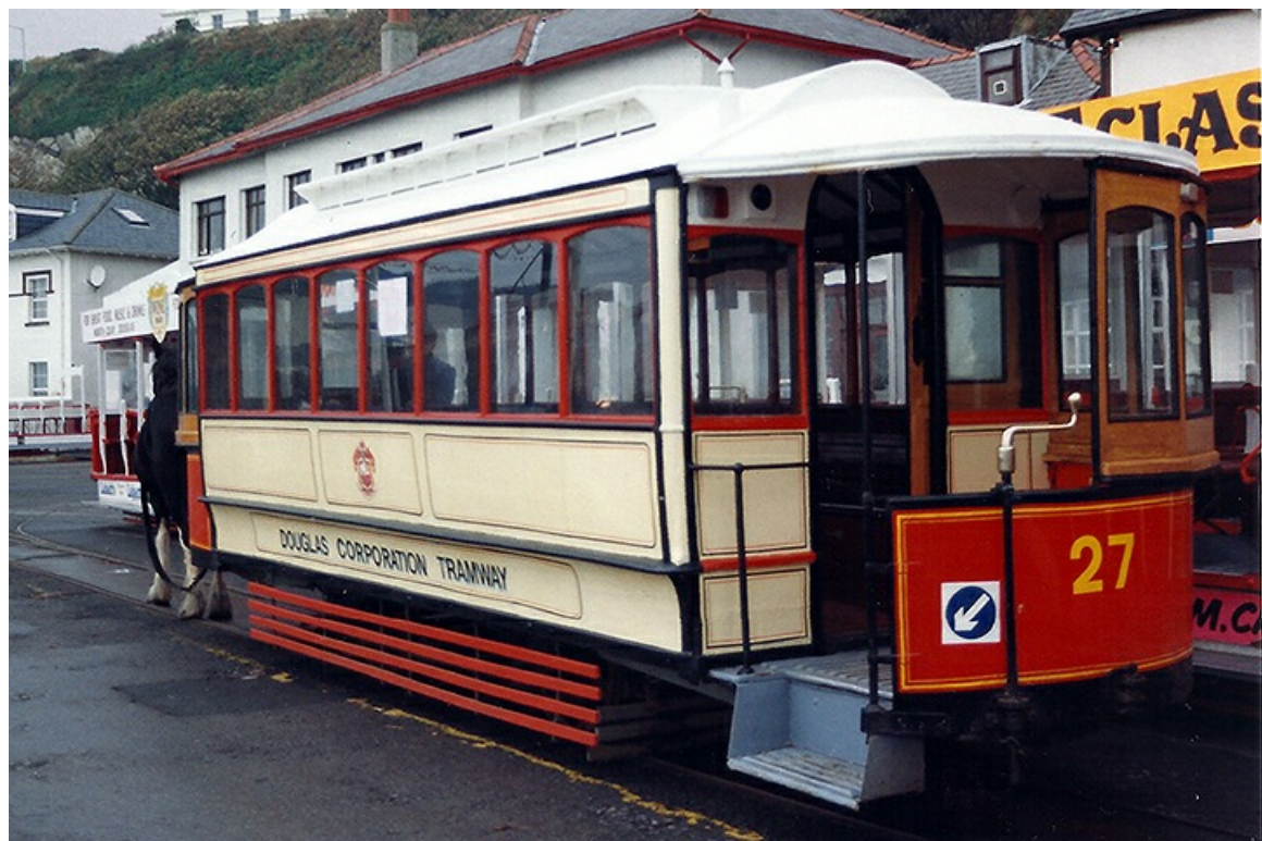
Douglas horse tram No. 27 built in 1892 by George Milnes & Company and seating 30. (John Blannin).
