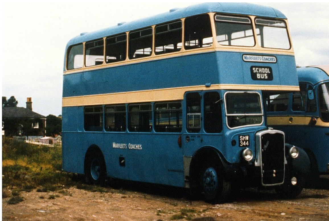
SHW344 was purchased specifically for school contract work and was a 1954 Bristol KSW6G with ECW 60-seat bodywork that was originally Bristol Omnibus Company No. 8174. (LTHL collection).
