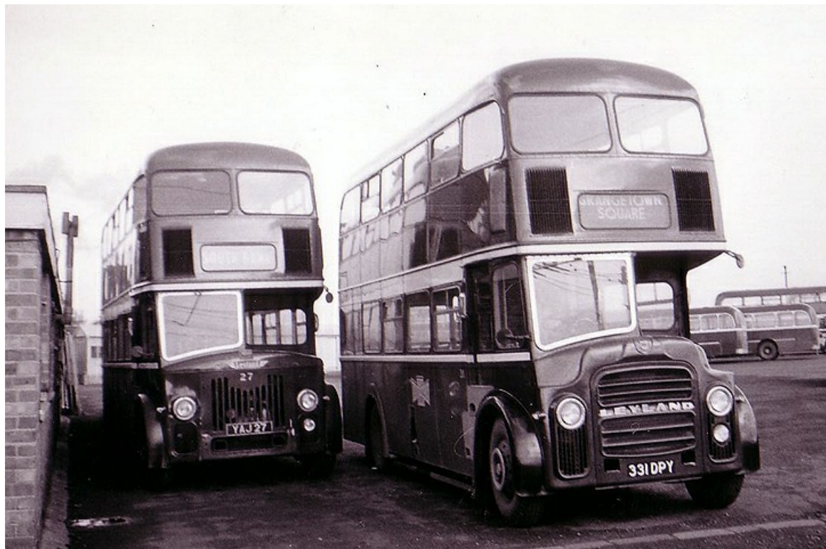
No. 31 (331DPY) was a 1963 Leyland PD2A/27 with Roe H33/28R bodywork, alongside 1962 Leyland PD2/27 No. 27 (YAJ27) originally with Roe H35/28R bodywork. (John Heighway courtesy Malcolm Jones).
