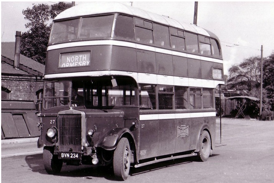
No. 27 (BVN234) was a 1941 Leyland TD7 with Roe H31/25R bodywork, one of a pair which were the first double-deck vehicles owned by Tees-side. (John Heighway courtesy Malcolm Jones).
