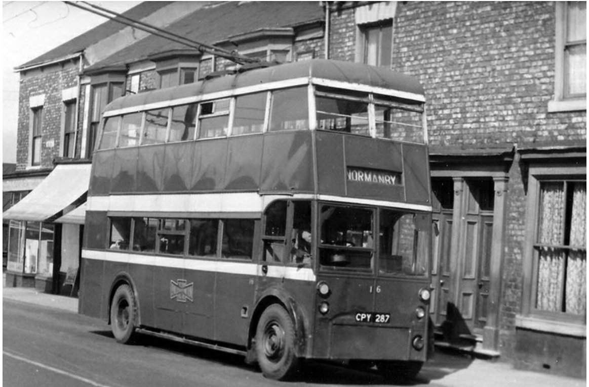
No. 16 (CPY287), a 1944 Sunbeam W with Weymann utility bodywork, which was rebuilt in 1958 by the Company with local builder Edmond. It was re-bodied by Roe in 1960 and passed to Teesside Municipal Transport in April 1968. (John Heighway courtesy Malcolm Jones).
