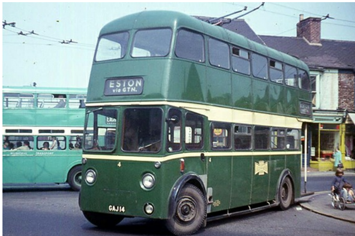
1950 Sunbeam F4 No. 4 (GAJ14) originally with East Lancs 56-seat bodywork but seen here after being re-bodied by Roe with a 61-seat body was one of the final batch of trolleybuses purchased. (John Kaye).
