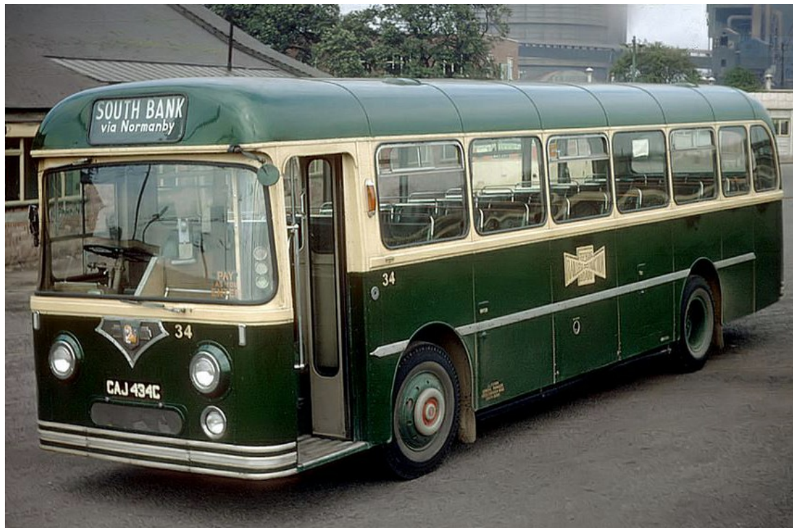
1965 Leyland Leopard No. 34 (CAJ434C) with Roe 45-seat bus bodywork. It passed to Teesside Municipal Transport in 1968. (LTHL collection).
