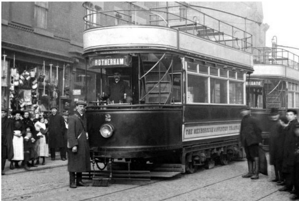
Car No. 2 in original condition with open top. It was a 1907 Brush-built 4-wheel car on Mountain & Gibson trucks seating 22 on the lower deck and 32 on the upper. It received a top-cover in 1908. (LTHL collection).
