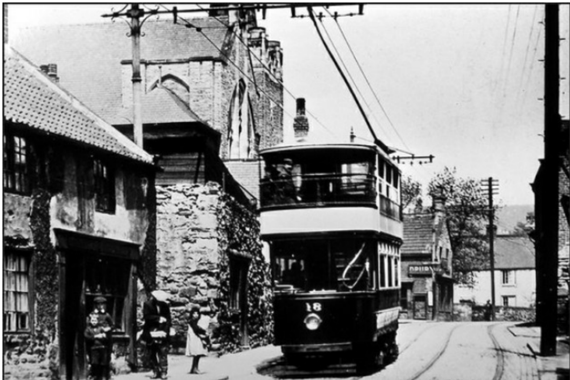
No. 18 of 1908 was a double-deck top-covered 4-wheel car on Brush trucks with Brush 54-seat bodywork. (LTHL collection).
