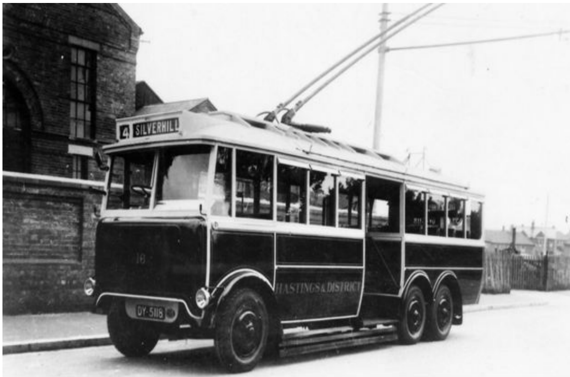
Seen here with its original owners Hastings & District Tramway Company is DY5118 a 1928 Guy BT32 with Ransomes 32-seat bodywork. It became Mexborough & Swinton No. 70 in 1942. (LTHL collection).
