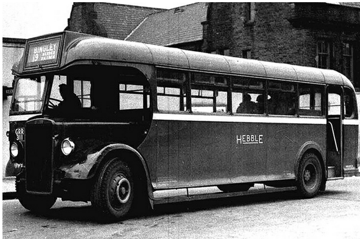
Hebble No. 1 (GRR311) was a 1947 Leyland PS1 with Weymann 35-seat rear-entrance bodywork ex-East Midland Motor Services (No. H1). It was re-numbered 101 in 1957 and withdrawn in 1959. (John Kaye).
