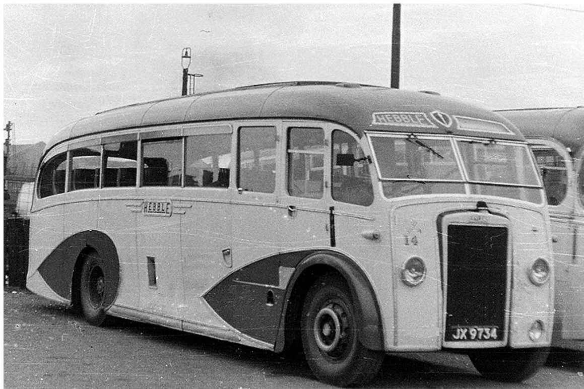
No. 14 (JX9734) was a 1947 Leyland PS1, originally fitted with second-hand body when new but re-bodied with this Windover FC33F body in 1952. (LTHL collection).
