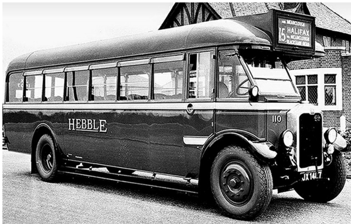
Hebble No. 110 (JX1407), a 1934 Albion PW67 with Brush 32-seat front entrance bus bodywork. (Bus Archive).
