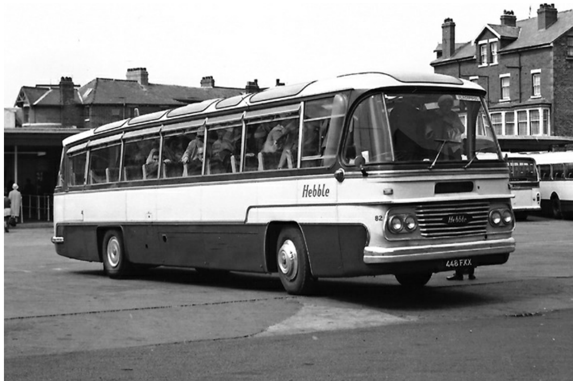
No. 82 (448FXX) was a 1963 AEC Reliance that came second-hand from Samuelsons New Transport in 1968. It had a Duple C49C body. (Bus Archive).
