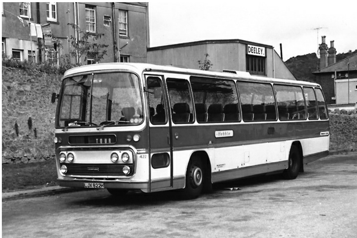
No. 422 (LJX822H) was a 1970 Leyland Leopard PSU3A/4R with Plaxton C47F coachwork. It was re-numbered 57 in 1971 and passed to National Travel (North East) in 1974. (Bus Archive).
