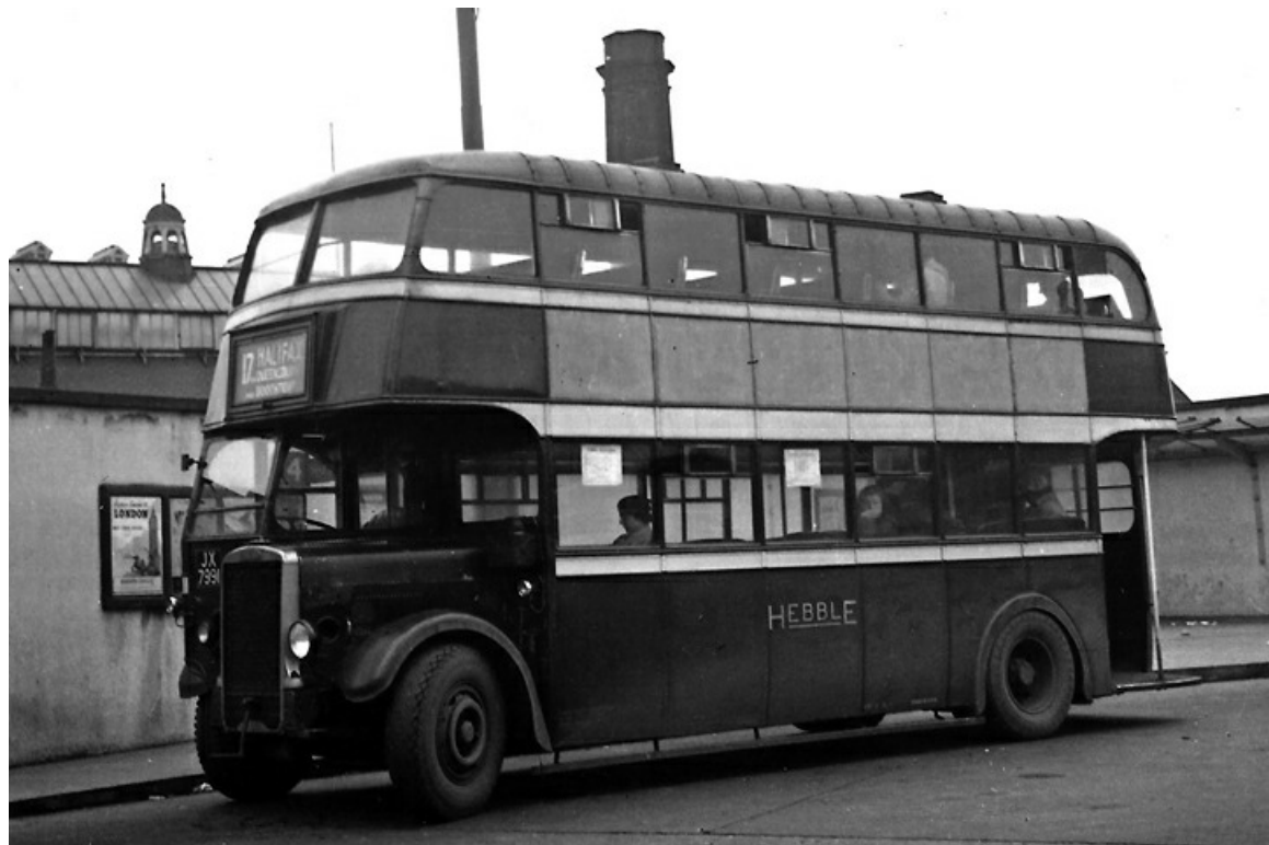
No. 161 (JX7991) was a 1940 Leyland TD5 with Eastern Coach Works L27/26R bodywork. (Bus Archive).
