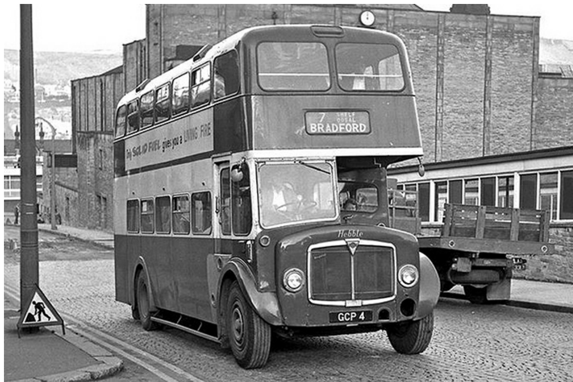
GCP4 was a 1956 AEC Regent V with Weymann 55-seat lowbridge bodywork. Originally No. 76 it became No. 276 in 1957 and was withdrawn in 1968. (LTHL collection).
