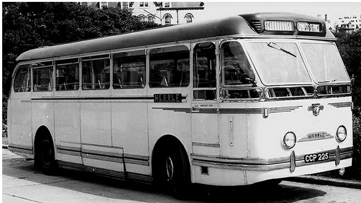
1952 Leyland Royal Tiger No. 55 (CCP225) with distinctive Leyland 41-seat centre-entrance bodywork. It became No. 26 in the 1957 re-numbering and was withdrawn in 1964. (LTHL collection).
