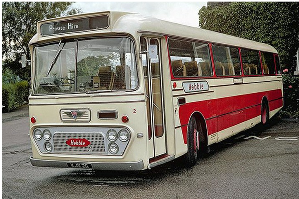
No. 2 (KJX2G) a 1969 AEC Reliance with Alexander 49-seat coachwork. It was re-numbered 502 in 1970 and passed to West Riding Automobile Co. in 1971 as their No. 271. (LTHL collection).
