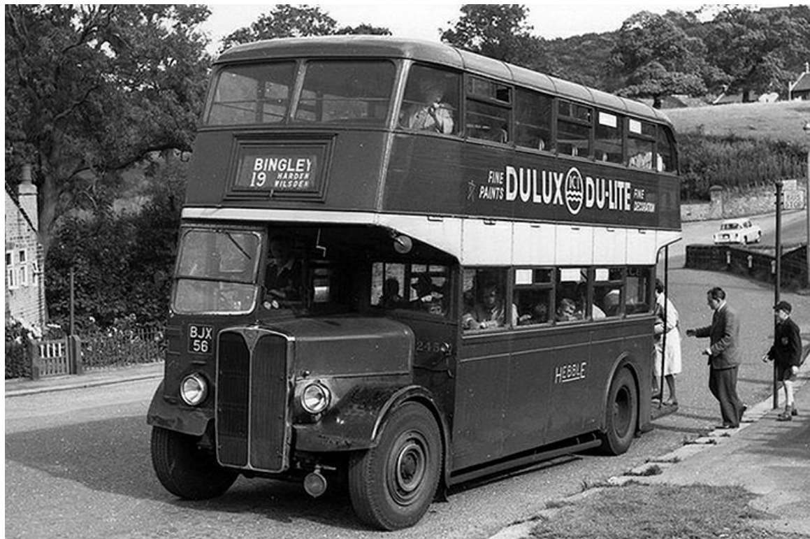
No. 245 (BJX56), a 1950 AEC Regent III with Roe 53-seat lowbridge bodywork, originally No. 45 it was re-numbered in 1957. It was withdrawn in 1962. (LTHL collection).
