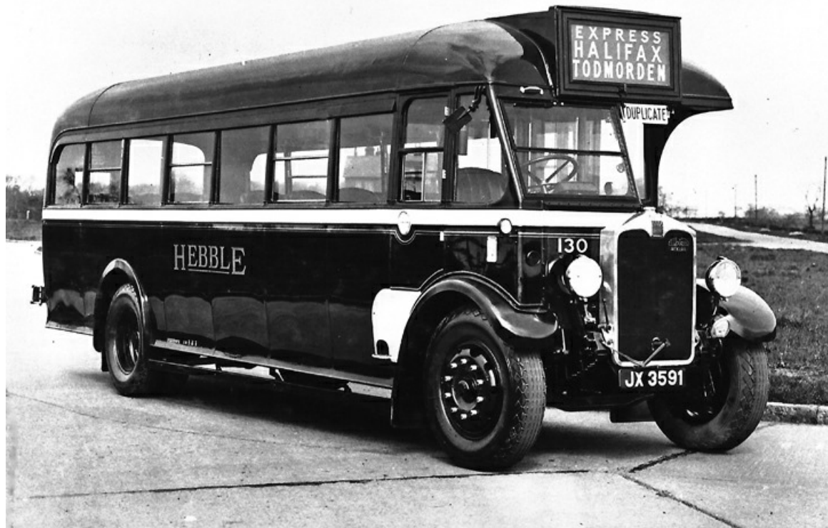
No. 130 (JX3591) was an Albion PW69 with Roe B32F bodywork. It had been withdrawn by 1946. (Bus Archive).
