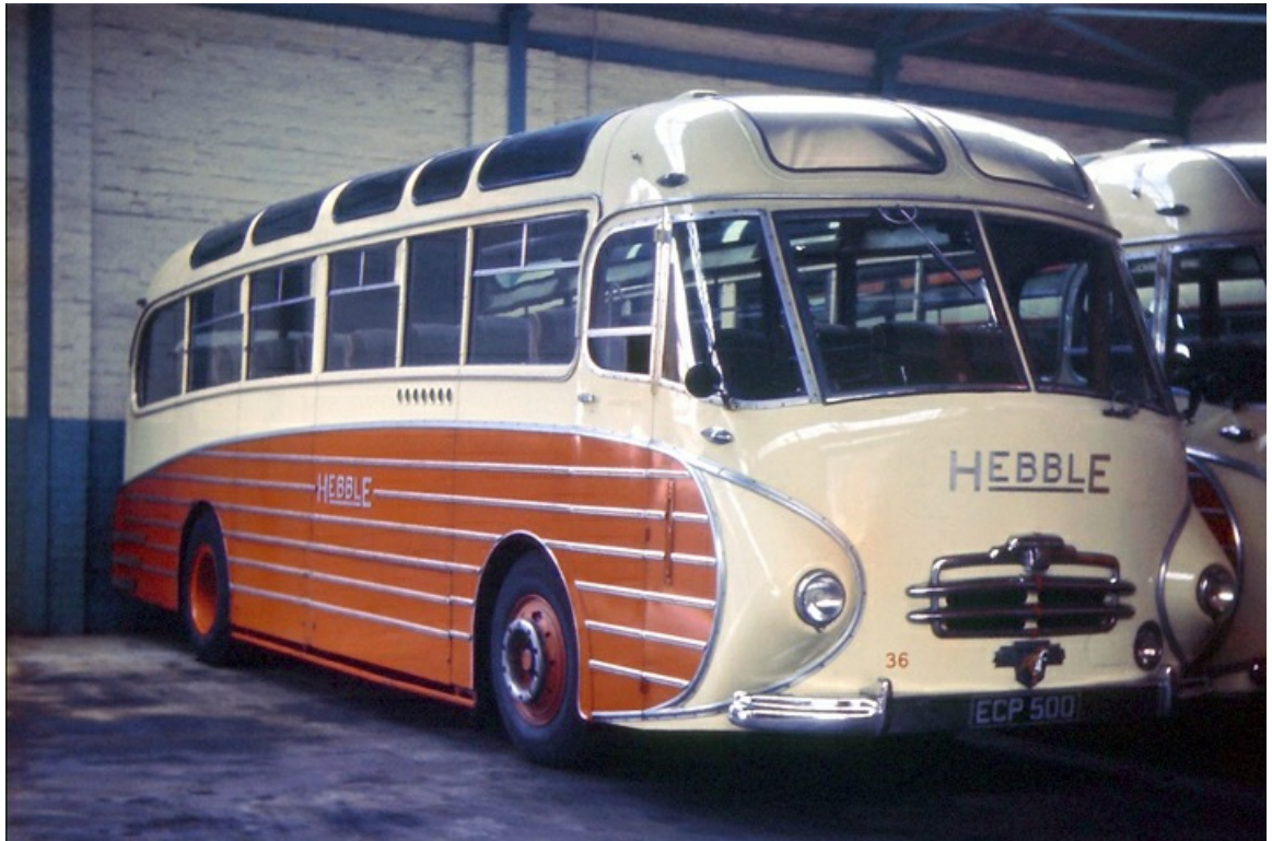
No. 36 (ECP500) was a 1954 Leyland PSU1/15 'Royal Tiger' with Bellhouse-Hartwell C37C coachwork. Originally No. 74 it was re-numbered in June 1957 and withdrawn in 1966. (John Huddleston).
