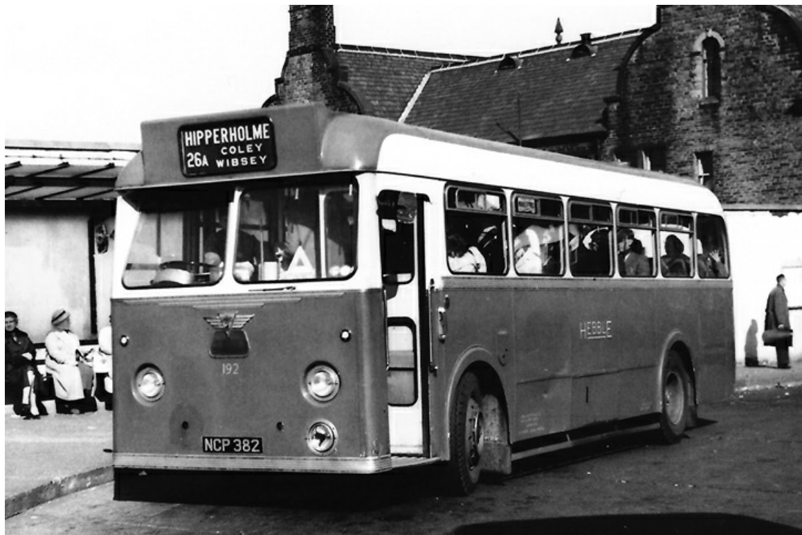
No. 192 (NCP382), a 1961 AEC Reliance 2MU3RV with Park Royal B43F bodywork. It was re-numbered 660 in 1970 and withdrawn the following year. (Bus Archive).
