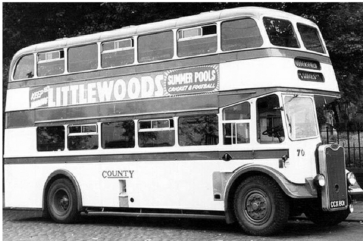
1945 Guy Arab II No. 70 (CCX801) with Roe lowbridge 53-seat bodywork, which replaced the original body (also by Roe) in 1953. (LTHL collection).
