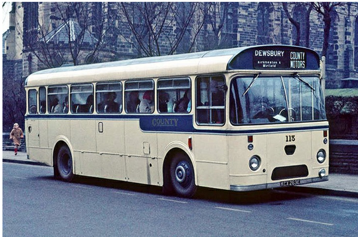
One of the last vehicles to enter service was No. 113 (KCX263E) a 1966 Leyland Tiger Cub PSUC1/12 with Marshall 45-seat dual purpose bodywork. (Linden Edwards courtesy John Stringer).
