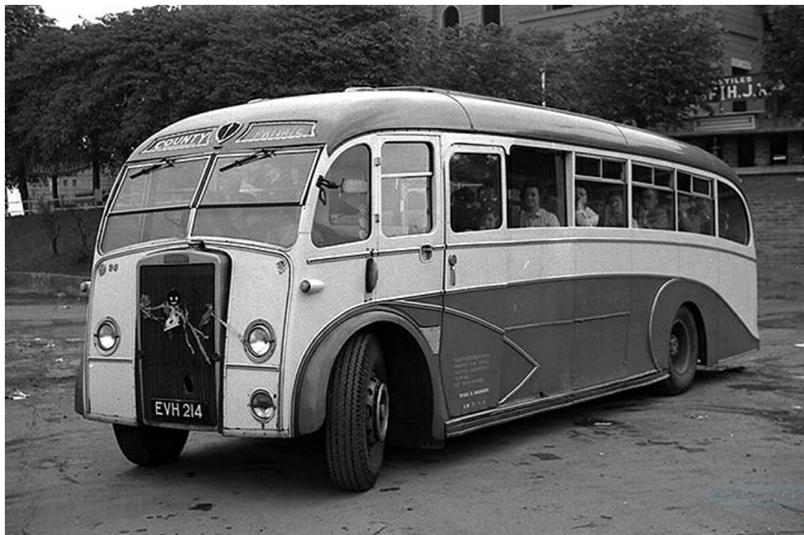
No.86 (EVH214) was a 1949 Leyland PS2 originally with a Roe half-cab body but was re-bodied in 1954 by Windover with a full front 35-seat body. (John Boylett courtesy John Kaye).
