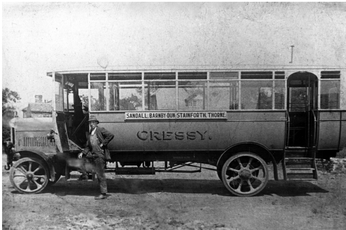
WT8728 was a Leyland RAF chassis with Leyland B32R bodywork acquired in 1925. (Bus Archive)
