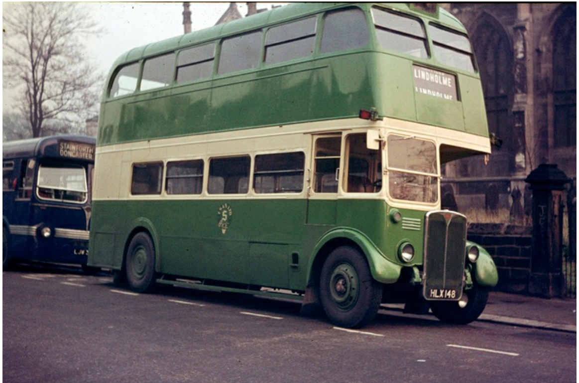
An unusual purchase in 1963 was HLX148 ex-London Transport RT331 an AEC Regent III with Weymann H30/26R bodywork dating from 1948. (Richard Simons).
