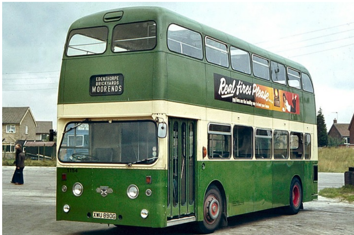
XWU890G was a 1969 Leyland PDR1/1 with Roe H44/31F bodywork. It is seen here after acquisition by South Yorkshire PTE wearing its new number - 1154. (Claire Pendrous).
