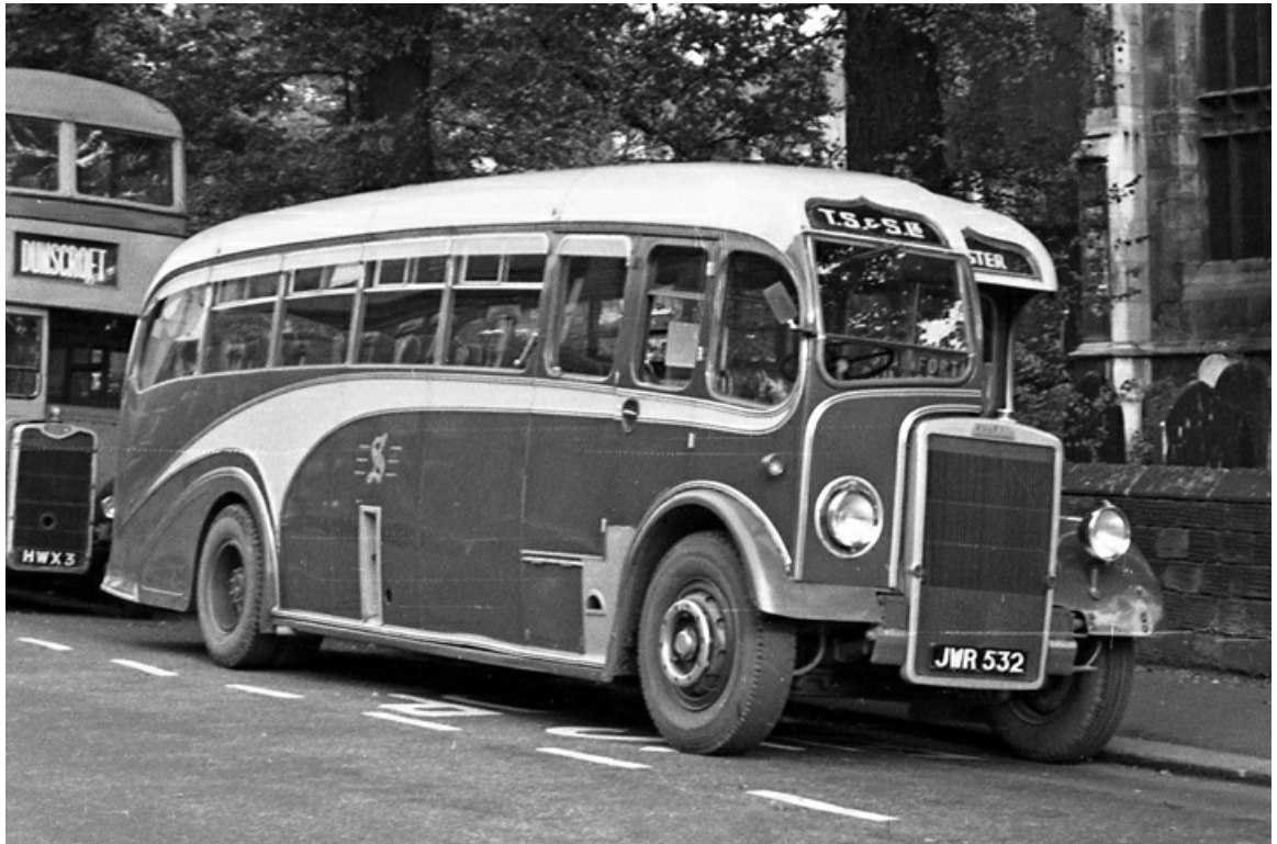
JWR532 was a Leyland PS1/1 with Yeates 33-seat coachwork, one of two purchased in 1949. (Bus Archive).
