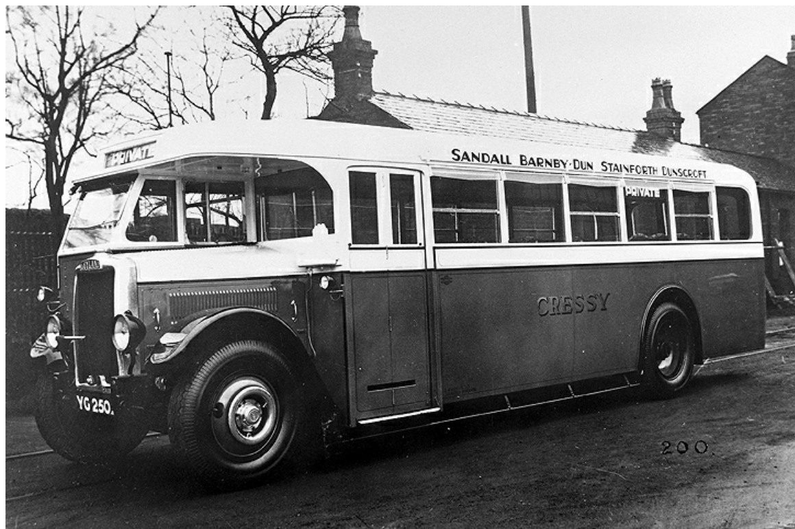
YG2501, seen here when new, was a 1932 Leyland TS4 with Roberts C32F coachwork. (Bus Archive)
