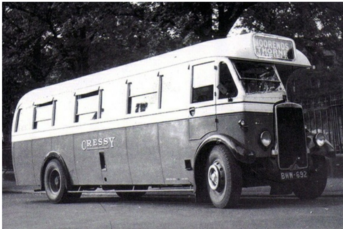
No. 9 (BWW692) was a 1937 Leyland LT7 with Barnaby 34-seat bus body. It was re-bodied again in 1949 with a 33-seat Barnaby coach body, but was withdrawn just two years later in 1951. (LTHL collection).
