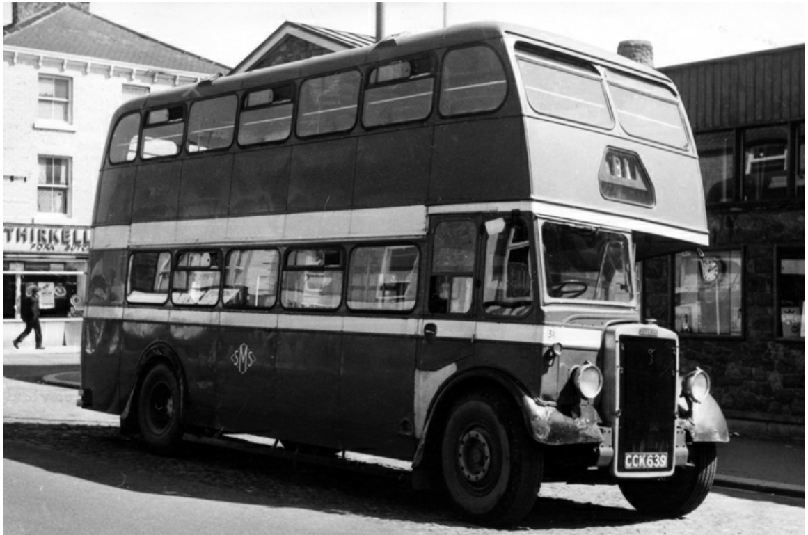
No. 31 (CCK639) was 1949 Leyland PD2/3 'Titan' with Brush lowbridge L27/26R bodywork that was formerly No. 2663 in the fleet of Ribble Motor Services. (Geoff Stainthorpe).
