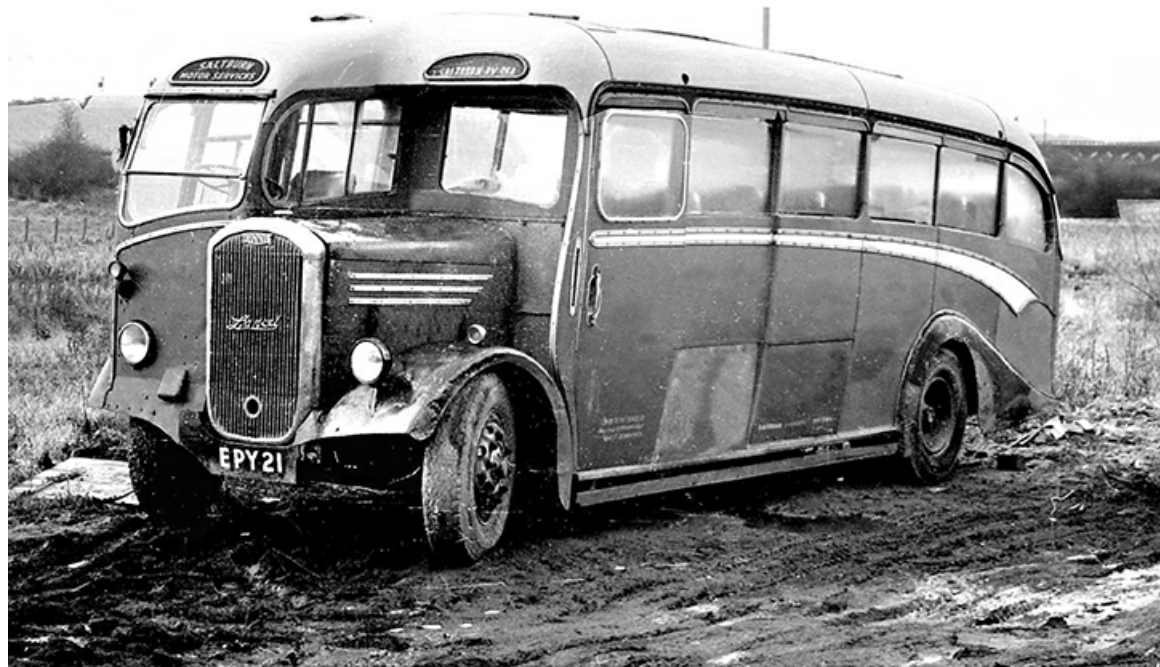
No. 28 (EPY21) was a Dennis Lancet with Duple 35-seat coachwork, dating from 1948. (LTHL collection).
