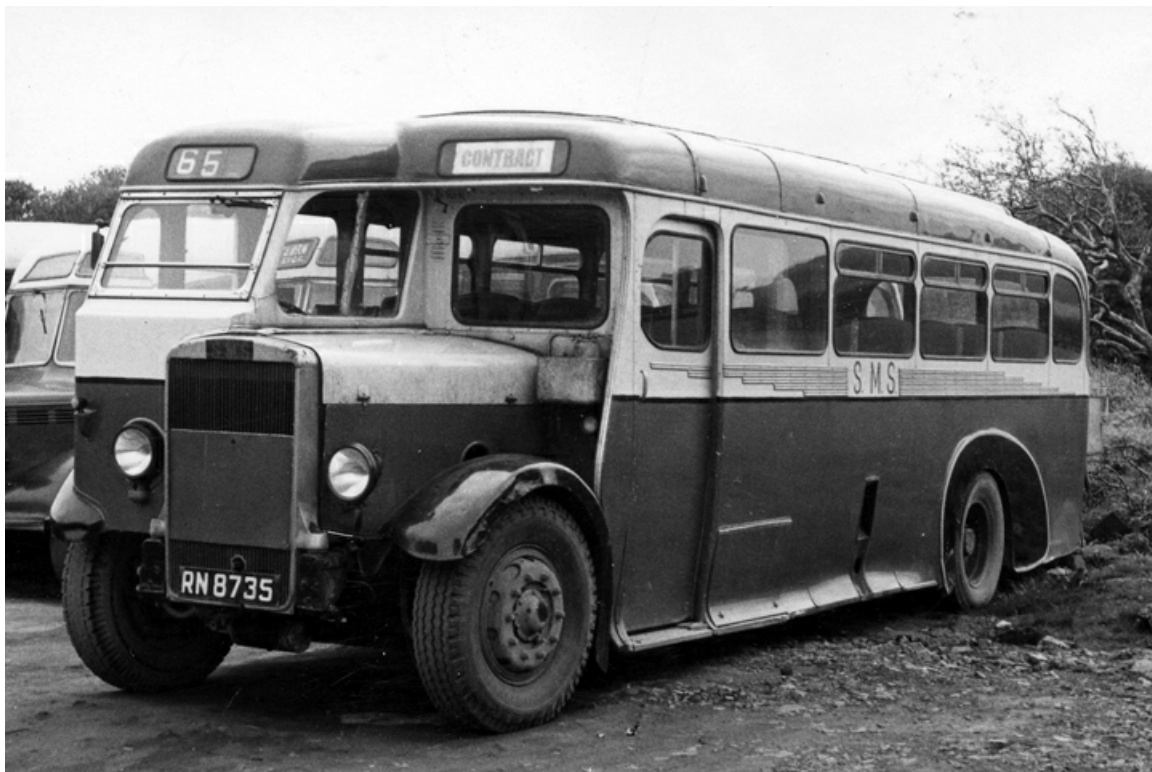
No. 35 (RN8735) was a second-hand acquisition from Ribble Motor Services in 1957. It was a 1939 Leyland TS8 with Duple C31F coachwork. (Geoff Stainthorpe).
