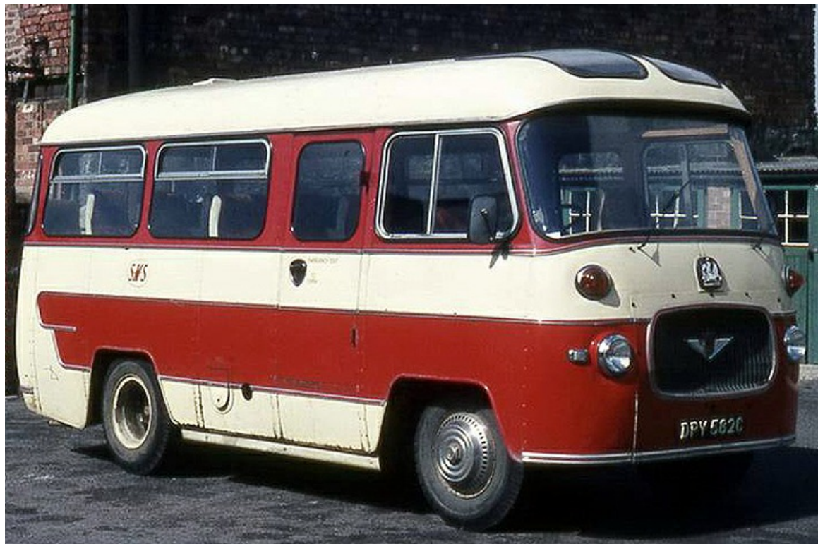
DPY582C was a 1965 Bedford J2SZ10 with Duple 19-seat coachwork. It was withdrawn in 1972. (Donald Hudson).
