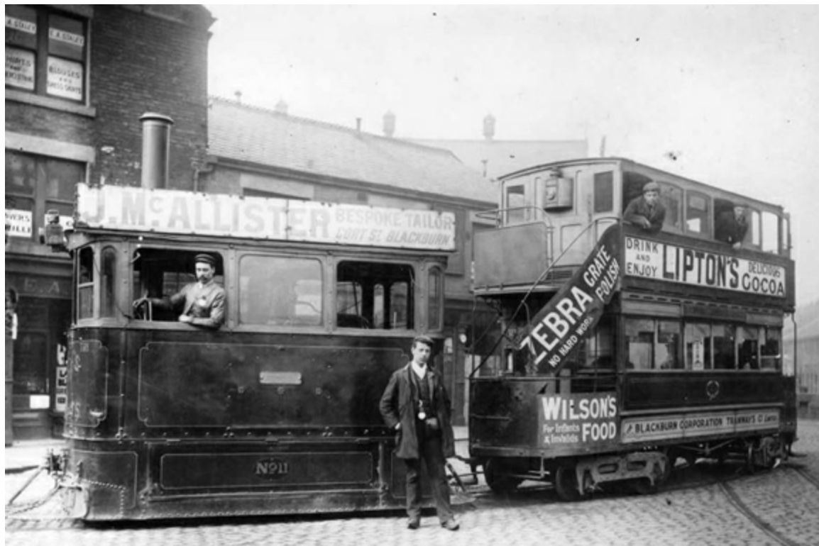
Thomas Green loco No. 11 and Falcon trailer car No. 13. The Falcon trailers were shorter than the Ashbury trailers and seated just 18 on the upper deck and 24 on the lower. (LTHL collection).
