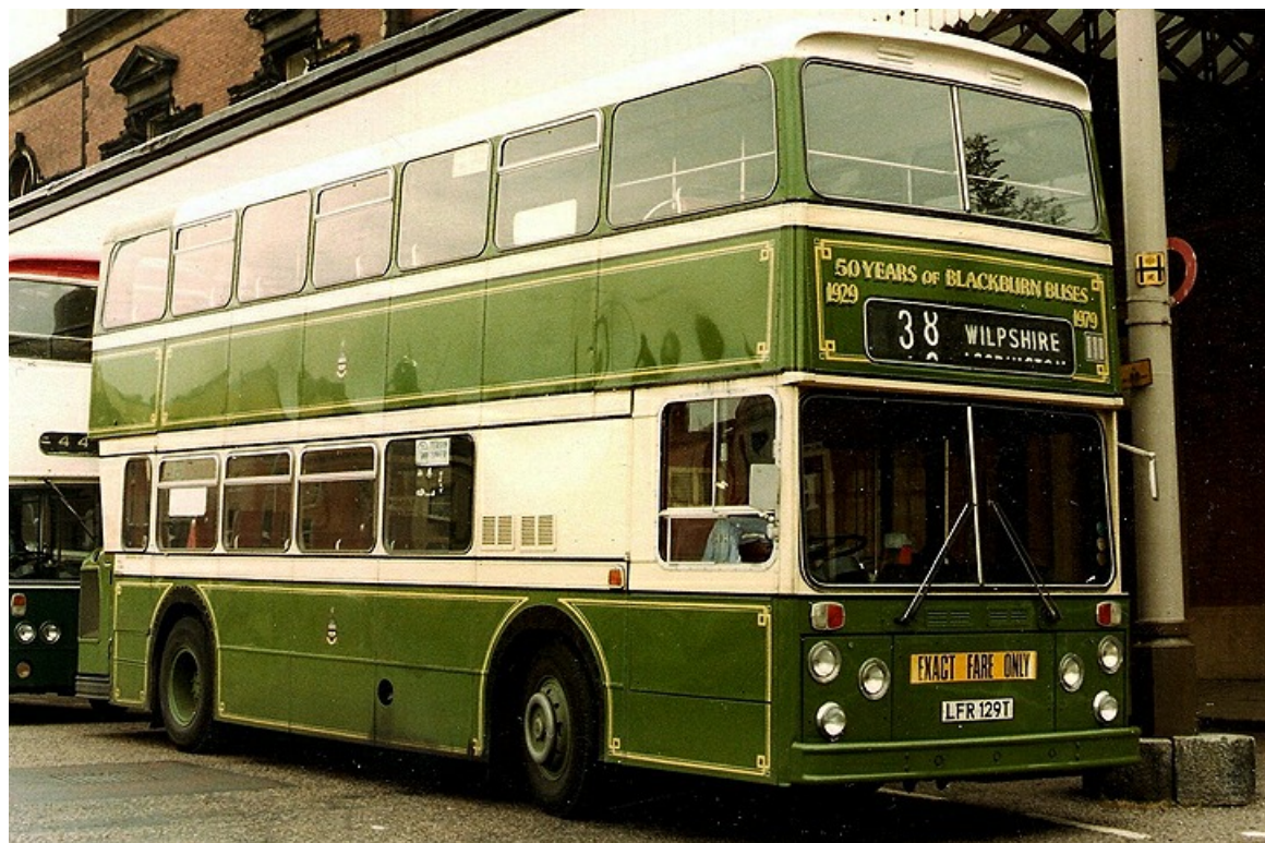
Celebrating 50 years of Blackburn buses in 1979 is No. 129 (LFR129T), a Leyland AN68A/1R with East Lancs H43/31F bodywork new in 1979. (Eddie Leslie).
