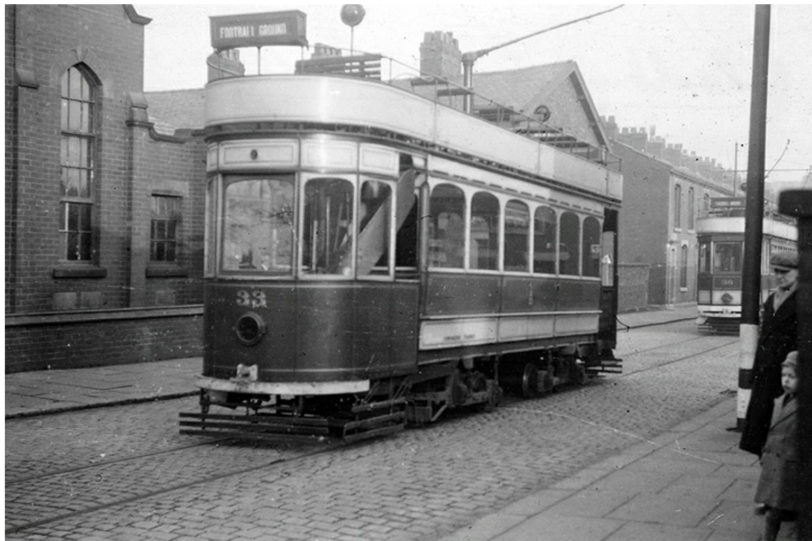
This second photograph of car 33 operating a football special to Ewood Park, shows it as rebuilt with vestibule and extended upper deck. (LTHL collection).
