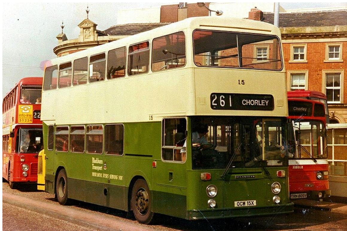
No. 15 (OCW15X) was a Leyland AN68C/1R 'Atlantean' with East Lancashire H43/31F bodywork, which had become standard in the Blackburn fleet by the time of its purchase in 1982. (Eddie Leslie).
