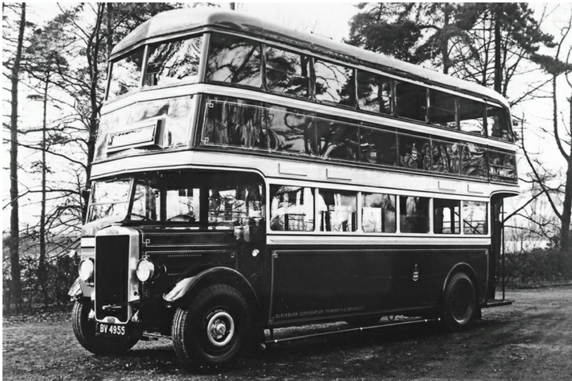
Seen here when new is No. 37 (BV4955) one of three Leyland TD4's purchased in 1935, although this vehicle was the only one with Leyland H30/26R bodywork, the others being bodied by English Electric. (Bus Archive).
