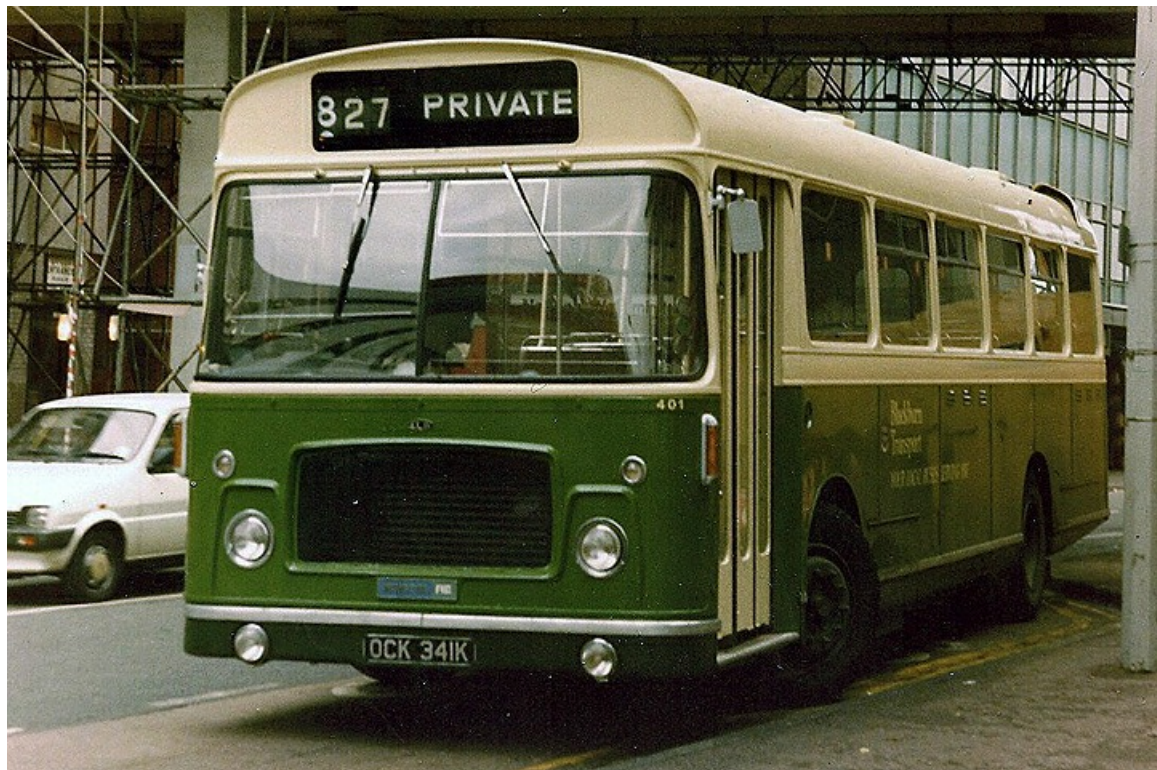
No. 401 (OCK341K) was one of six Bristol RESL6L's with ECW B47F bodywork purchased from Ribble Motor Services in 1986 when already 15 years old. (Eddie Leslie).
