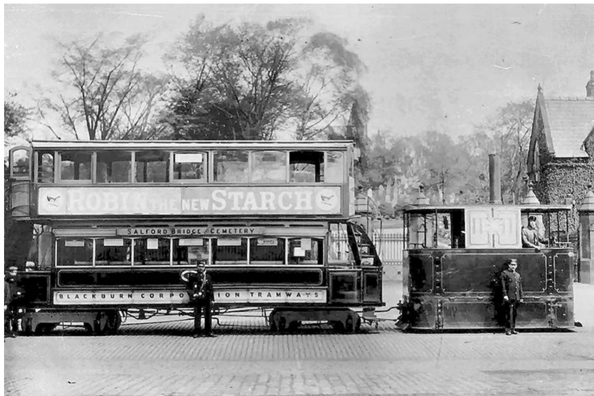
Blackburn Corporation Beyer, Peacock loco 21 ex-North Staffordshire Tramways and Milnes bogie trailer 18 ex-Blackburn & Over Darwen Tramways at the Cemetery terminus c. 1899. (LTHL collection).
