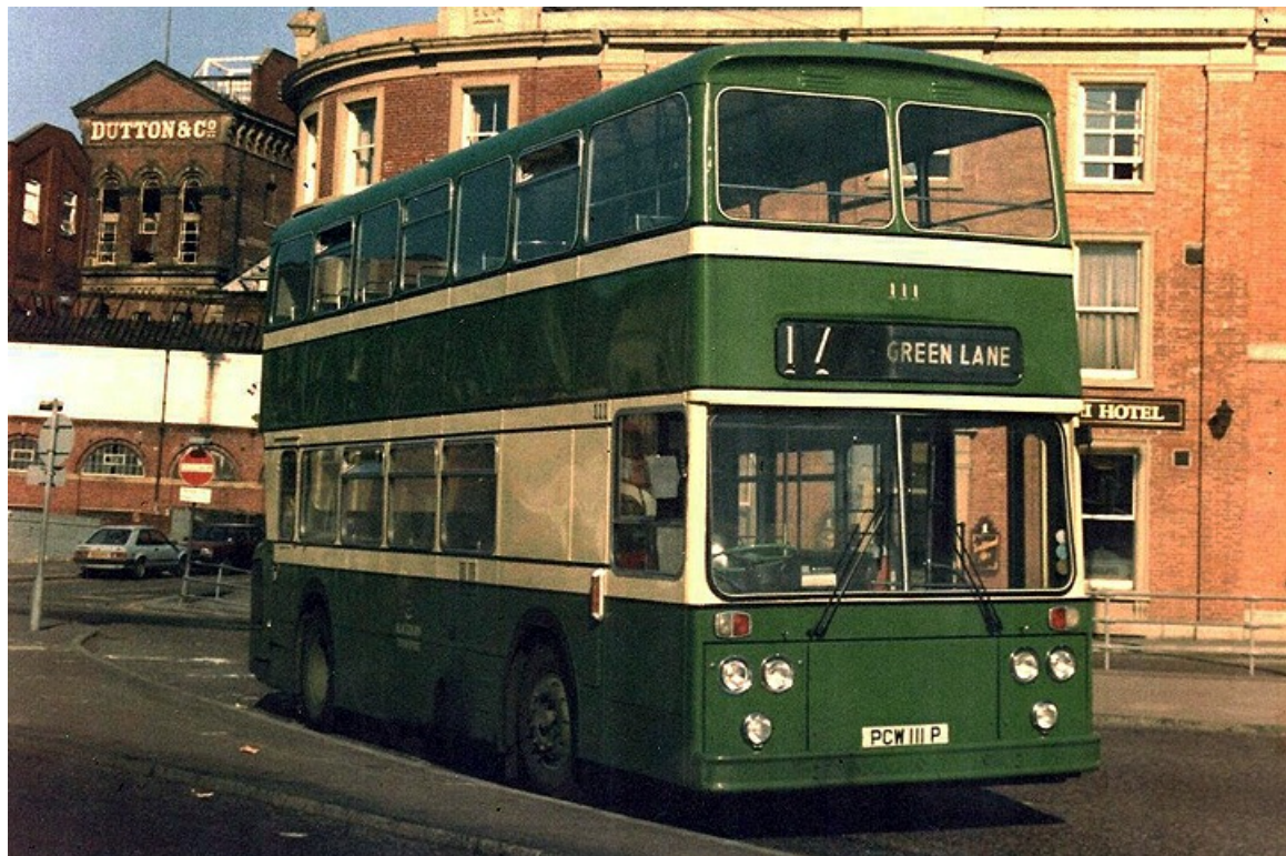
No. 111 (PCW111P) was a 1976 Leyland AN68A/1R 'Atlantean' with East Lancs H45/31R bodywork. (Eddie Leslie).
