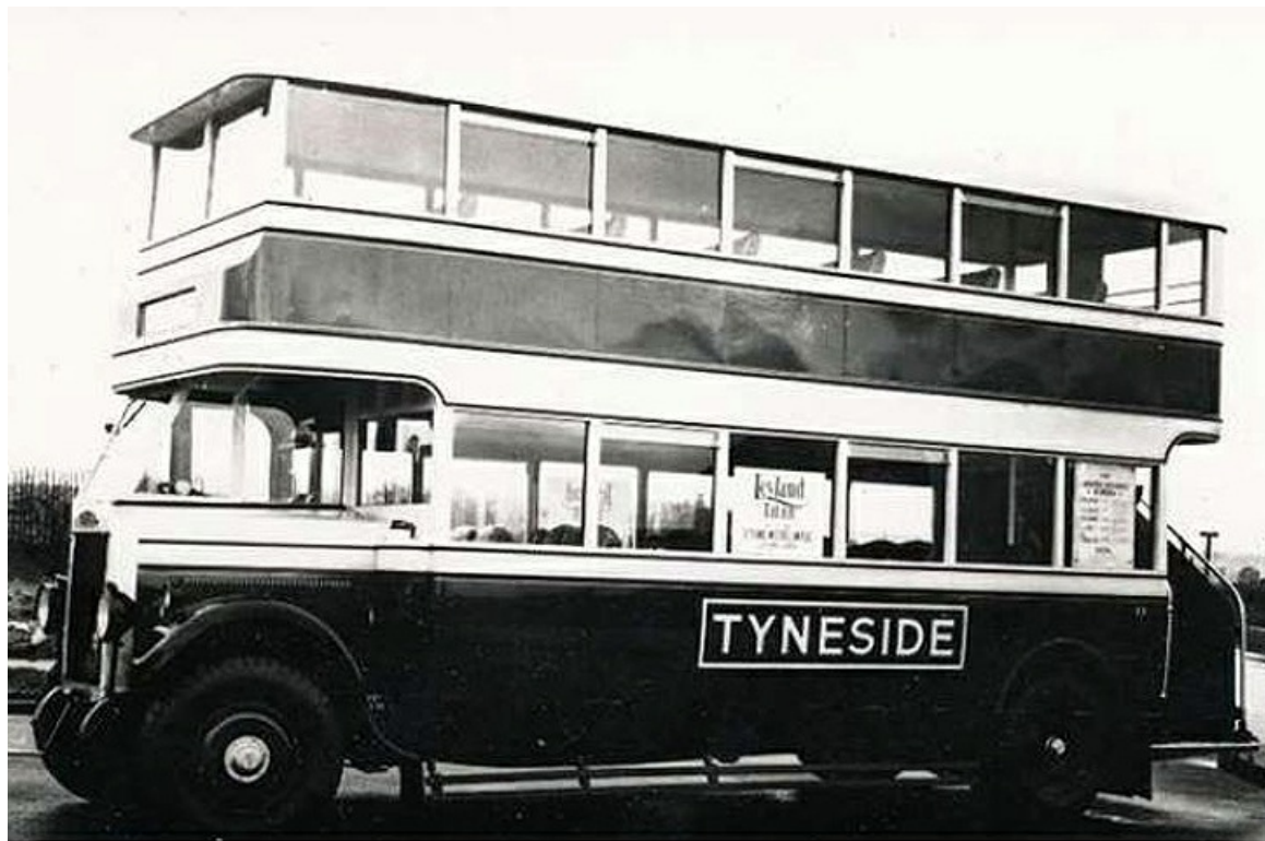
One of the first batch of Leyland TD1's with Leyland 51-seat lowbridge bodywork delivered in 1930. The style of fleetname in an enclosed 'box' lasted until the Second World War when it was dropped. (LTHL collection).
