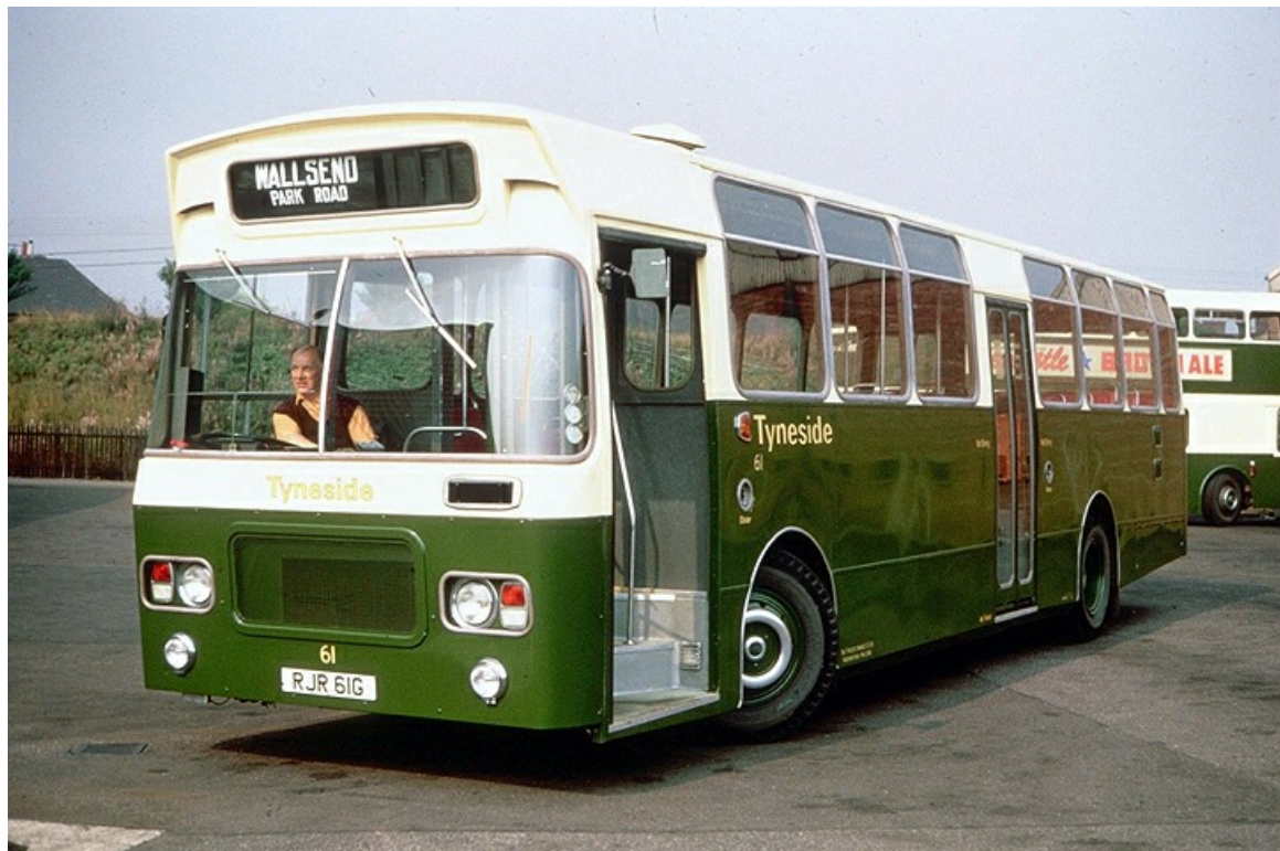
One of only two single-deckers ever to be operated by the Tyneside company was No. 61 (RJR61G) a 1969 Leyland PSUR1A/1R 'Panther' with Marshall dual-entrance 48-seat bodywork. (David Taylor).
