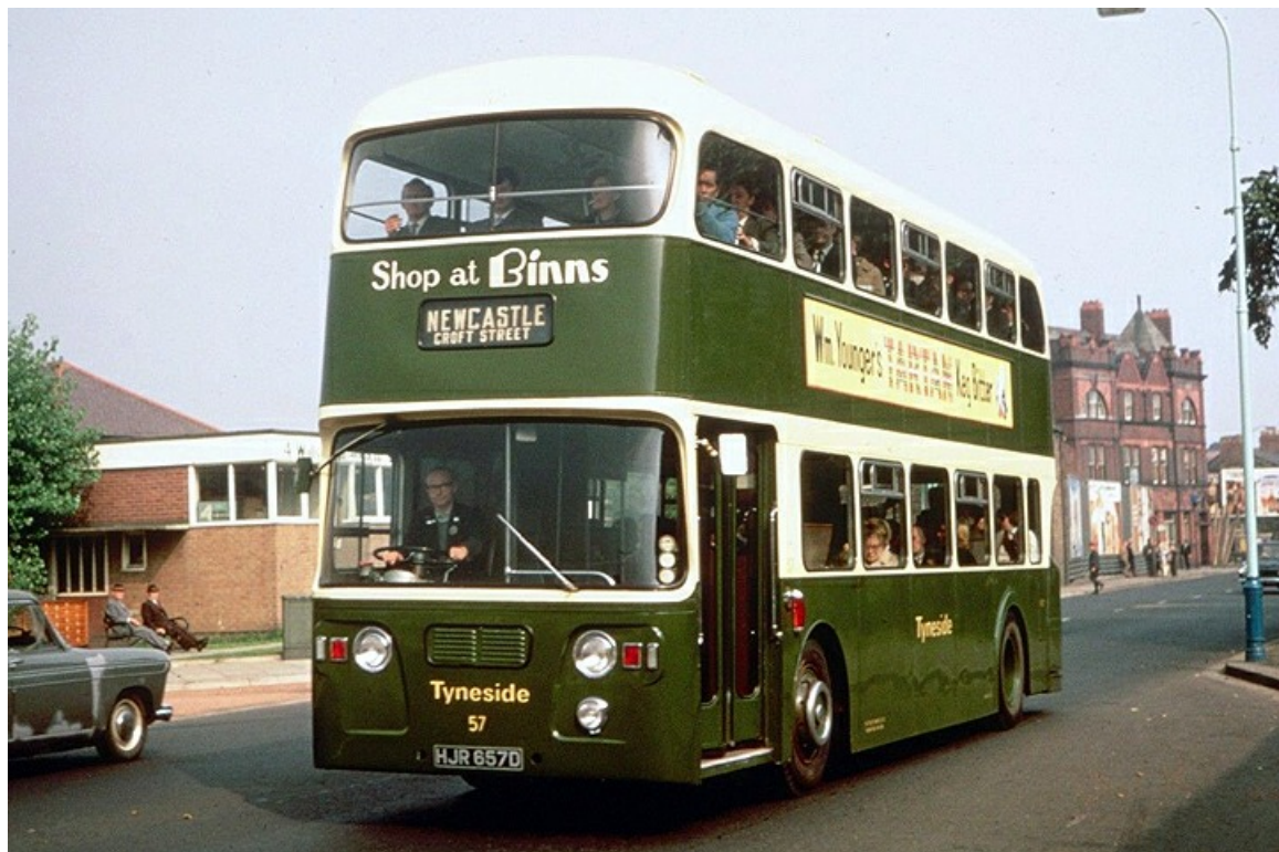
No. 57 (HJR657D) was a 1966 Leyland PDR1/1 with unmistakable Alexander 75-seat bodywork. It became Northern General No. 3324 on 1 January 1976 when the Tyneside fleet was absorbed. (LTHL collection).
