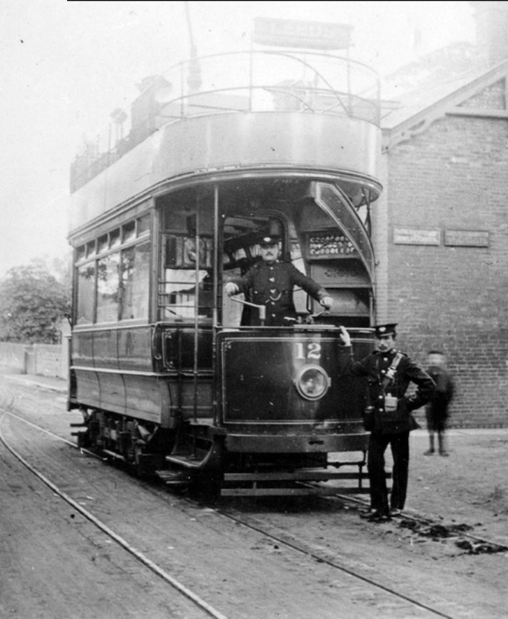
No. 12 was an Electric Railway and Tramway Carriage Works 4-wheel open top double deck car built in 1904 on Brill 21E trucks and seating 56. (LTHL collection).
