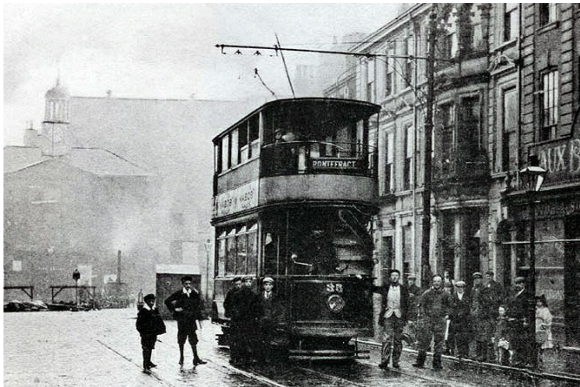
No. 35 was a 1905 top covered car built by the Electric Railway and Tramway Carriage Works of Preston on Brill trucks. It is seen on its way to Pontefract. (LTHL collection).
