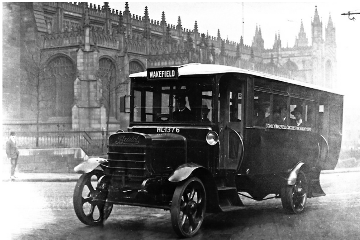
No. 110 (HL1376) a 1922 Bristol 4-ton with Bristol B30D bodywork on its way to Wakefield. (Bus Archive).
