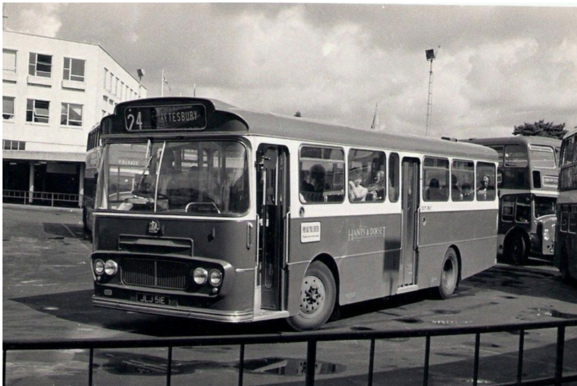
Bedford VAM14 No. 825 (JLJ51E) was new in 1967. It had Strachan 33-seat dual entrance bodywork. It was upseated to 41 in 1968, renumbered 1502 in 1971 and withdrawn the following year. (LTHL collection).
