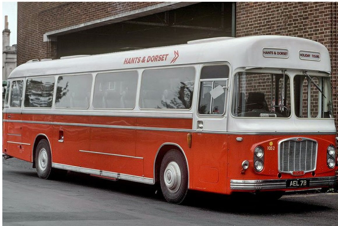
No. 899 (AEL7B) was a 1964 Bristol RELH6G with ECW 47-seat coachwork. It was re-numbered 1052 as seen here in 1971 but was destroyed by fire in 1976. (LTHL collection).
