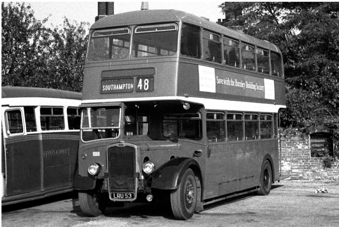
No. 1324 (LRU53), a 1952 Bristol KSW6G with ECW 60-seat bodywork. It was renumbered 1387 in 1971 and withdrawn in 1972. (LTHL collection).
