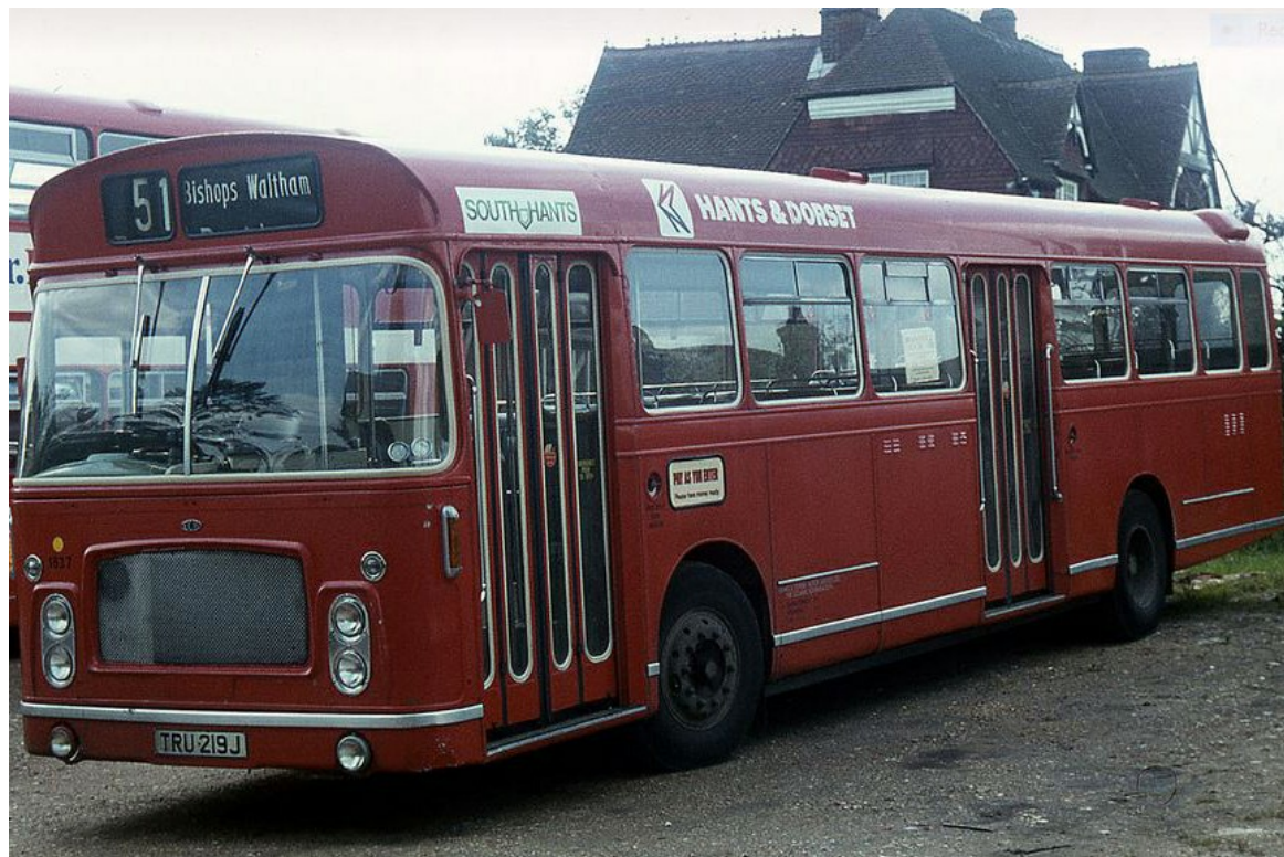
No. 3041 (TRU219J) was a 1970 Bristol RELL6G with ECW 45-seat dual entrance bodywork. It was renumbered 1637 in 1971 and passed to Hampshire Bus in 1983 on the demise of Hants & Dorset. (John Law).
