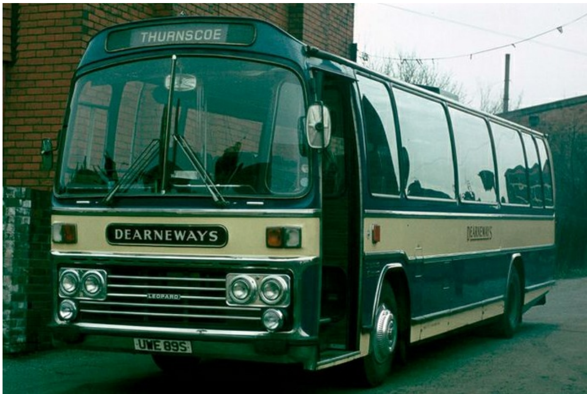
No. 89 (UWE89S) was a 1976 Leyland PSU3E/4R Leopard with Plaxton 51-seat coachwork. (Richard Simons).
