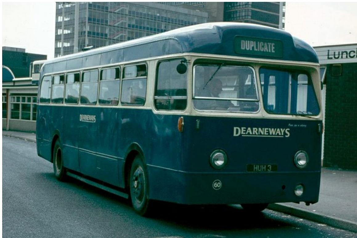
No. 60 (HUH3) was a 1953 Leyland PSUC1/1 with Weymann 44-seat bodywork that was formerly No. 1003 in the Western Welsh fleet and was acquired in 1966. It was withdrawn in 1974. (Richard Simons).
