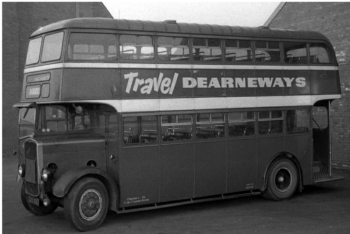
No. 19 (ERU600) was a 1939 Bristol K5G with ECW 53-seat lowbridge bodywork that was acquired from Hants & Dorset Motor Services in 1960. It was withdrawn in 1962. (John Law).
