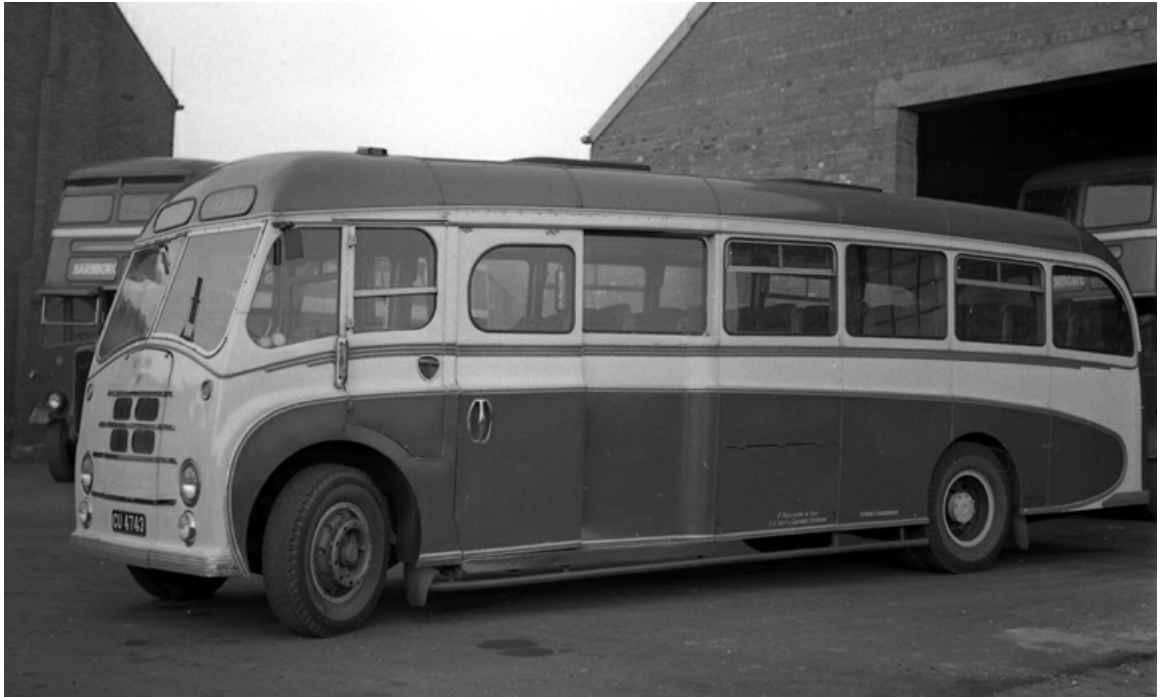
Acquired in 1959 was No. 10 (CU4743), a 1947 Leyland PS1/1/ with Burlingham 33-seat full-front coachwork that was new to Hall Brothers of South Shields. Seen here at the depot, it was withdrawn in 1961. (John Law).
