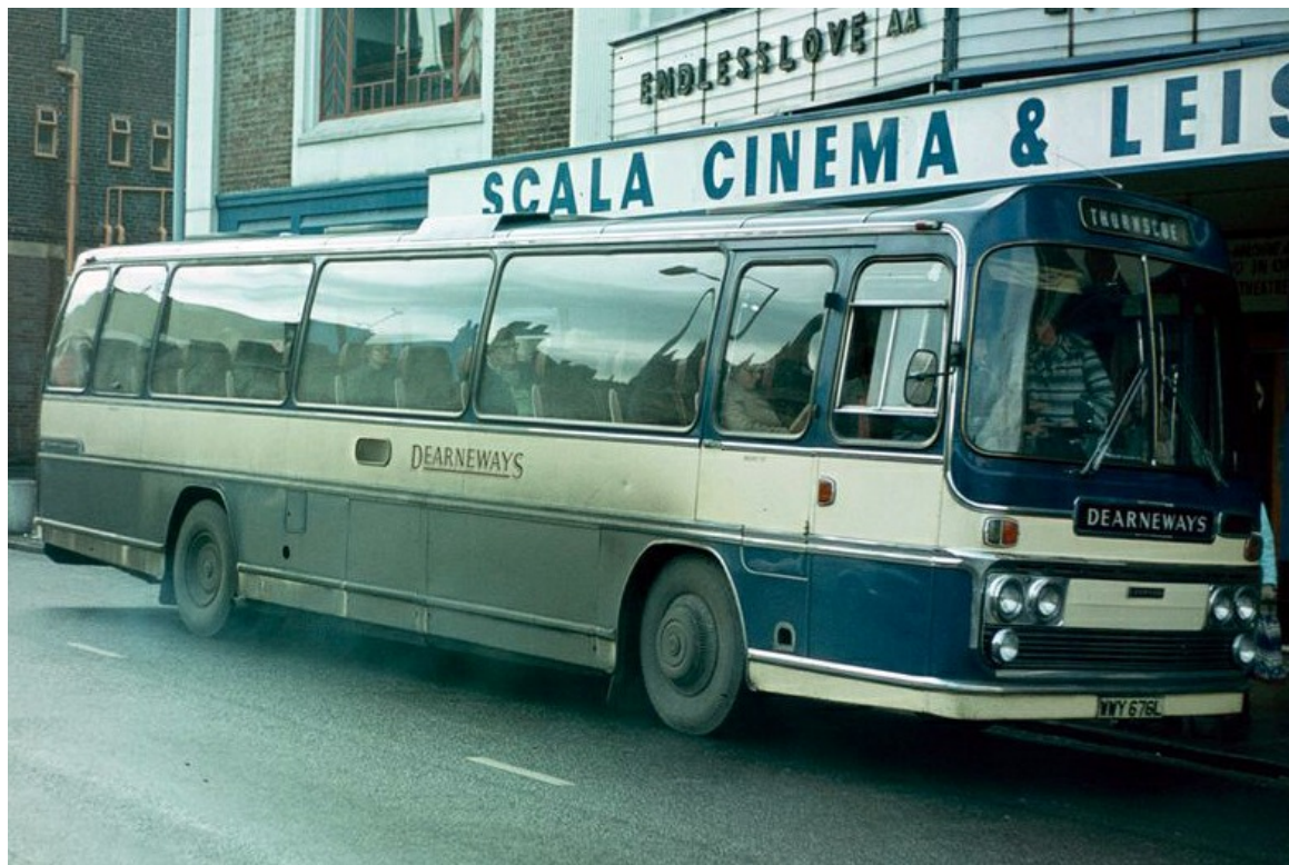
No. 76 (WY676L), new in 1973. was a Plaxton bodied 51-seat Leyland Leopard PSU3B/4R. (Richard Simons).
