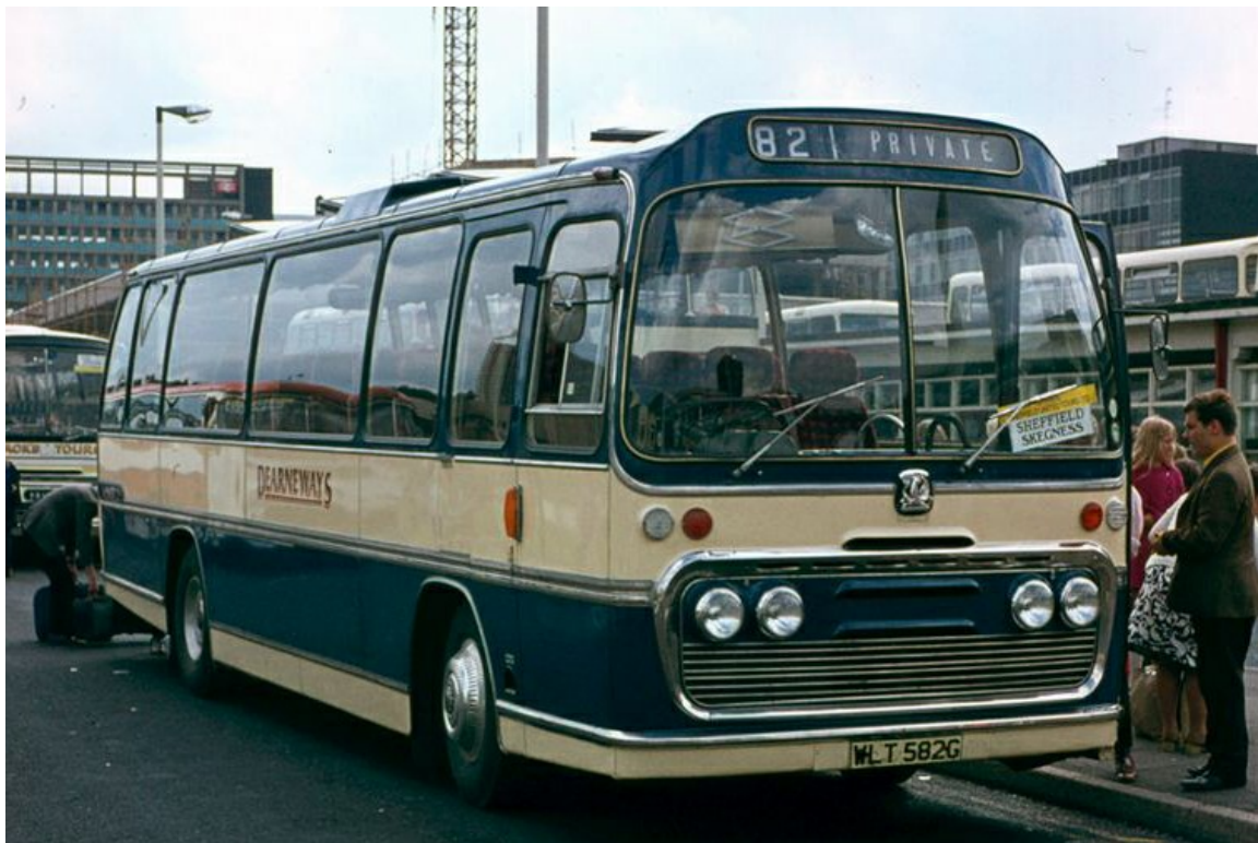
In 1974 Dearneways acquired four ex-Grey Green Bedford VAM70 coaches with Plaxton 45-seat coachwork. This is No. 82 (WLT582G), which had been new in 1969. (Richard Simons).
