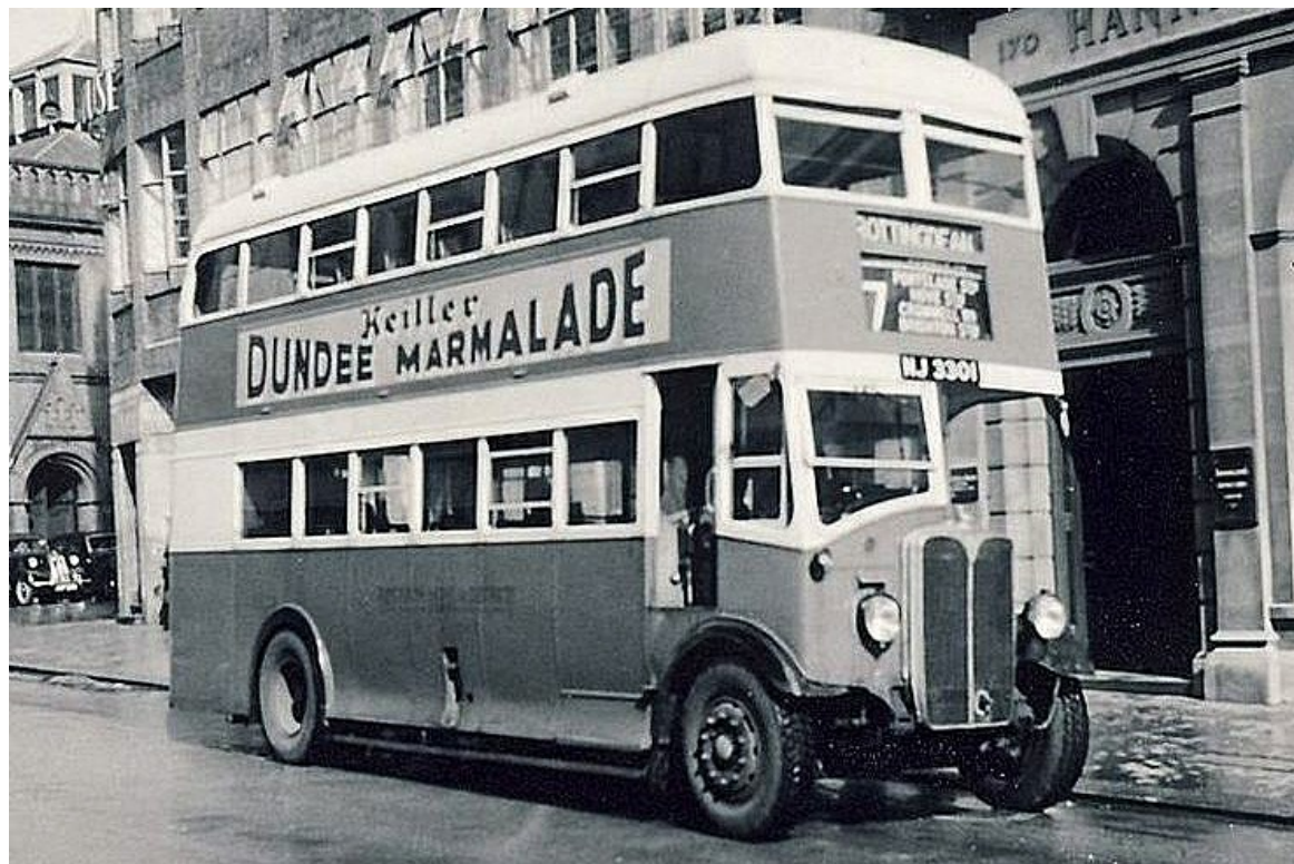
No. 6301 (NJ3301) was another AEC Regent with Tilling 56-seat bodywork that was rebuilt as shown by Beadle in 1946. It was withdrawn in 1955. (Wimborne Railway Society Archive).
