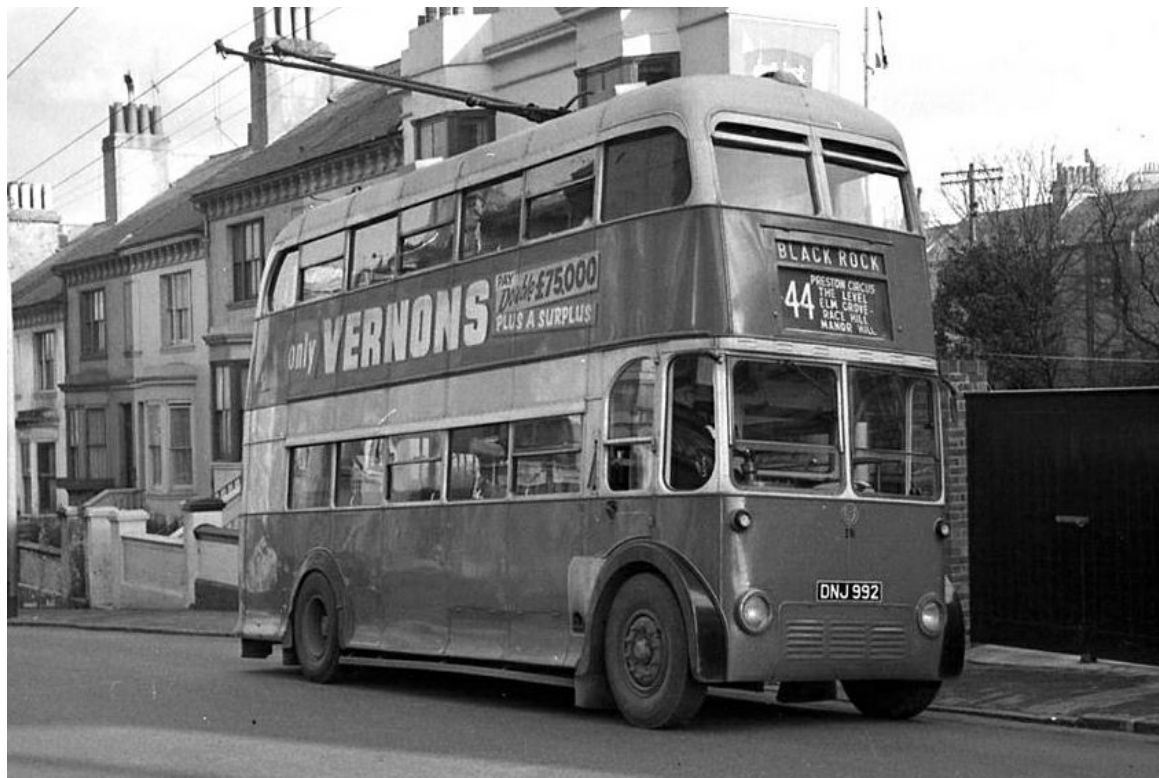
No. 391 (DNJ992) was one of three 1948 BUT9611T's with Weymann 56-seat bodywork delivered in 1948. (John Boylett courtesy John Kaye).
