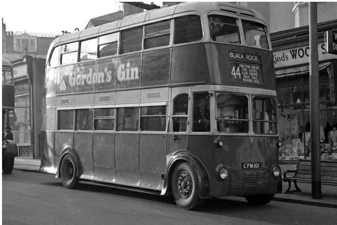
No. 344 (CPM101) was a 1945 AEC 661T with Weymann 54-seat bodywork seen here in Chatham Place, New England Road, Brighton in January 1959. (John Boylett courtesy John Kaye).
