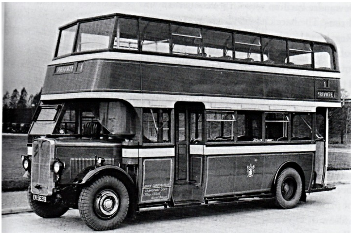
No. 46 (EN5639) was an AEC Regent with Roe dual door H24/24D bodywork, again with the unusual twin staircases, one projecting over the bonnet. (LTHL collection).
