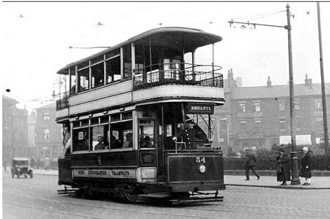
No. 54, seen here passing through Kay Gardens en route to Radcliffe, was built in 1913 by the United Electric Car Company of Preston on Mountain & Gibson trucks. (LTHL collection).
