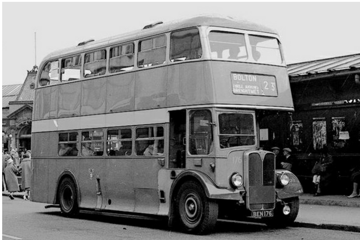
No. 176 (BEN176) was an AEC Regent III with Weymann 56-seat bodywork one of a pair that joined the fleet in 1952. (Mike Beamish).
