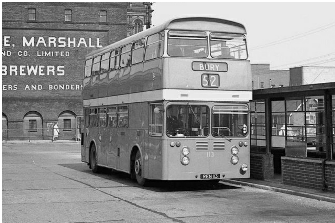
No. 113 (REN113) was a 1963 Leyland PDR1/1 with MCW 74-seat Liverpool-style bodywork. (Mike Beamish).
