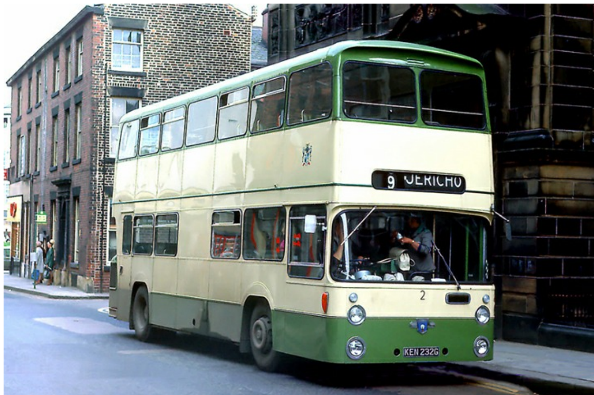
No. 2 (KEN232G) was among the final deliveries to Bury Corporation in 1969 before it was absorbed into SELNEC PTE. It was a Leyland PDR1/1 with East Lancs dual door 72-seat bodywork. (Alan Snatt).
