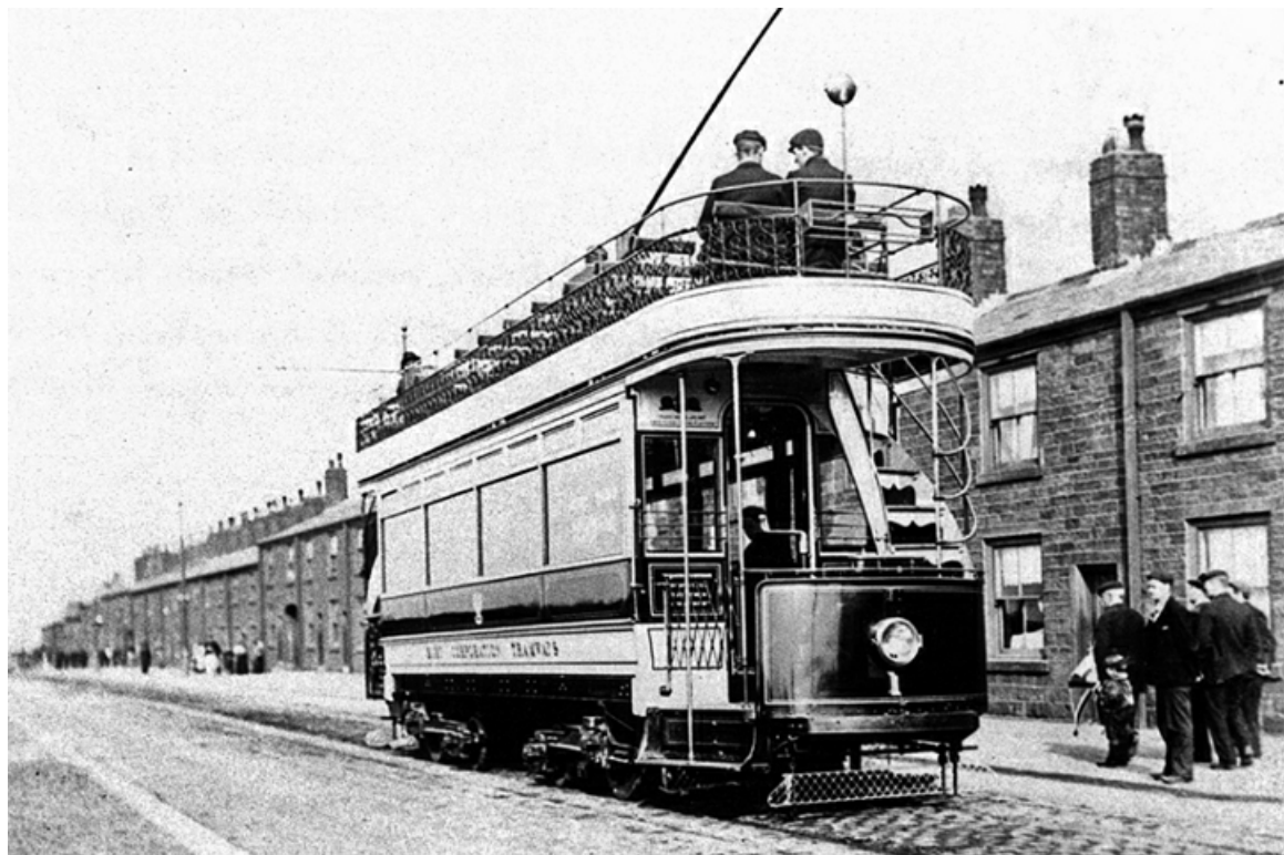
Bury car No. 1 was a 1903 Milnes-built bogie car on McGuire No. 3 trucks and seating 73. It is seen here on Rochdale Old Road c. 1903 and in original condition. (LTHL collection).
