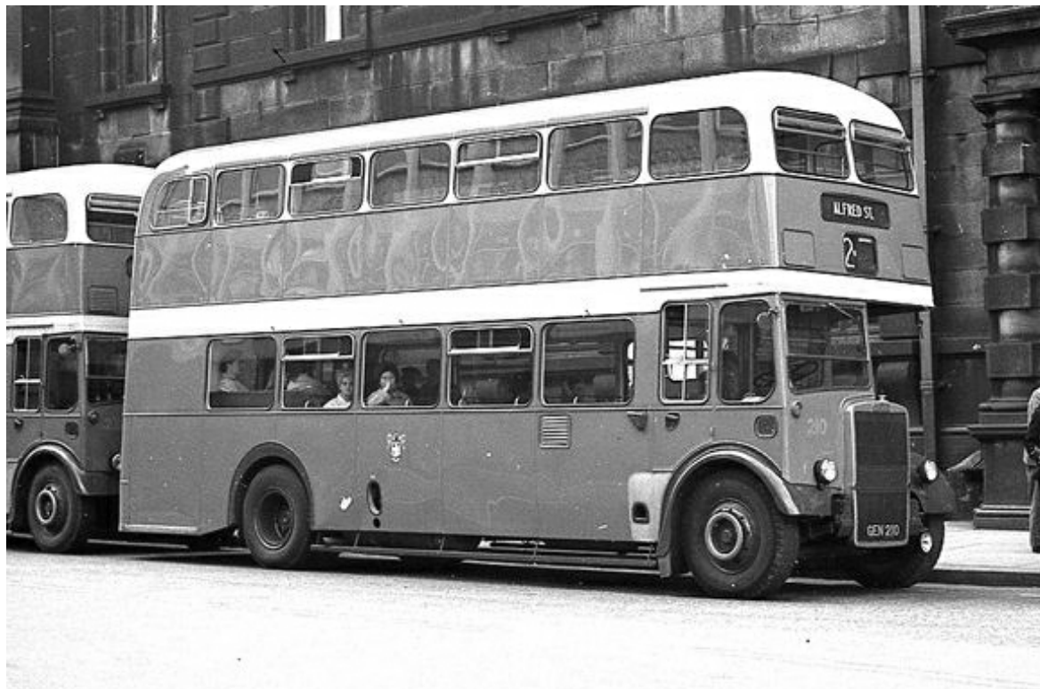
No. 210 (GEN210) was a 1958 Leyland PD3/6 with attractive Weymann 73-seat bodywork. It passed to SELNEC PTE in 1969 as their No. 6360. (Mike Beamish).
