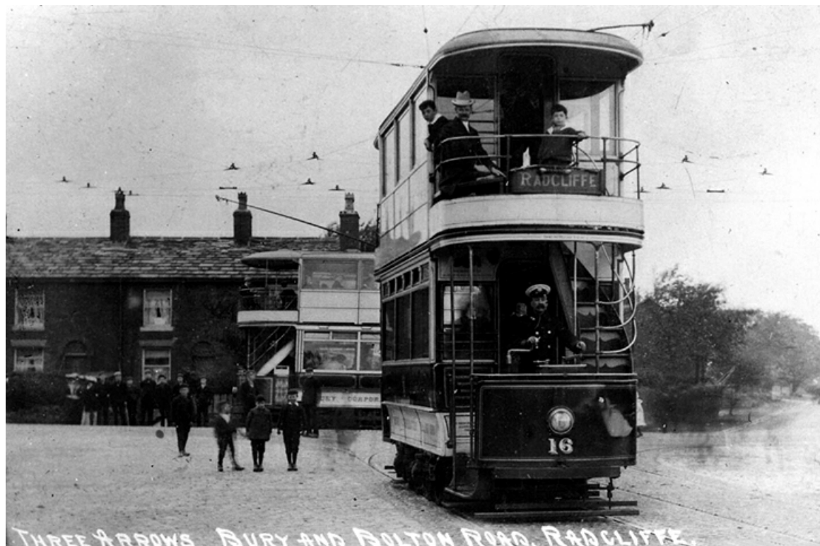
Car No. 16 at the Three Arrows. It was a 1903 Milnes-built 4-wheel car seating 56 and is seen here with its balcony top-cover that was fitted c. 1905. (LTHL collection).
