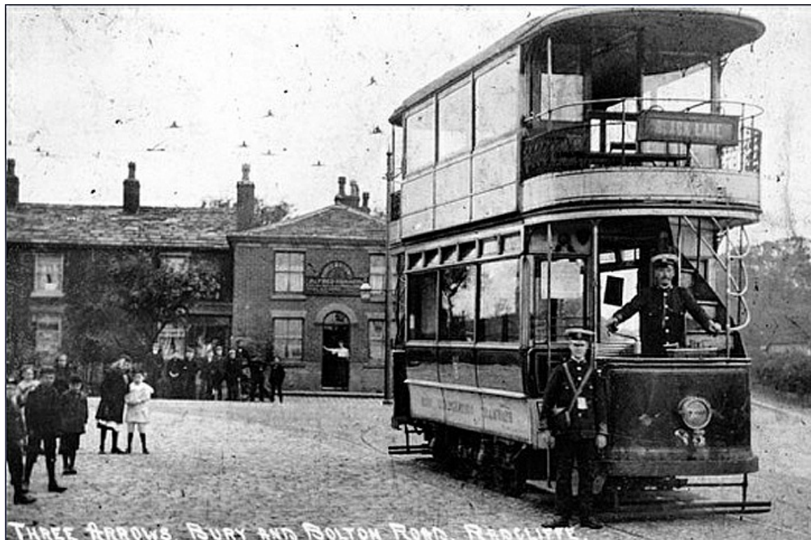
Car No. 35 was a built in 1905 by the local firm of Wilson & Stockall on Mountain & Gibson trucks and seated 56-seat. It was top-covered from new. (LTHL collection).
