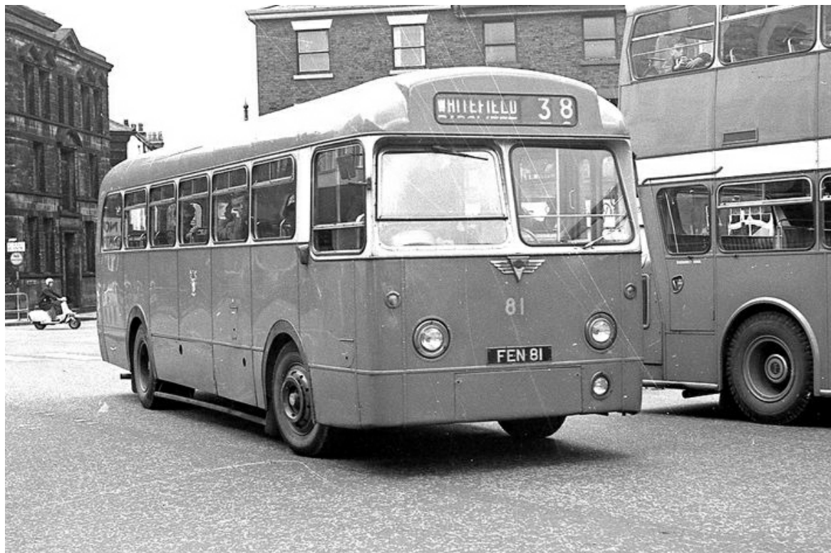
Bury purchased 6 of these AEC Reliance with Weymann 43-seat bodywork in 1957. This is No. 81 (FEN81) the first of the batch. (Mike Beamish).
