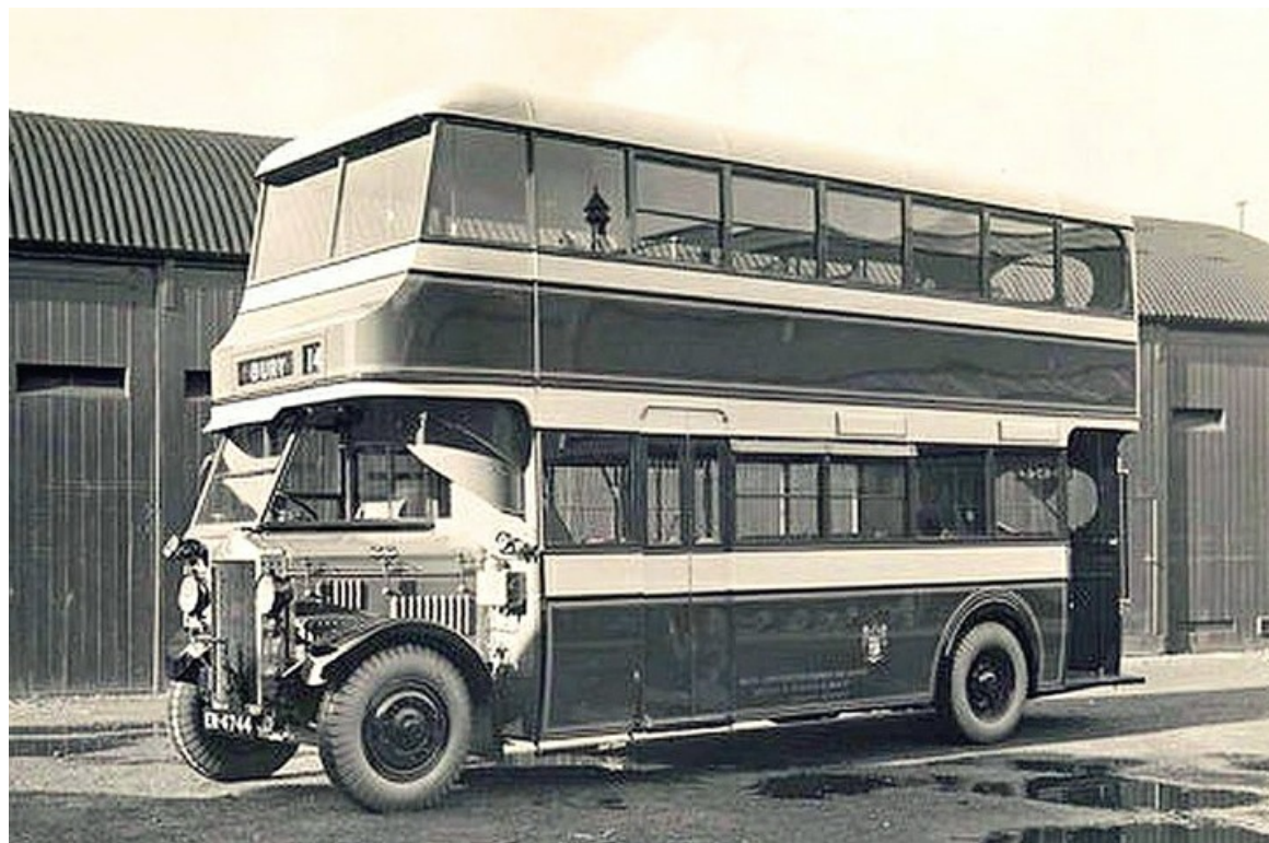
No. 28 (EN4744) was a 1930 Crossley VR6 with Brush 48-seat dual door bodywork and unusual twin staircases. (LTHL collection).
