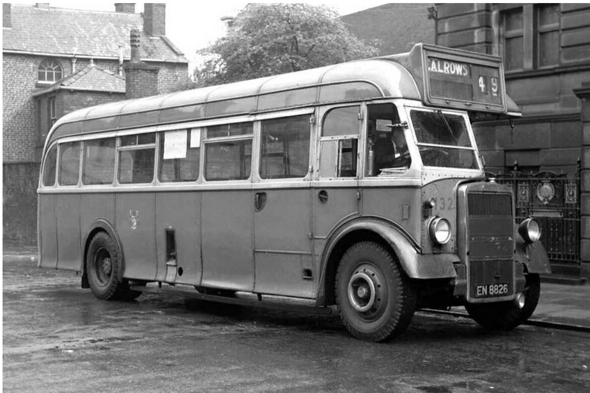
No. 132 (EN8826) was 1947 Leyland PS1 with Roe 35-seat bodywork converted to forward entrance by Northern Counties in 1954 as shown here. (John Kaye).
