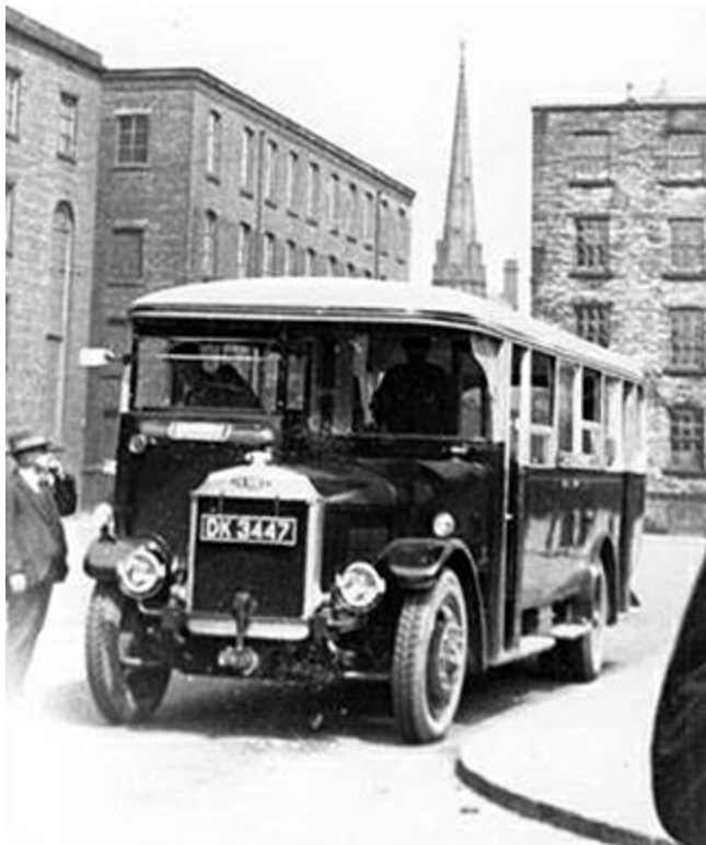
One of Rochdale Corporation's initial intake of buses in 1926 was No. 5 (DK3447) a Dennis E with Strachan & Brown 30-seat dual-entrance bodywork. (LTHL collection).
