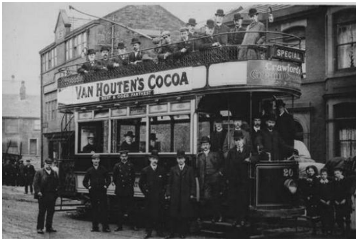
No. 20 at Smallbridge in 1905, was a 1905 Brush-built 4-wheel car. It survived almost to the end of the system, being withdrawn in 1932. (LTHL collection).
