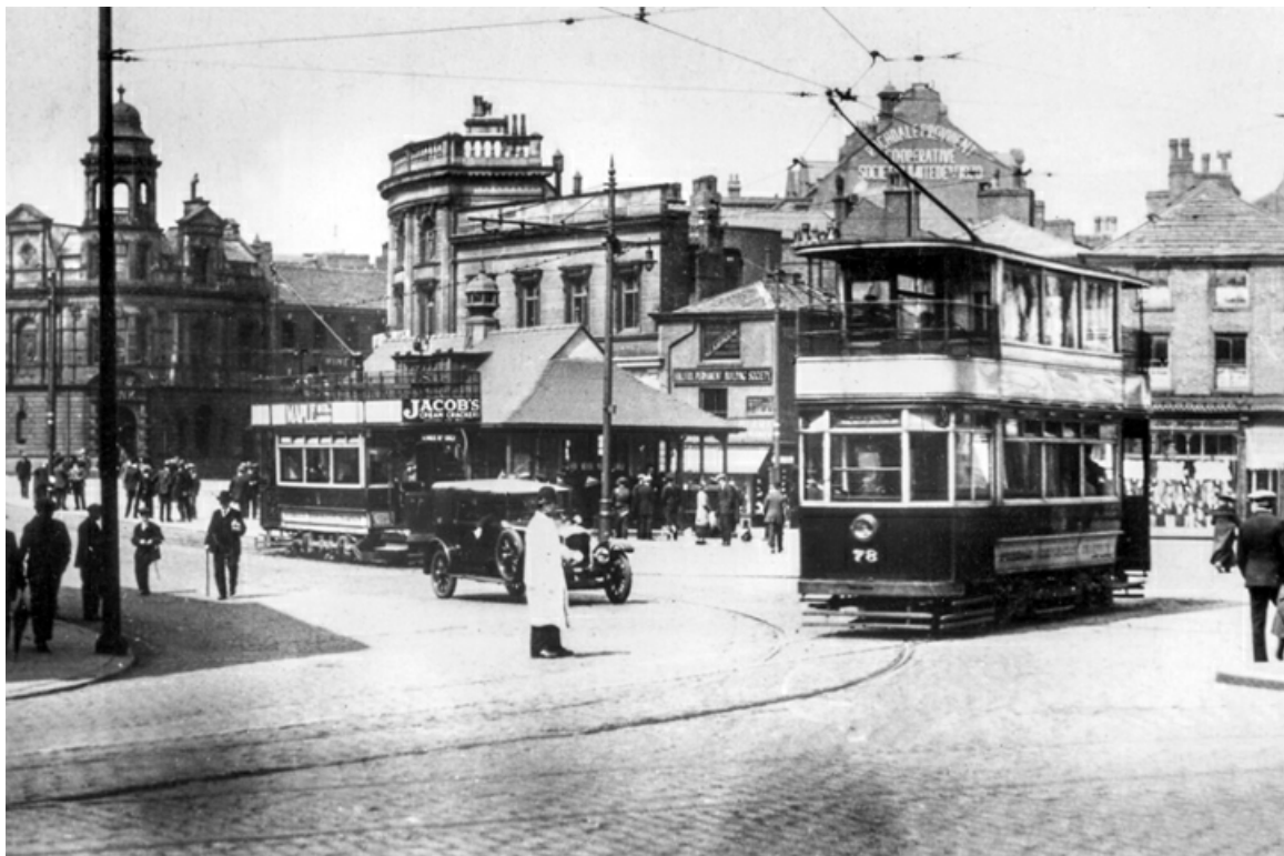
Car No. 78, a 4-wheel double-decker built in 1920 by English Electric on Brill 21E trucks and seating 48 exits Drake Street watched by a white-coated policeman on traffic duty, a long gone sight. (LTHL collection).
