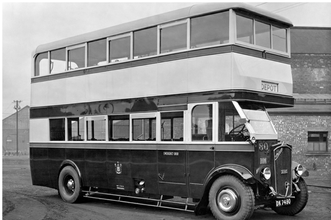
1931 Dennis Lance No. 80 (DK7490) with English Electric 52-seat bodywork. (GEC collection courtesy David Beilby).
