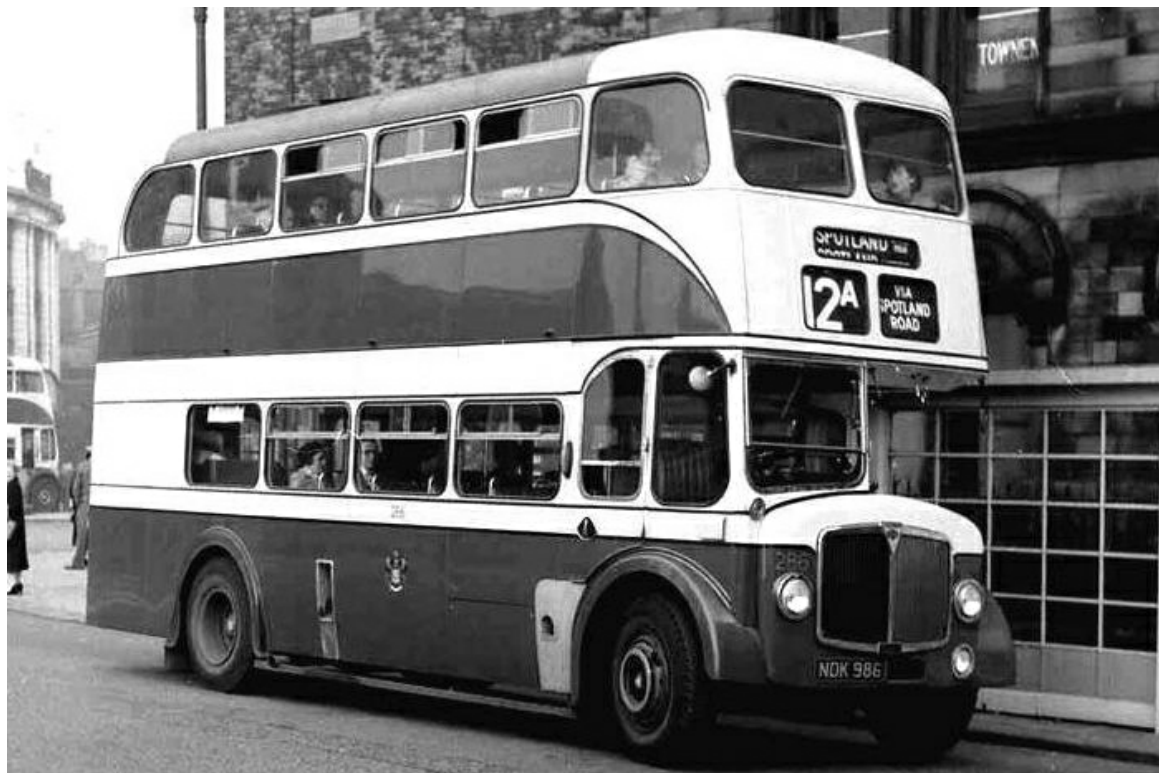
No. 286 (NDK986) was a 1956 AEC Regent V with Gardner 6LW engine, pre-selector gearbox and sporting a Weymann 61-seat body. (John Kaye).
