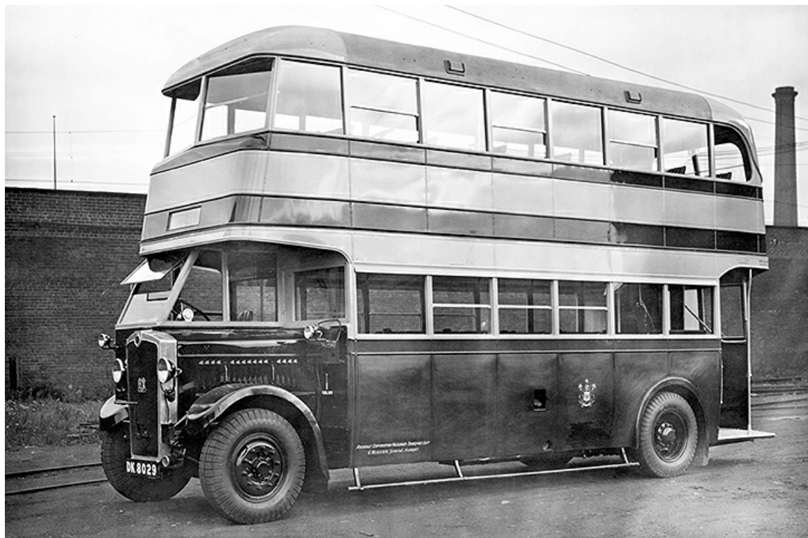
Crossley Condor No. 114 (DK8029) with English Electric 52-seat bodywork. It was withdrawn at the end of 1945. (GEC collection courtesy David Beilby).
