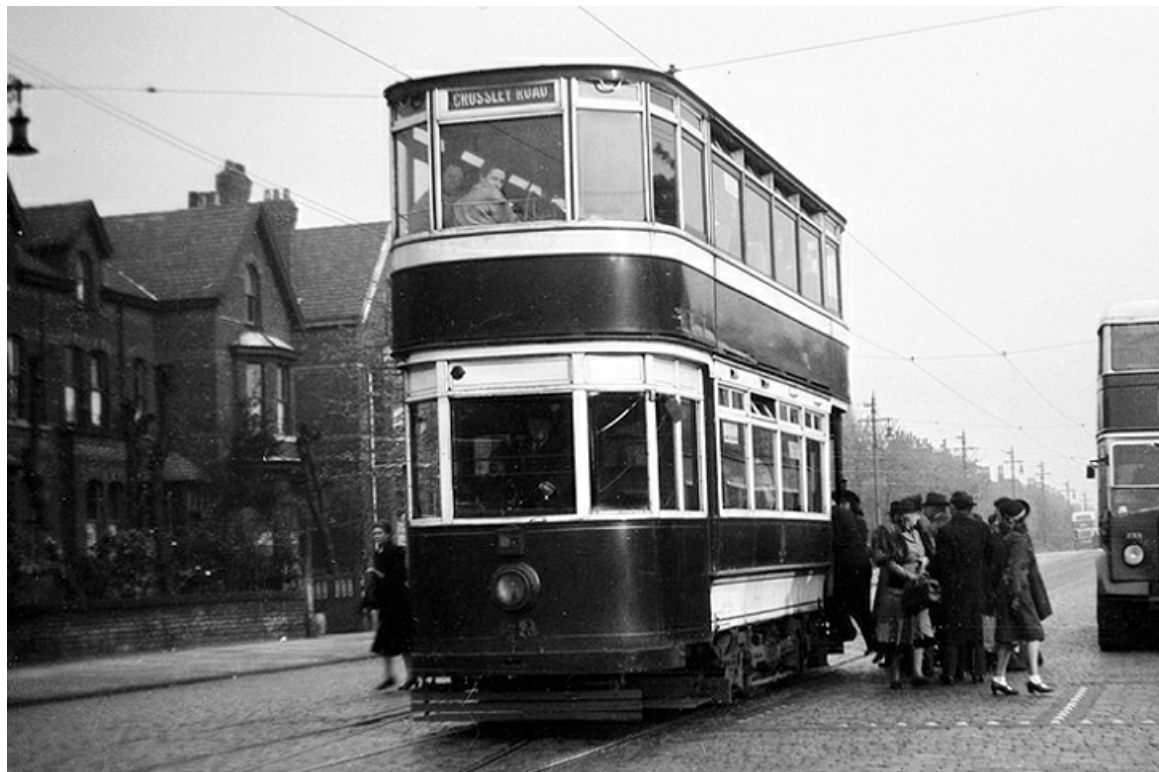
No. 69 was a fully-enclosed 4-wheel car seating 56, built by Cravens on Cravens trucks and dating from 1923. (LTHL collection).
