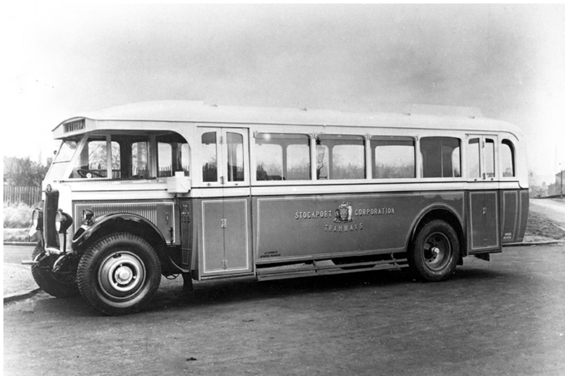
No. 165 (JA1465) a 1930 Leyland TS3 with Leyland B30D bodywork, one of six purchased that year. (Bus Archive).
