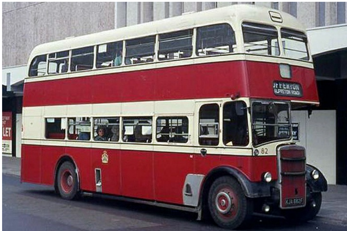
No. 82 (KJA882F) was a 1968 PD3/14 with East Lancs 70-seat bodywork. It became SELNEC PTE's No. 5882 in 1969. (John Kaye).
