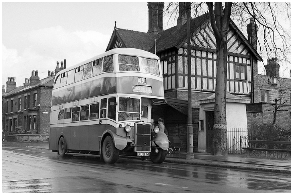
No. 242 (CDB12) was a 1947 Crossley DD42/3 with Crossley's distinctive H30/26R bodywork. (Bus Archive).
