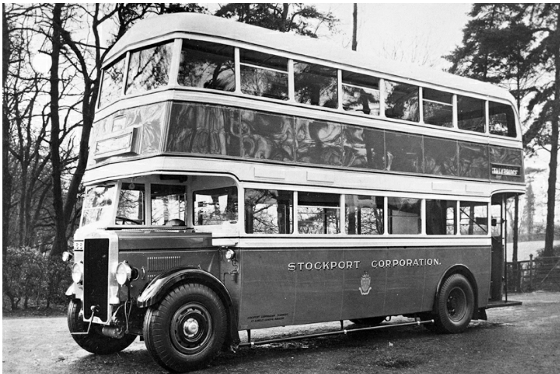
1934 Leyland TD3 No. 166 (JA5443) with Leyland 52-seat bodywork, which survived in service until 1958 before withdrawal. (Bus Archive).
