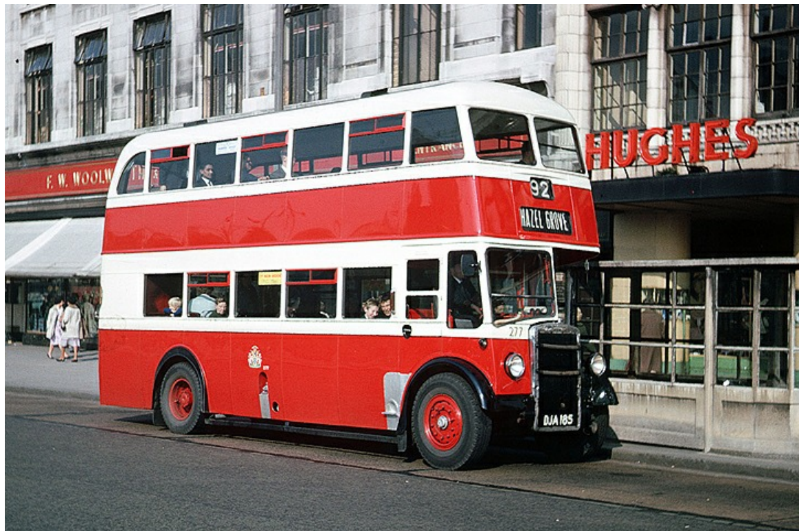
Looking as though it has come straight out of the paintshop is No. 277 (DJA185), a Leyland PD2/1 with Leyland H30/26R bodywork dating from 1949. (Bus Archive).
