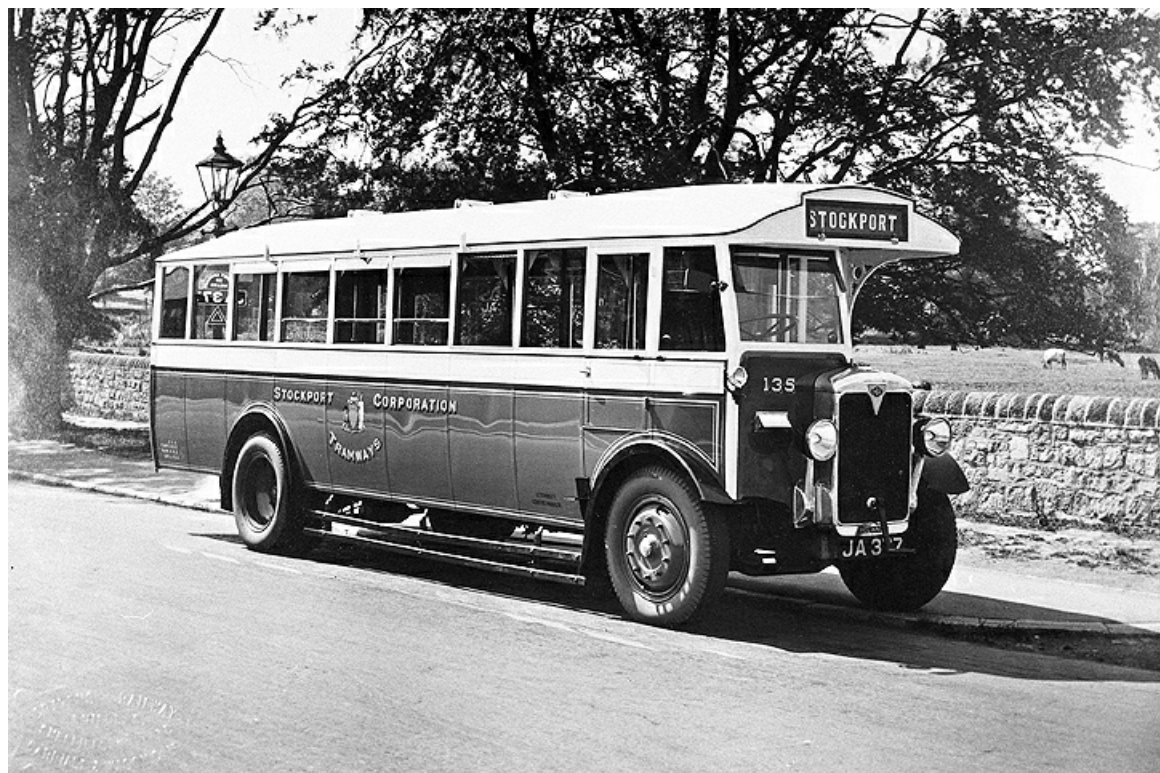
No. 135 (JA377), one of 12 Cravens B32D bodied AEC Reliance chassis purchased in 1929. (Bus Archive).
