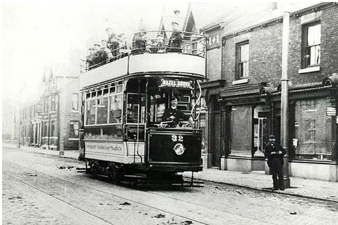
No. 32 was a 1905 Brush-built 4-wheel car that was top-covered two years later. It was withdrawn just a year before the demise of the system in 1951. (LTHL collection).
