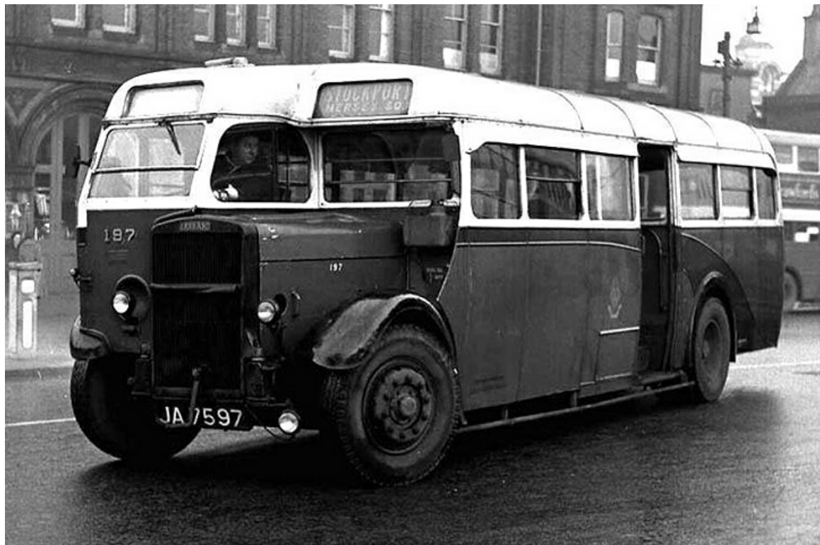
No. 197 (JA7597) was a 1937 Leyland TS8 with 35-seat English Electric bodywork seen in Mersey Square in February 1958. (John Kaye).
