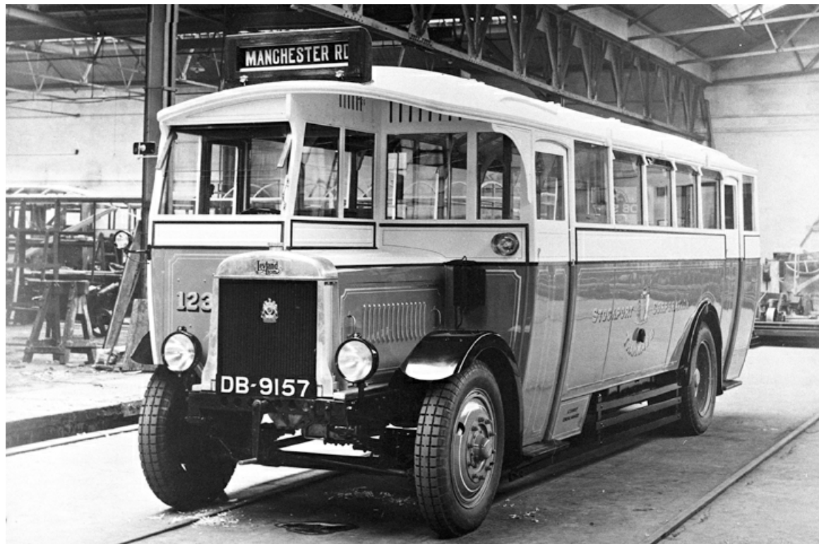
No. 123 (DB9157) was a 1928 Leyland PLSC1 'Lion' with Cravens B32D bodywork, which was rebuilt to B34R at a later date. (Bus Archive).
