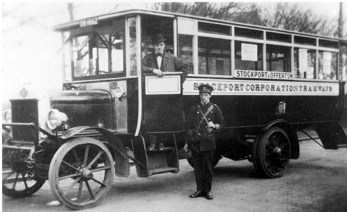
No. 101 (DB1662) a 1919 AEC YC with British Commercial 30-seat rear entrance bodywork one of three purchased to replace the troublesome trolleybuses. (Bus Archive).
