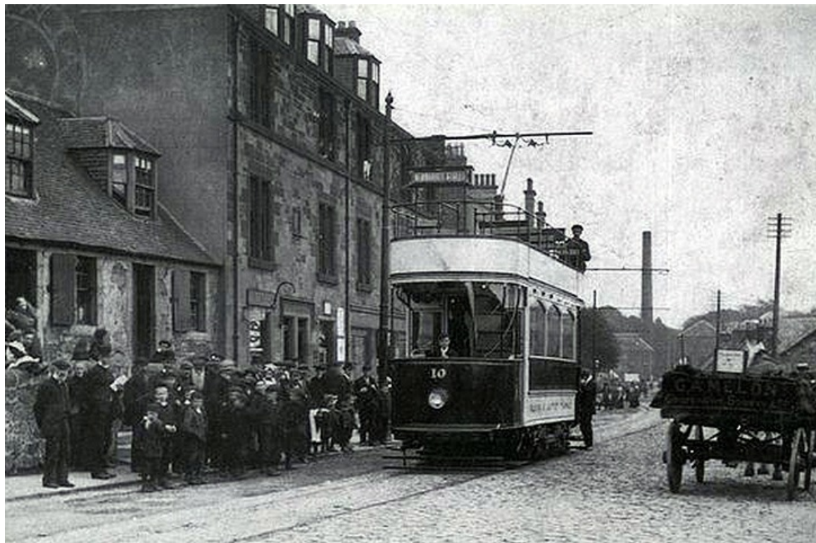
One of the original 1905 cars was No. 10, built by the French firm of Compagnie Générale de Construction of Paris and shipped to Scotland, seen here at Camelon Bridge. This tramcar was replaced in 1921 by a new single-deck saloon car which took its number. (LTHL collection).
