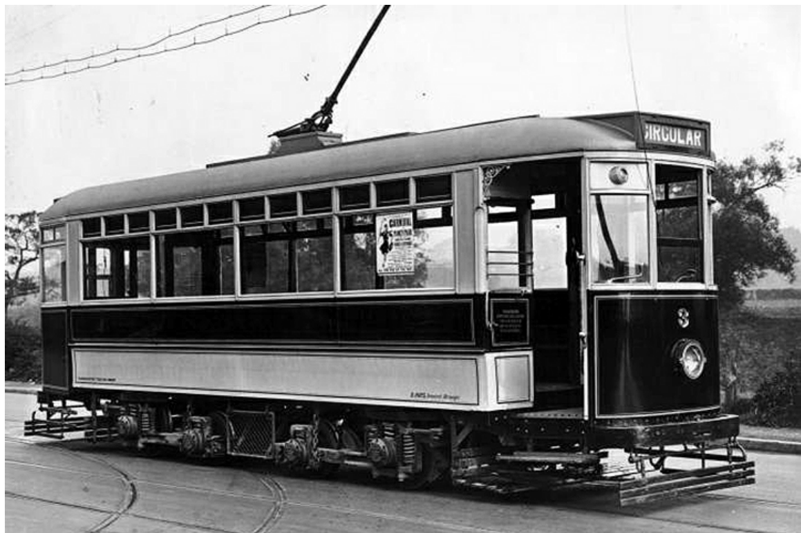
No. 3 was one of ten Brush-built single-deck saloon cars purchased in 1921 to replace the double-deckers. They afforded much better protection from the inclement Scottish weather. (LTHL collection).
