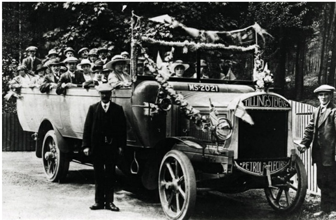
MS2021 was new in 1919 to Falkirk & District Tramways and is seen here decorated for an unknown occasion. Numbered 10 it was a Tilling-Stevens TS3 probably with Tilling bodywork. (LTHL collection).
