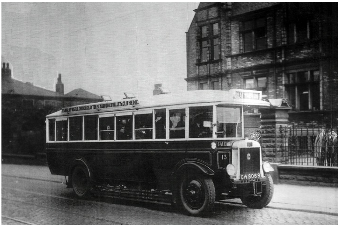
The Calder Motor Company was taken over in September 1929 and included this vehicle. No. 13 (CW8069) was a 1928 Leyland LSC1 with Leyland B31R bodywork; it retained its number with Rishton & Antley and passed to Ribble MS in 1930 as their No. 1004. (LTHL collection).
