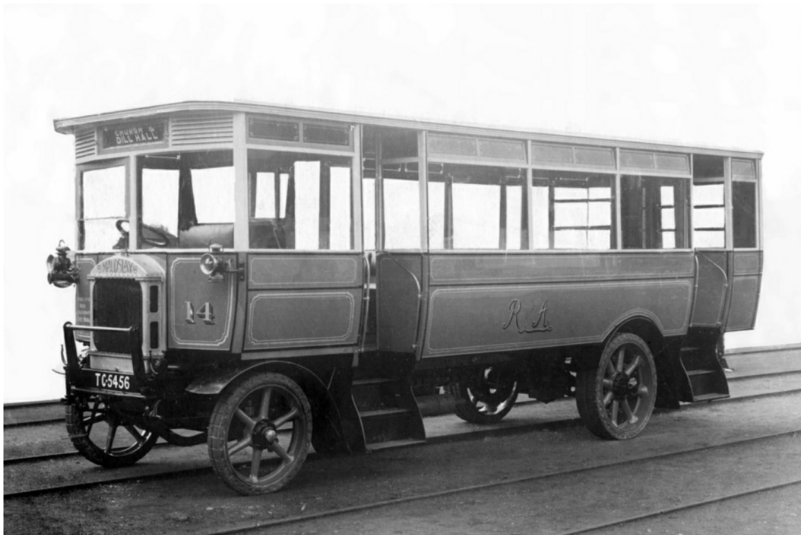
No. 14 (TC5456) a 1923 Maudslay CP originally with a charabanc body is seen here in an official English Electric photo sporting its new FB32D body. (GEC collection courtesy David Beilby).
