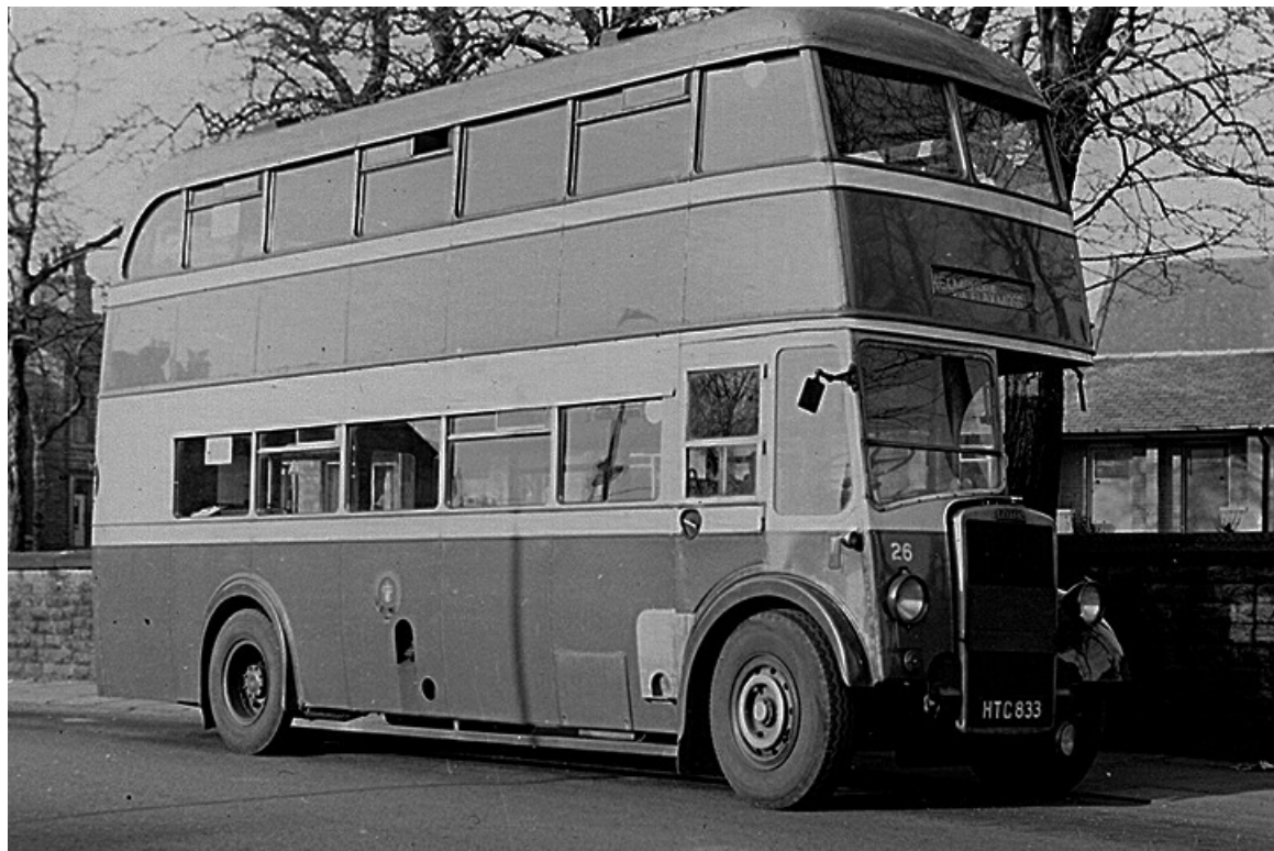
No. 26 (HTC833) was a 1947 Leyland PD1A with Leyland H30/26R bodywork. (LTHL collection).
