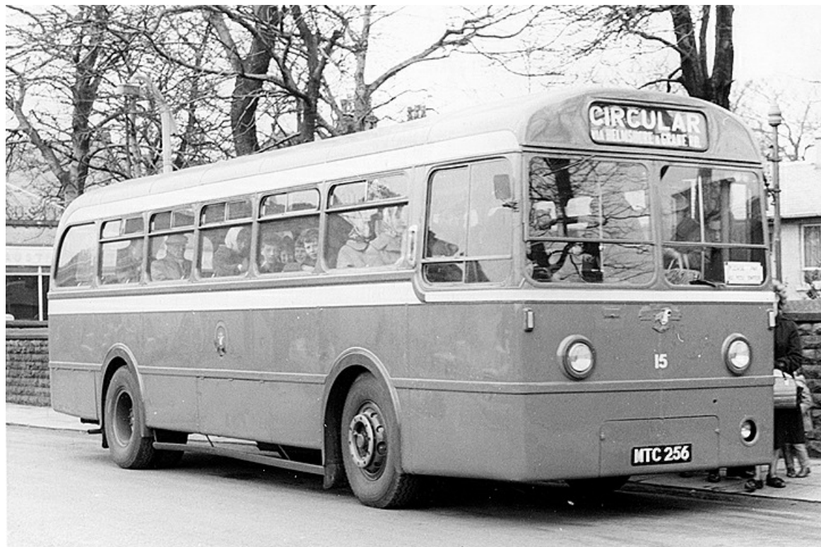
Haslingden No. 15 (MTC256) was one of two ex-Ramsbottom UDC vehicles purchased in 1962 and 1963. It was a Leyland PSU1/13 with Roe B44F bodywork, new in 1950. (LTHL collection).
