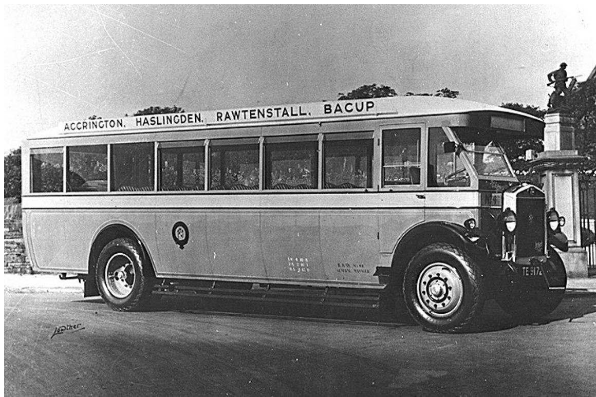
In 1929 Haslingden purchased this example of a Leyland Lion LT1 with Leyland 31-seat rear entrance bodywork. Numbered 4 (TE9172) it was withdrawn from service in 1936. (LTHL collection).
