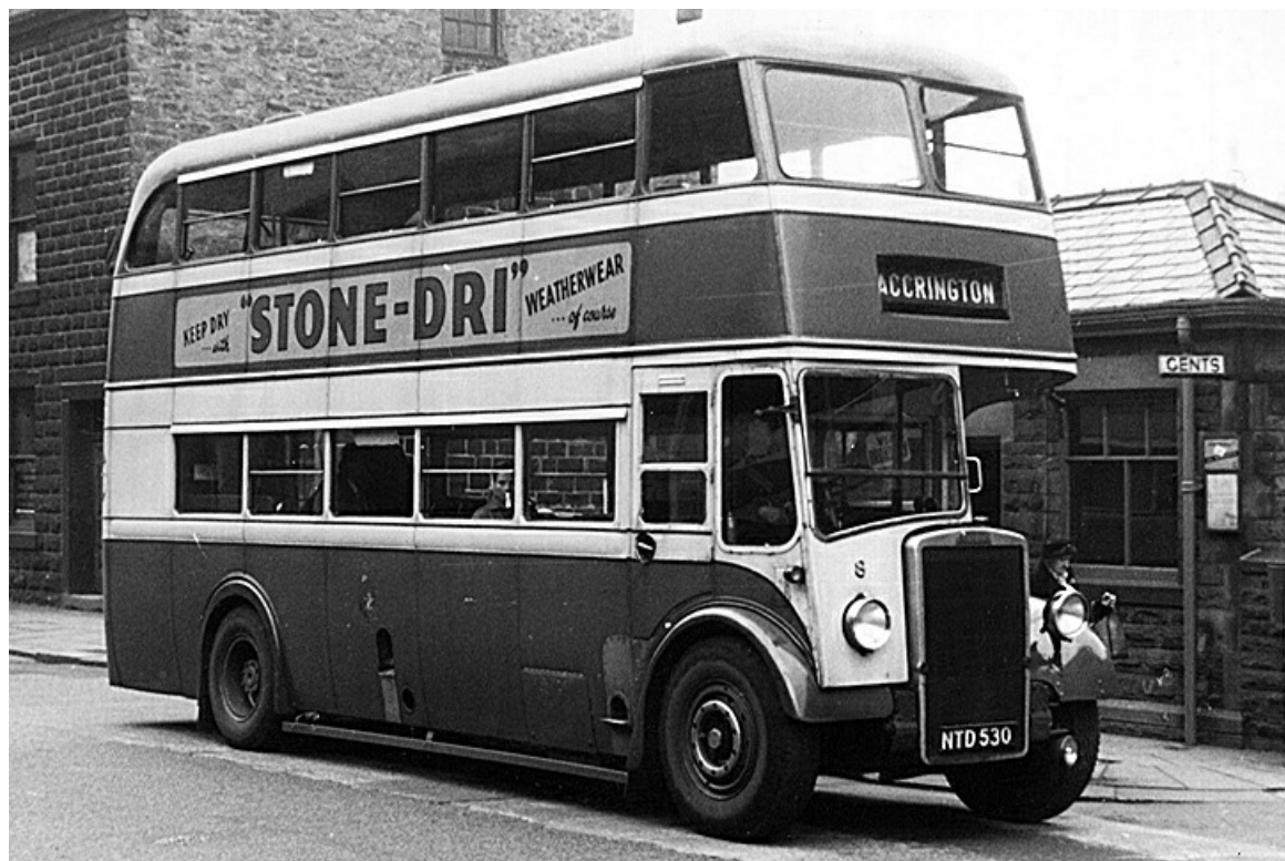
No. 8 (NTD530) an all-Leyland PD2/1 with H30/26R bodywork that joined the fleet in 1951. (LTHL collection).
