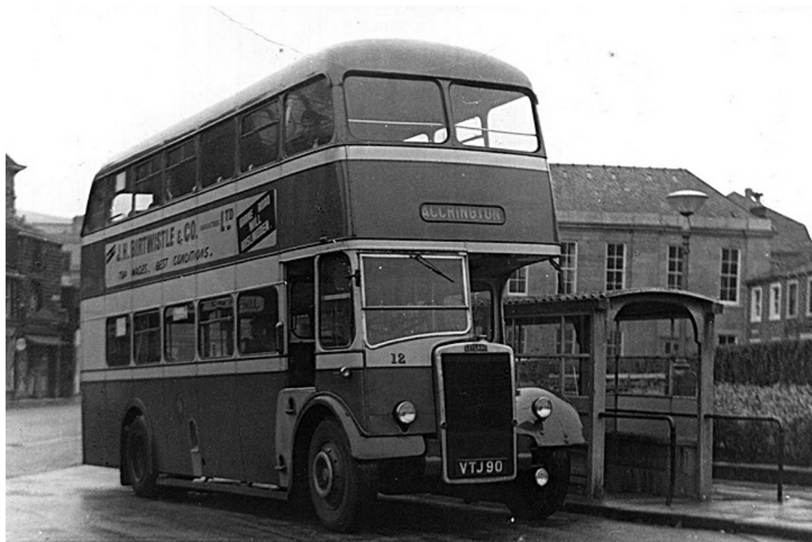
No. 12 (VTJ90) a 1955 Leyland PD2/12 with East Lancs H31/28R bodywork. It passed to Rossendale JTC in 1968 where it was re-numbered 42. (LTHL collection).
