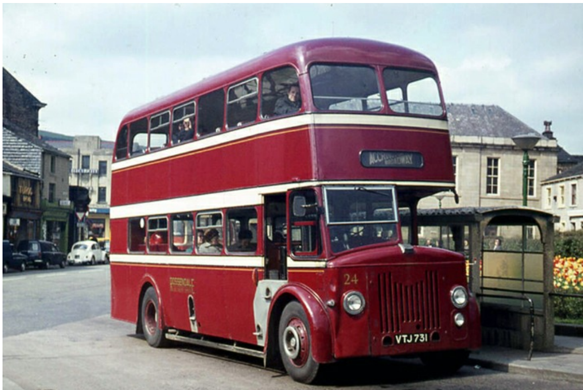
No. 24 (VTJ731) was a 1955 Leyland PD2/20 with an East Lancs 59-seat body. Originally numbered 60 it was re-numbered in 1964 and is seen here in Bacup in 1971 then part of the Rossendale Joint Transport fleet. (John Kaye).
