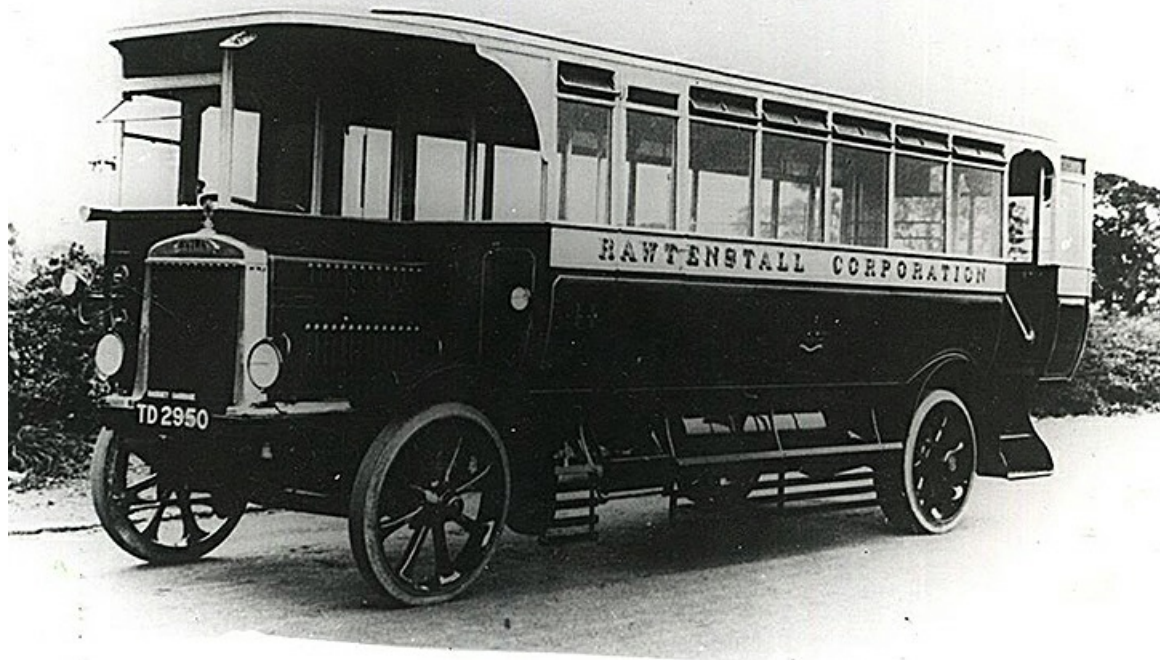
No. 41 (TD2950) was a 1925 Leyland SG11 with Leyland 36-seat dual-entrance bodywork. The forward entrance is barely visible in this photograph although the gap in the guard rail gives away the location. (LTHL collection).
