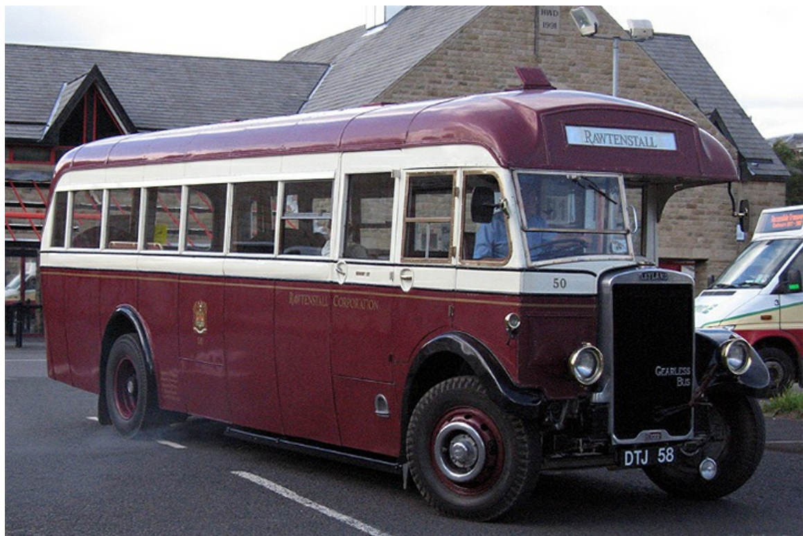
No. 50 (DTJ58) is a 1939 Leyland TS8c with Leyland 36-seat rear entrance body, now in preservation. (LTHL collection).
