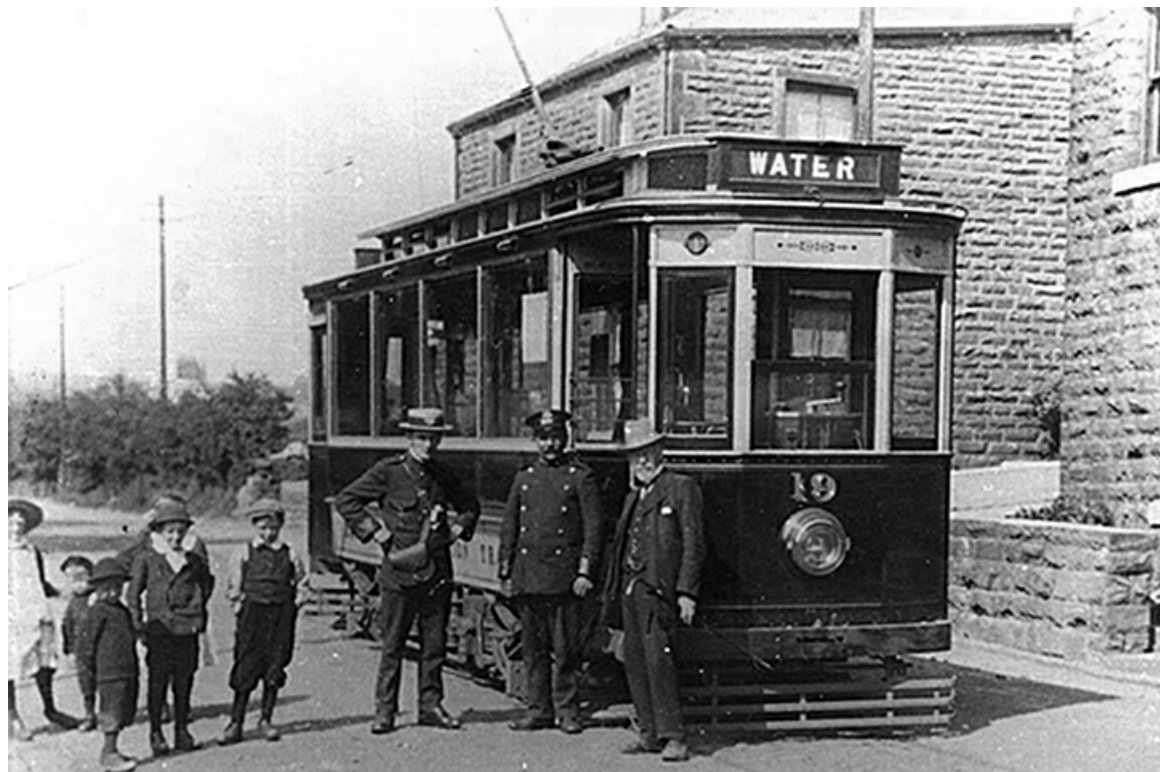
No. 19 was one of the 6 single-deck trams in the fleet - primarily for use on the Water route. It was built by the United Electric Car Company of Preston and seated 30. (LTHL collection).
