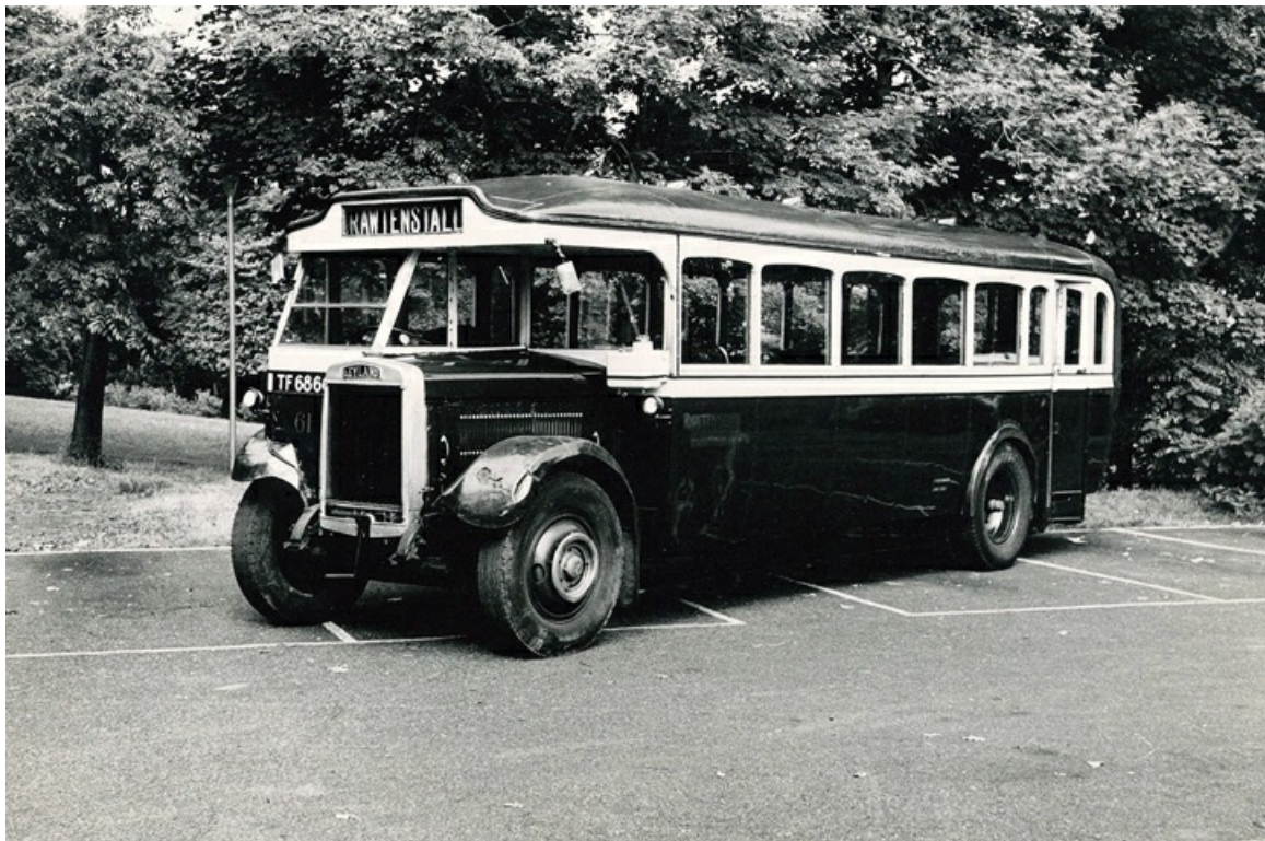
No. 61 (TF6860), a 1931 Leyland LT3 with Leyland B36R bodywork. It was withdrawn in 1947 and subsequently used as a snowplough. (LTHL collection).
