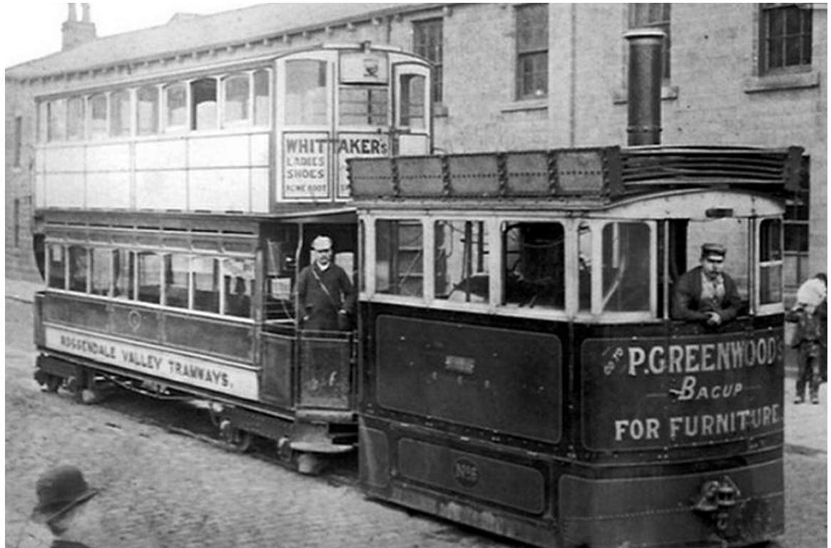
Thomas Green loco No. 6 of the Rossendale Valley Tramways Company towing a Milnes trailer car. The company was acquired by Rawtenstall Corporation in 1908 who continued to operate the tramway until electrification of the system the following year. (LTHL collection).
