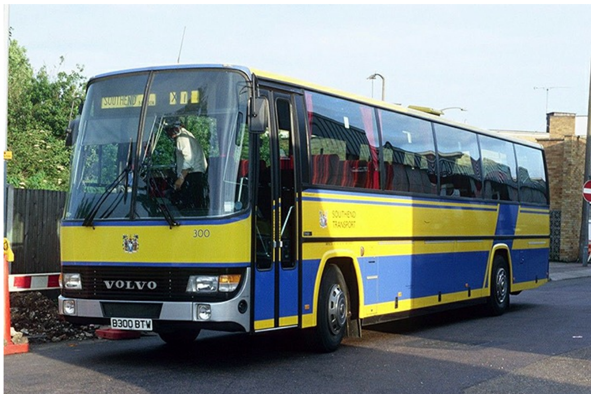
No. 300 (B300BTW), a Volvo B10M-61 with Berkhof 53-seat coachwork that was in the fleet for just under 12 months in 1985. (LTHL collection).
