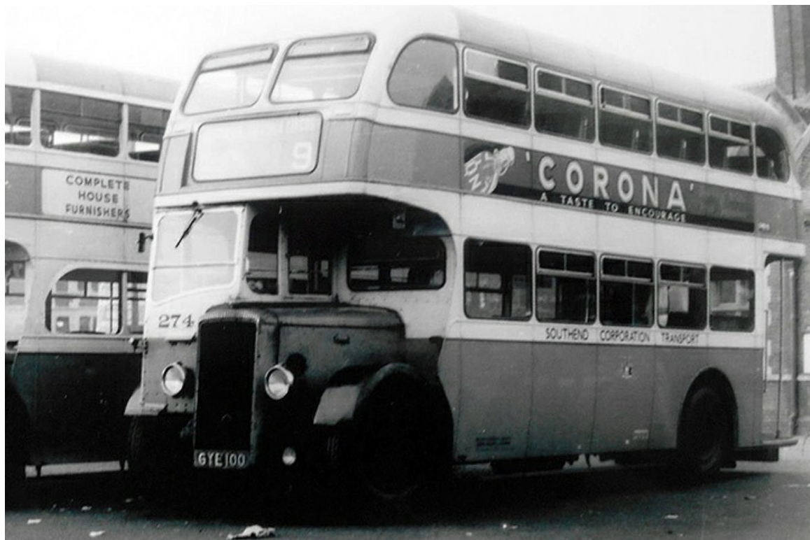
1945 Daimler CWA6 No. 274 (GYE100) came via London Transport in 1954. It was re-bodied by Massey with this 55-seat body before entering service. (LTHL collection).
