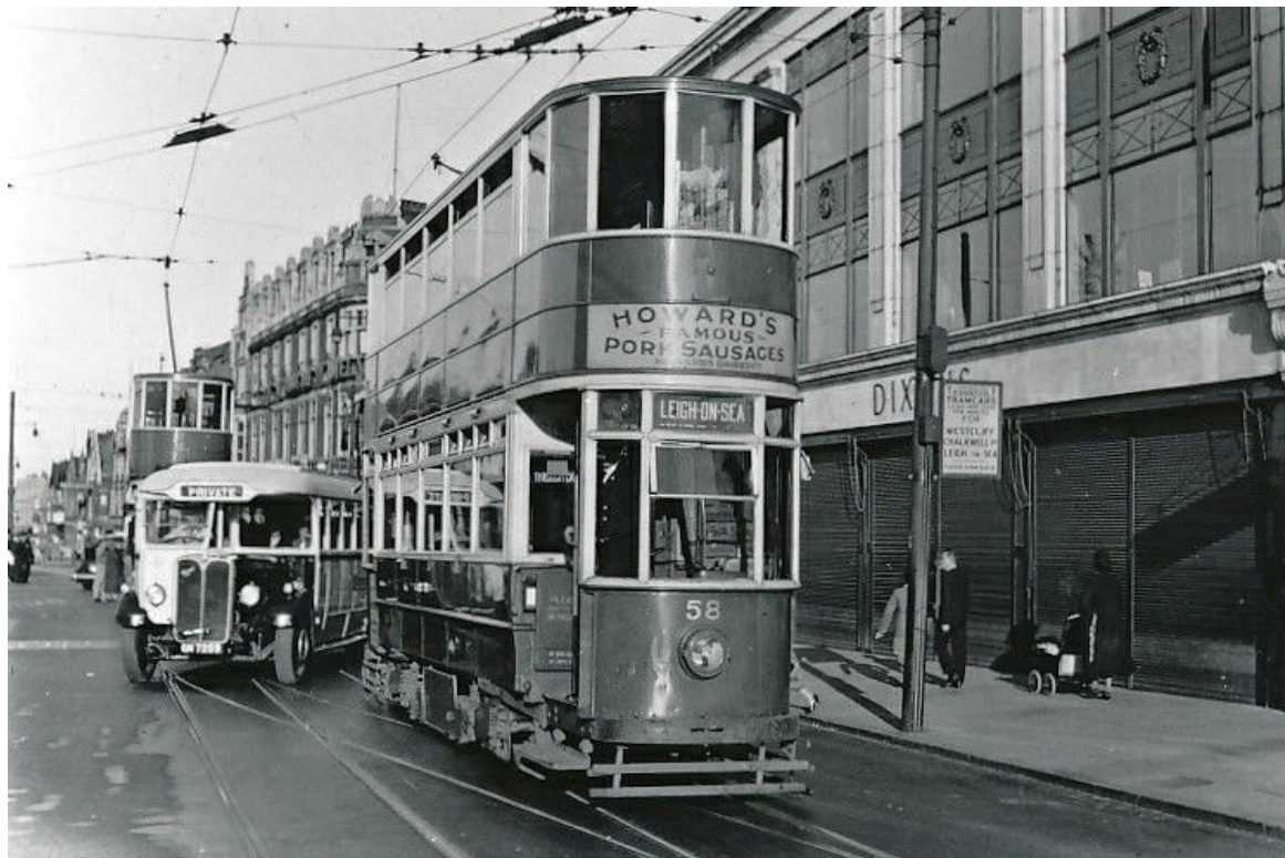
No. 58 was an English Electric fully-enclosed car on English Electric trucks, dating from 1924 and seating 70. (LTHL collection).
