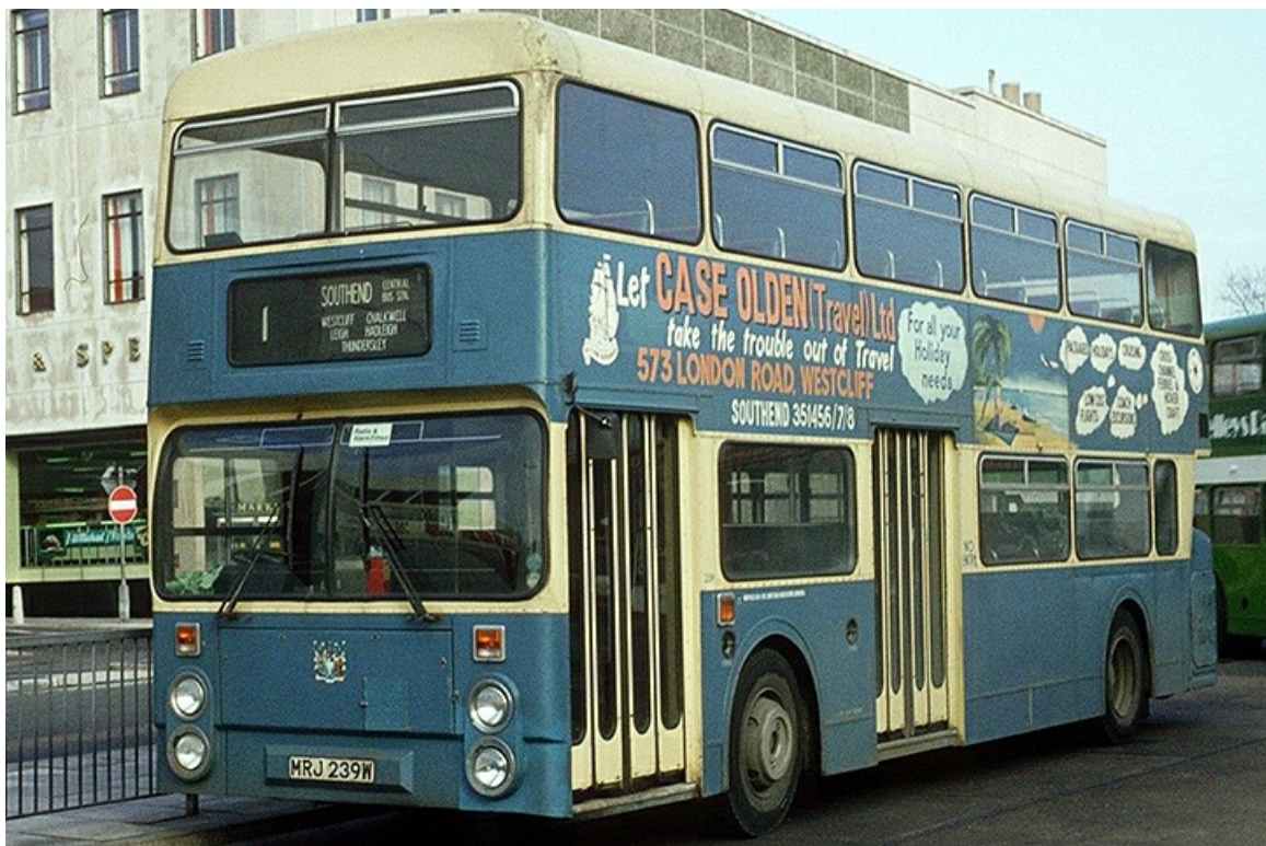
No. 239 (MRJ239W) was a 1981 Leyland Fleetline FE33ALR with Northern Counties 80-seat bodywork. (LTHL collection).
