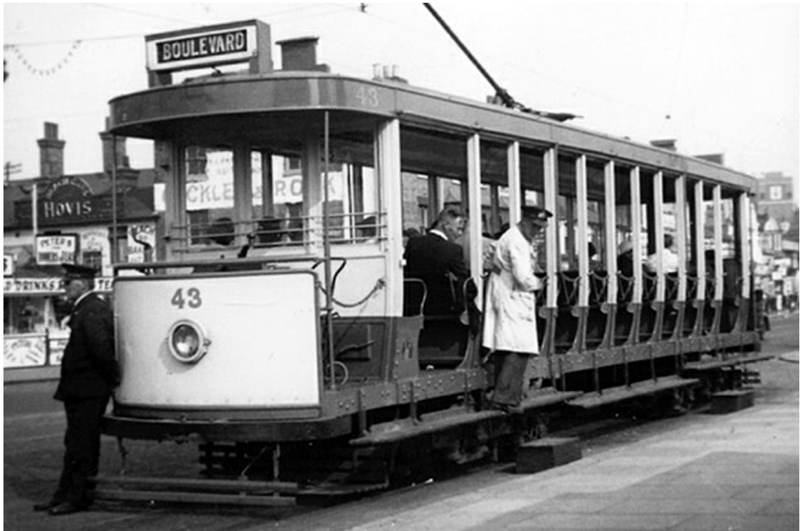
In 1921, to cater for the influx of visitors, Brush supplied this roofed toastrack (No. 43) seating 49. (LTHL collection).
