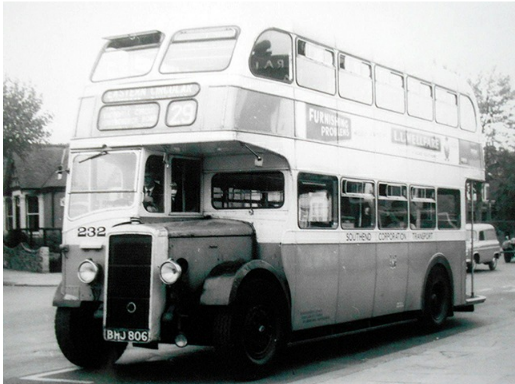
1945 Daimler CWA6 No. 232 (BHX806) with Massey 57-seat bodywork that replaced the utility Duple bodywork in 1952. (LTHL collection).
