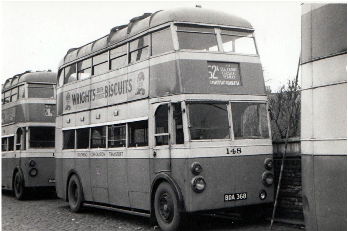
Sunbeam MF2 No. 148 (BDA368) with Park Royal 54-seat bodywork dating from 1937 was a second-hand purchase from Wolverhampton Corporation that joined the fleet in 1950. (LTHL collection).
