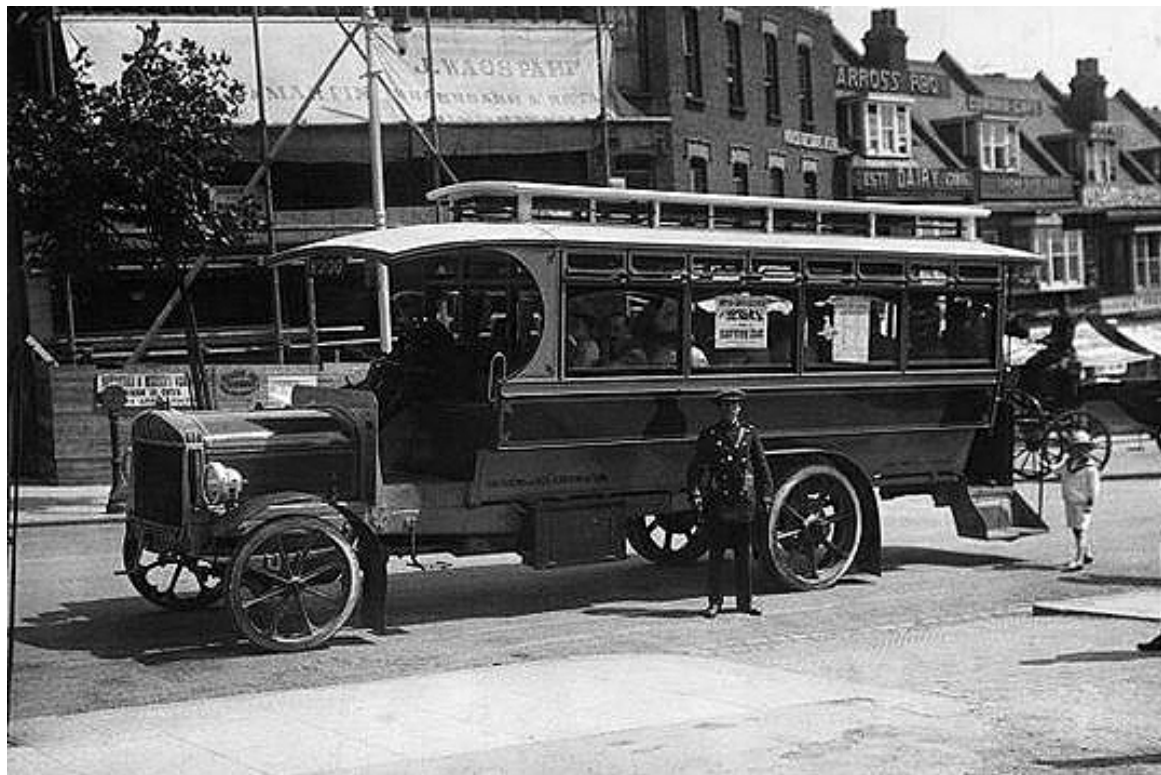
Southend No. 3 (HJ30), a 1914 Tilling-Stevens with Brush 22-seat bodywork. (Getty Images/Hulton Archive).
