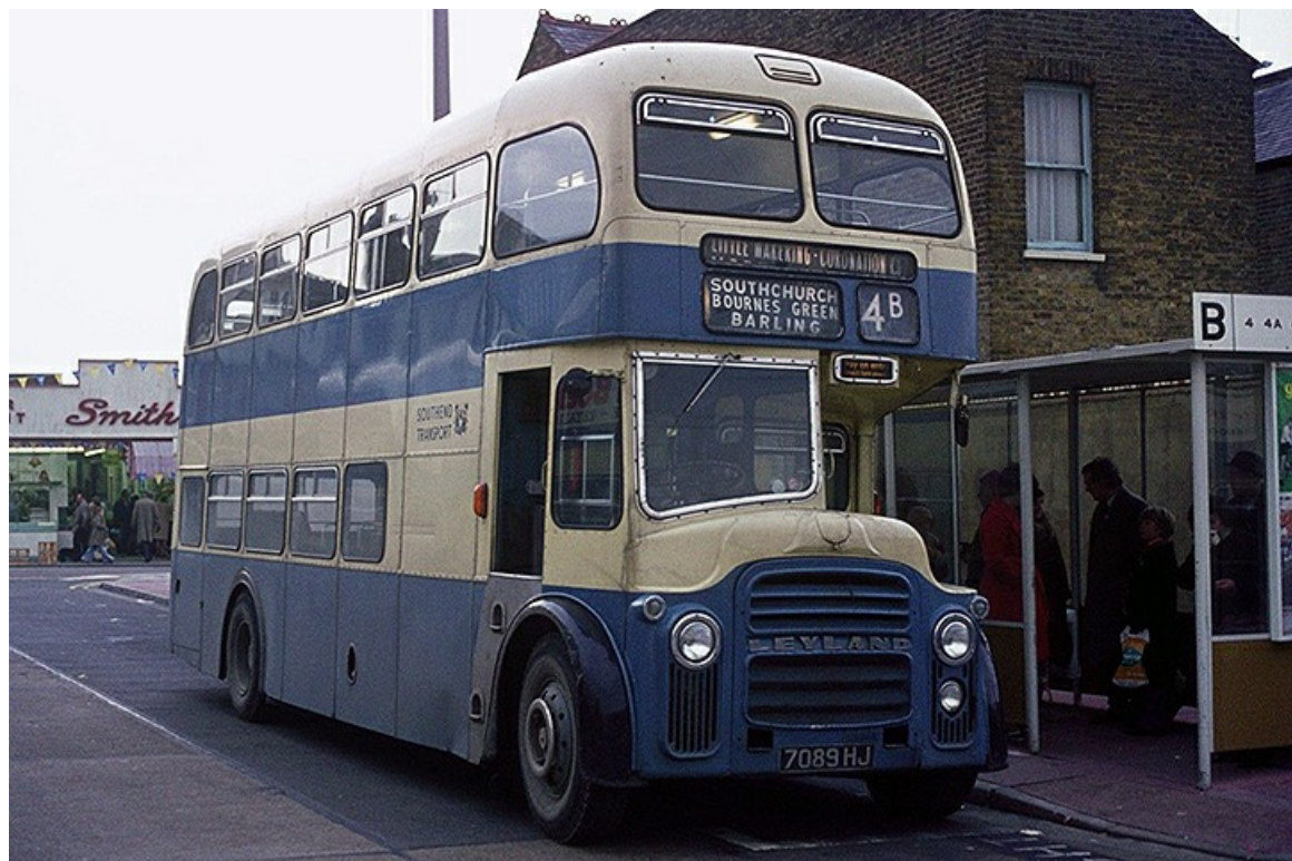
No. 325 (7089HJ) was a 1963 Albion Lowlander LR7 with Alexander 70-seat bodywork. (LTHL collection).
