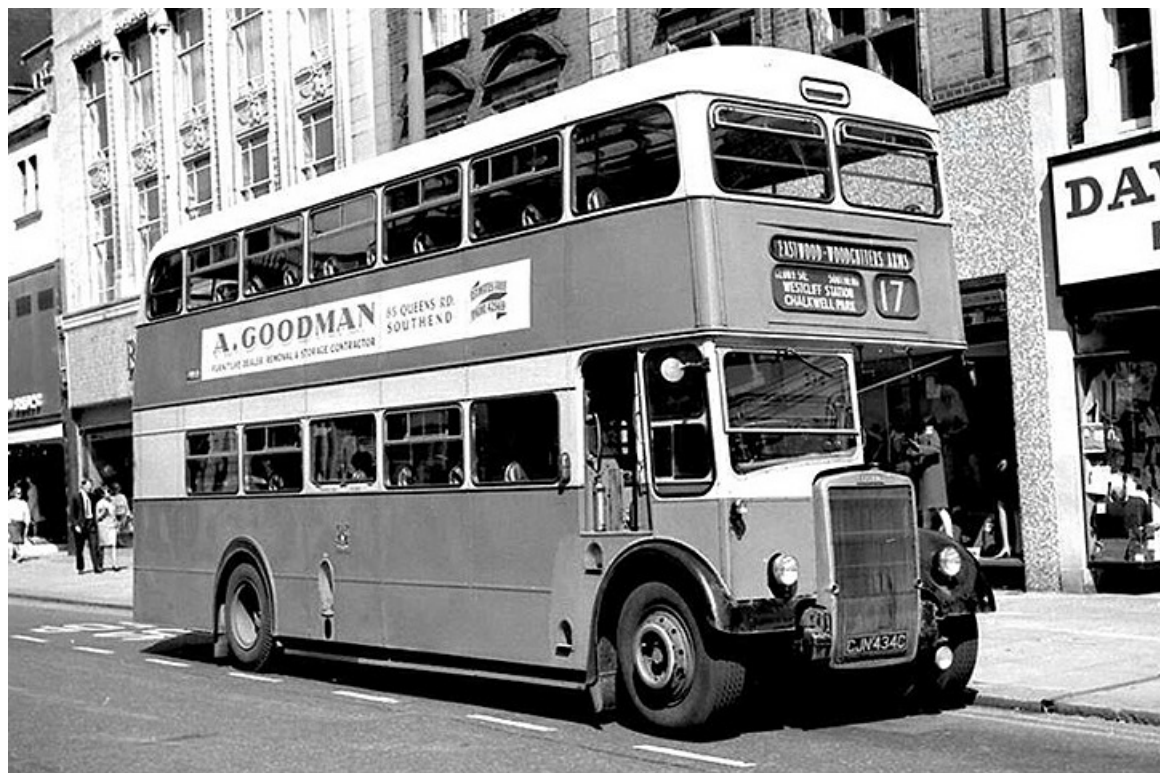
No. 334 (CJN434C) was a 1965 Leyland PD3/6 with Massey 70-seat bodywork, seen here in High Street in 1967. (John Boyllett courtesy John Kaye).
